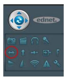
Starting the automatic, horizontal movement of the camera (to the right/to the left). Press again to end movement.
