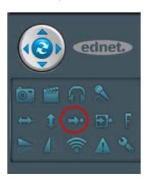
With this function, you can steer the camera to a pre-determined point. 8 different points can be stored.
