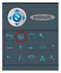
A single press on "video record" starts the camera recording; pressing again will stop recording. The recorded videos are stored in the file indicated by you and can then be retrieved by means of the "search" function. (See "13.6 Search" on page 28)
