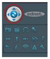
In addition, the movement control area serves to drive the camera automatically or manually. The middle area moves the camera automatically into all directions, with the respective arrows in the outer area the camera can be steered manually.
