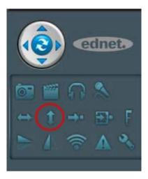
Swings the camera vertically (up/down). Press again to end movement.
