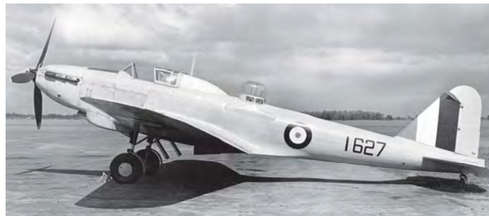
ABOVE: RCAF 1627 shows a Canadian turret modification to the Battle for gunnery training purposes. This created the MkII. VIA LARRY MILBERRY
