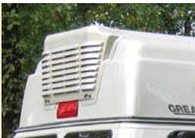
The built-in roof air conditioner provides a cleaner exterior look, more interior headroom in the rear of the coach and features a built-in heat pump
