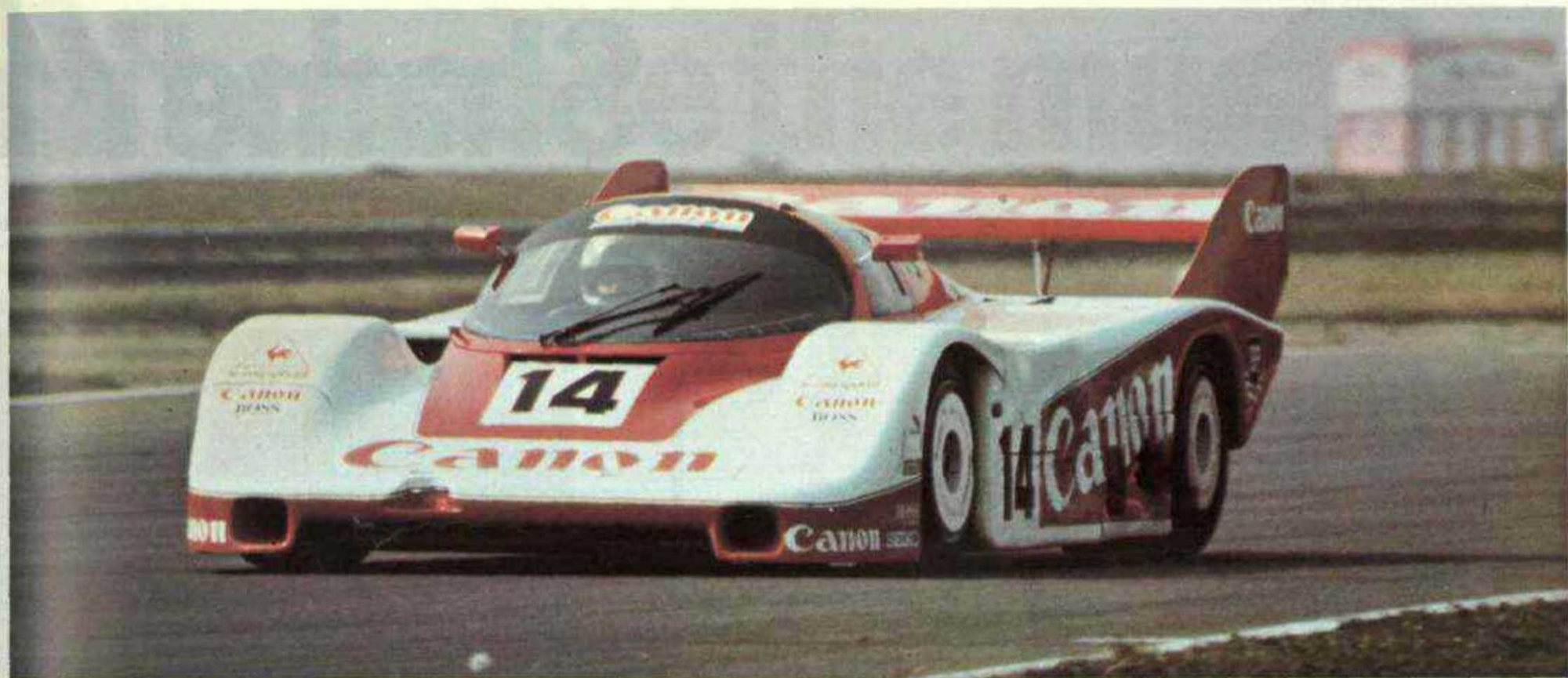
A TERMINAL speed of over 160 mph on the Club Straight at Silverstone was reached just after shifting briefly into fifth gear. Yet, braking at the 300 metre board, the 956 lost speed so rapidly that it could have been stopped before the apex of Woodcote Corner.
