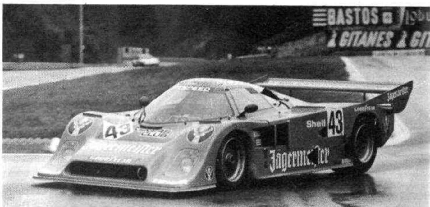
A WELCOME addition to the Spa grid was the Zakspeed Ford C1/4, powered by a turbocharged 1.7 litre engine. Inspired by the C100, the C1/4 ran well in the early stages, to retire with a broken gearbox.
