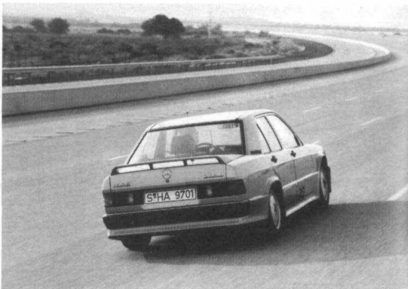
WITH the 16-valve Cosworth cylinder head the Mercedes 190E 2.3-16, to give the car its full title, develops 185 bhp. At Nardo, the new car covered 50,000 kms in under 202 hours at an average speed of 247 kph.
