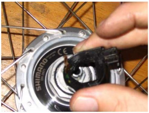
If this is the first time your hub has been opened, there will be a mess of white, semi-solid substance (which I assume is Teflon) slathered around the wire where it passes through an opening in the silver metal spacer at the triangular end. You'll probably need to pick away some of the Teflon to remove the spacers. Below the spacers, the wire runs in the groove on the hub axle. After you've removed the spacers (parts 4 and 5), the hub will look like this:
