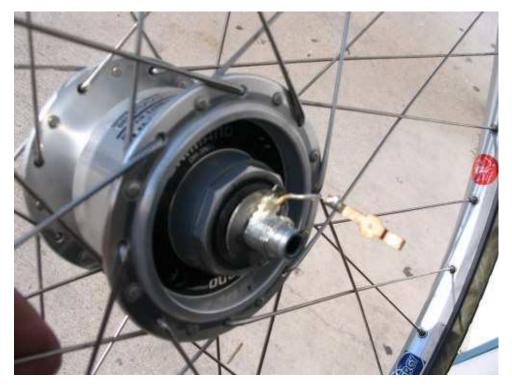
Place the wire along the groove in the hub so that the back plate (part 3) can be removed and the cone screwed off the axle without damaging the wire.
