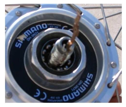
Break the lock nut from the cone on the non drive side of the hub and remove both. Then using a 32mm wrench grab the large nut on the drive side of the hub pictured below and turn counterclockwise. This will take a little force, brace the wheel against your body for a good grip.
