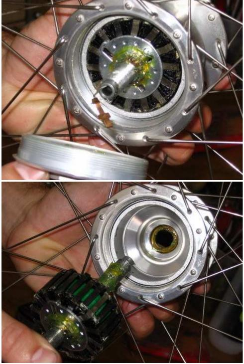
With the axle out of the way, the bearings on each side of the hub can easily be removed and the cups cleaned and inspected. Remove all the old grease and repack, replacing bearings as necessary.
