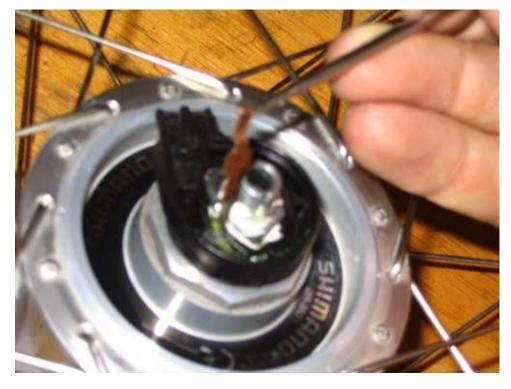
You'll notice an opening on the bottom of the plug assembly body. This opening is large enough for the current connector to pass though. Carefully work the plug assembly body off the hub.
