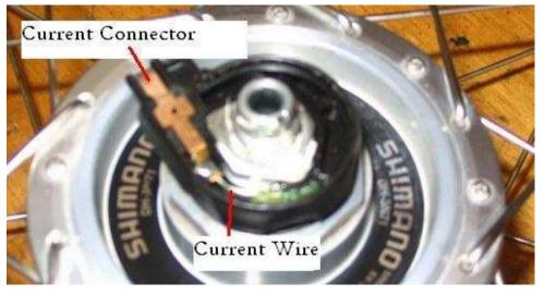
Use your sharp tool to lift up the current connector and wire. Be careful not to stress the soldered connection between the two.
