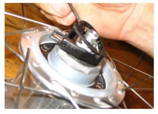
Now the current connector and current wire are exposed. Sorry for some of the blurry pictures below.  $% \left( {{{\left[ {{{\left[ {{\left[ {{\left[ {{{\left[ {{{c_{1}}}} \right]}}} \right]}} \right.}} \right]}} \right]} \right]$
