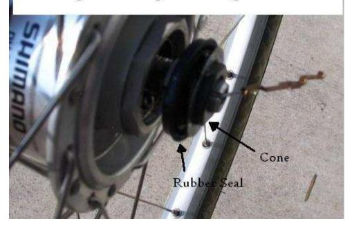
At this point the ball bearings on the drive side are exposed, but they're not easily accessible and you'll find it hard to clean the cups of the hub well unless we remove the axle.
