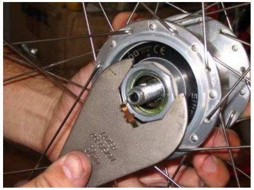
Now the inner assembly of the dynamo can can be removed.
