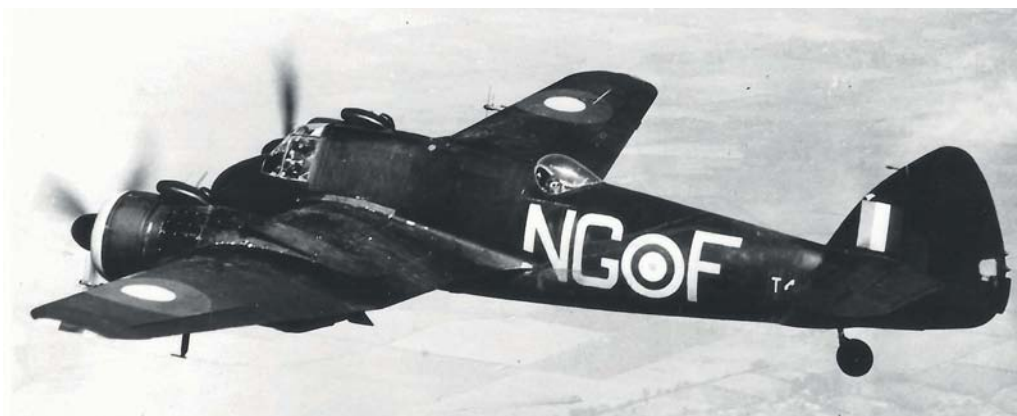
Below: Nose and wing-mounted radar aerials are evident on this 604 Squadron Mk.II in the spring of 1941. VIA R C B ASHWORTH
