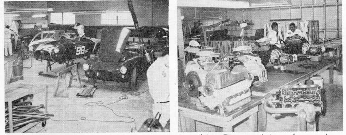
PRODUCTION LINE (left) of the A.C.-Cobra shows two cars nearing completion. The present production rate of one car per day is to be increased. RIGHT: Engines for the Cobra. In standard form the 4,261 c.c. V8 Ford engine develops 260 b.h.p. at 5,800 r.p.m.
