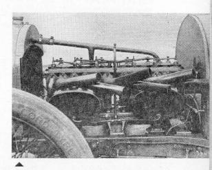
SIDE VALVES were used on the Belgian Excelsior, one of the very few Edwardian six-cylinder racing engines.
