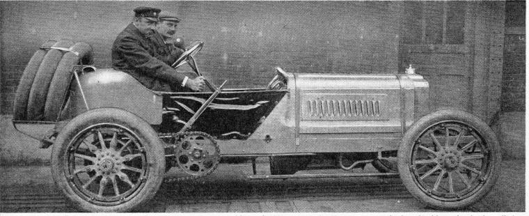
OVER SQUARE. The very successful Richard Brasier had a side valve four-cylinder engine of 165 mm.  $\times$  140 mm.
