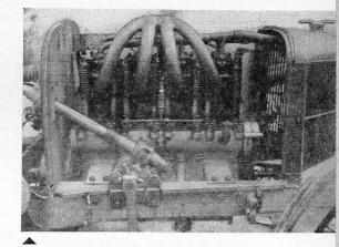
MEDIUM STROKE. The four-cylinder 85 mm.×132 mm. 3-litre Alcyon engine of 1912. The four radial valves per cylinder had the valve springs located on the pull-rods. Note the induction manifolds.
