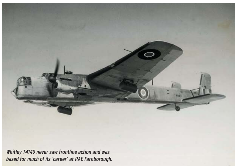
A view of T4149 clearly showing its underwing rocket canisters.
