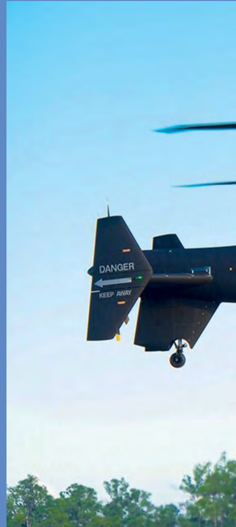
Below: The V-280 is a third-generation tiltrotor, which follows a remarkably different design compared with other aircraft in its class, such as the Osprey. It uses a V-tail, smaller wings and a sleeker, compound fuselage. It is also smaller than the V-22. Bell
