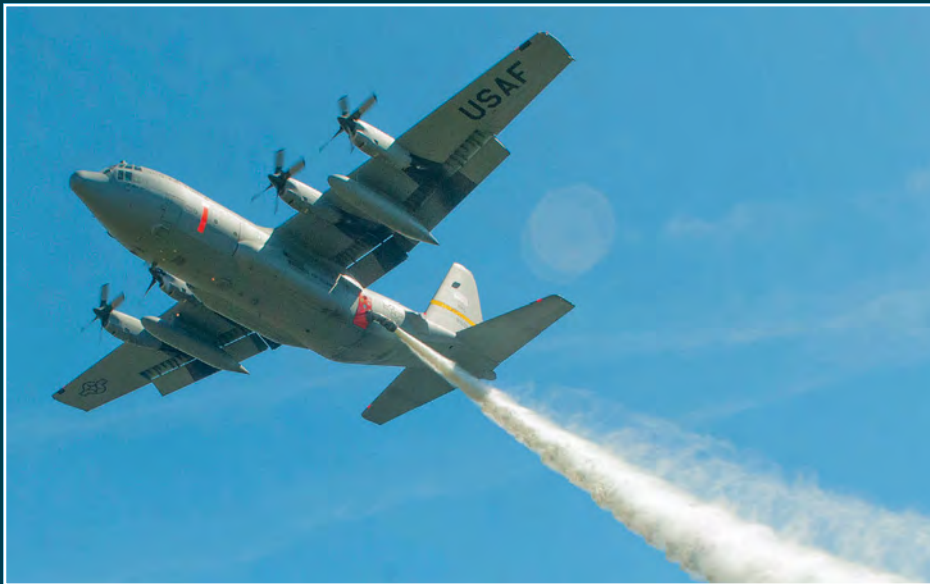
Each year the four MAFFS units undertake qualification and certification together. Here a C-130H from the Wyoming ANG's 153rd AW discharges its load during 2016 drop training. USAF ANG/Tech Sgt Emerson Marcus
