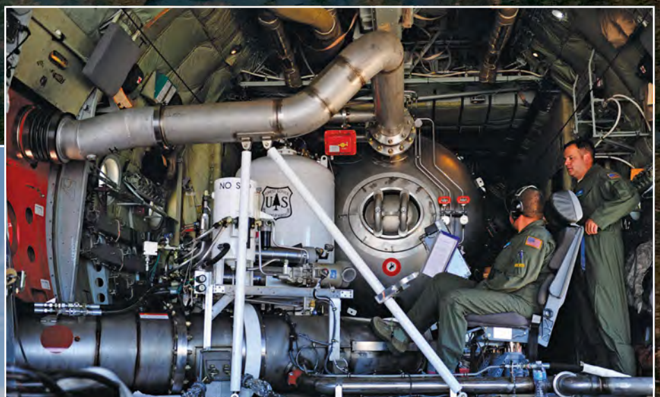
Above: The palletised MAFFS II unit is installed in under two hours and is manned by a Crew Chief in the rear of the aircraft. USAF/SSgt Stephany Richards
