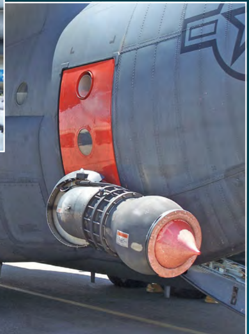
Below: The pintale nozzle can be used at various settings for different retardant dispersal patterns and rates. US Forest Service/Richard Stowers
