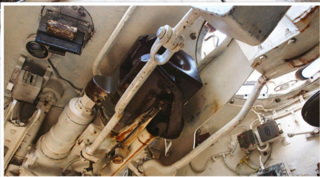
Below: The cramped interior of the conventional Sherman tank was made even tighter with the addition of the Firefly's heavy 17-pounder
