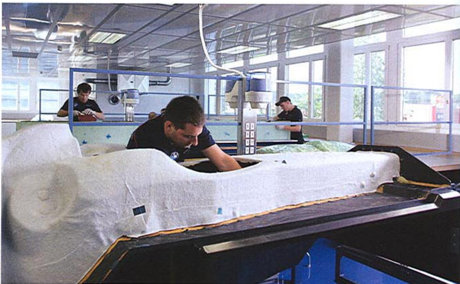
A monocoque 'upper' section is prepared for curing in the autoclave. The roll-hoop (inside the air-intake) is bonded later
