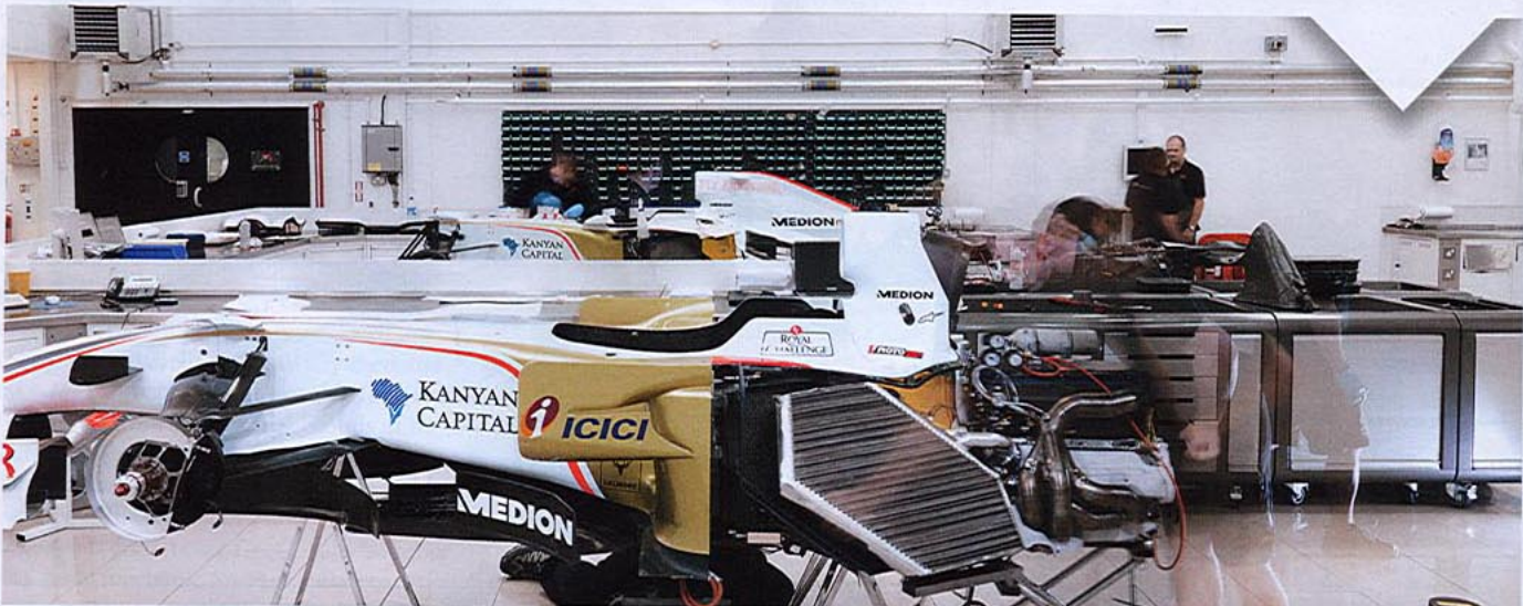
Day two - the Ferrari engine and its plumbing are in place, then the gearbox goes on
