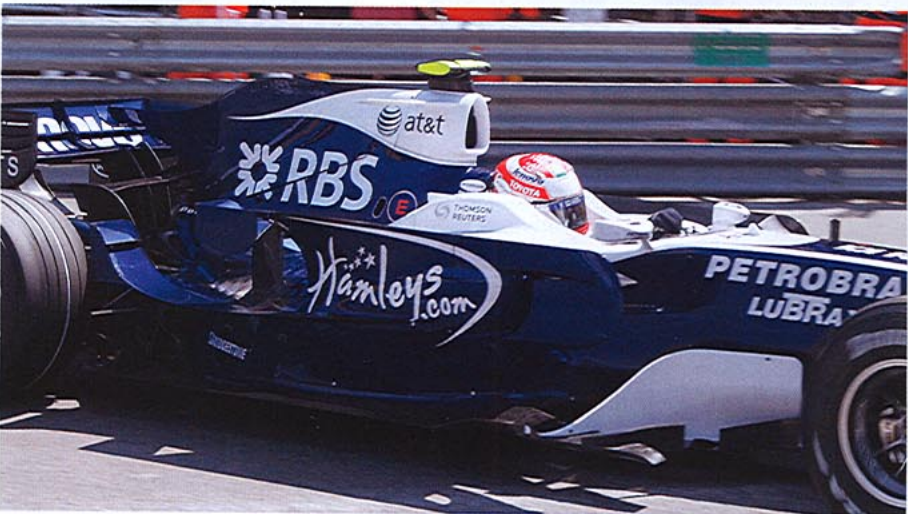
Red Bull were the first to develop the anvil wing; Williams introduced their version for this year's Monaco GP
