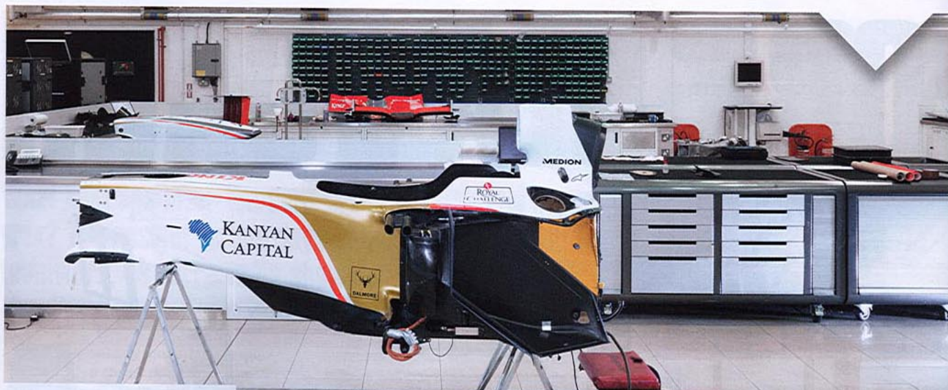
The 'tub' doesn't change much during the first day, as checks are made and small parts fitted
