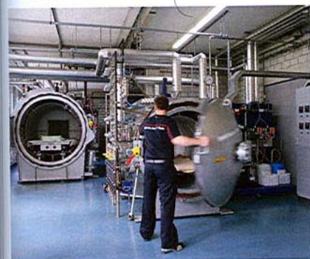
The cars' carbon fibre parts are 'baked' in these autoclaves
