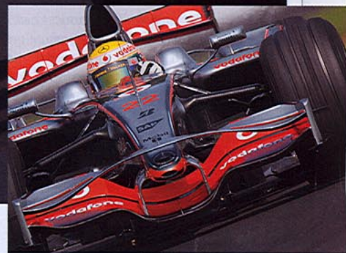
Bridge wings let other aero devices toward the back of the car work more efficiently
