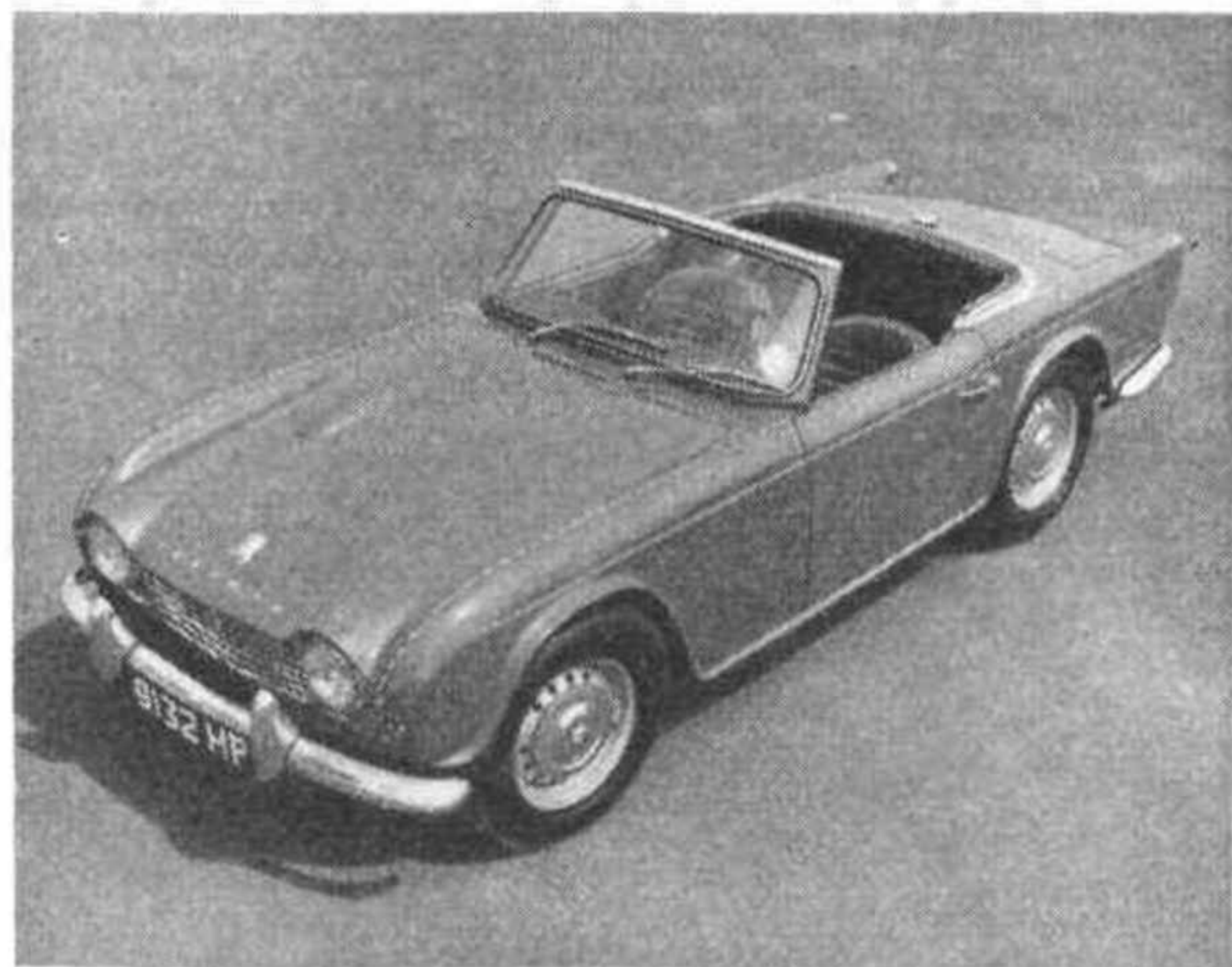
New lines, a larger engine and rack-and-pinion steering are features of the new 100 b.h.p. Triumph TR4.
