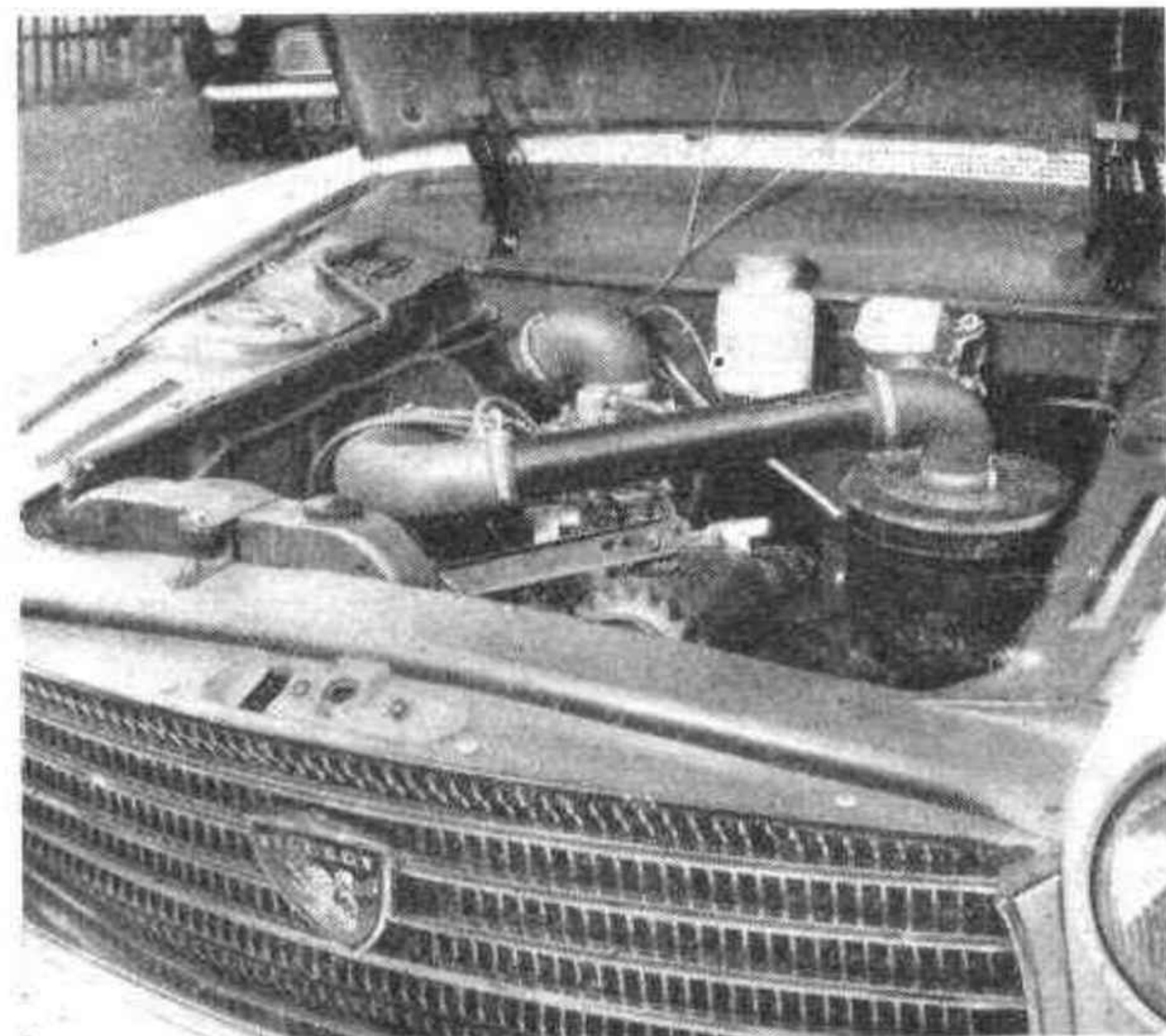
A low bonnet line is ensured by inclining the engine of the Peugeot 404 at 45° to the off side. This power unit retains the classic push-rod valve gear, with segmental hemispherical combustion chambers in an Alpac head.
