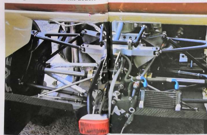
Looking down onto the Arrows A8. Note the placing of the long radiators in fan-like position following the trend in F1. Nothing unusual about the double wishbones with their push rods and mini rocker. The ergonomics of the cockpit have been carefully designed.
