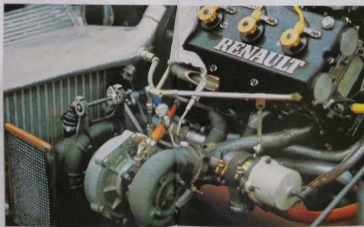
The Renault V6 is compact, slim and contrasts sharply with the bulky nature of the turbos and intercoolers.
