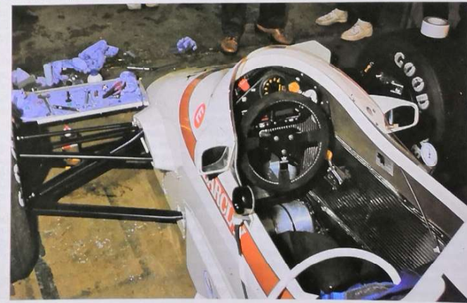
Looking down onto the Arrows A8. Note the placing of the long radiators in fan-like position following the trend in F1. Nothing unusual about the double wishbones with their push rods and mini rocker. The ergonomics of the cockpit have been carefully designed.
