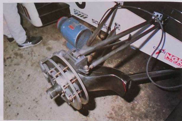
An original piece of work. Two carbon discs on the Williams' front wheel!
