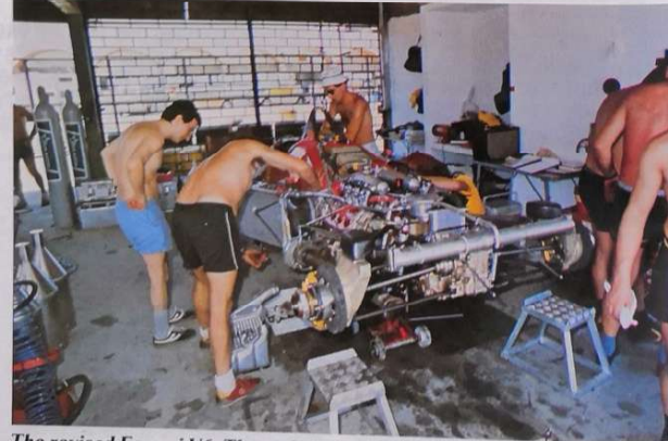
The revised Ferrari V6. The turbos have been repositioned on either side of the engine.
