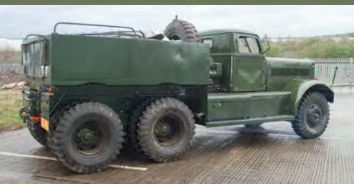
ABOVE: Nigel's Diamond T 980 with eight-ton ballast body RIGHT: 980s served into the early 1970s in British use BELOW: The ballast body was found in a field in Norfolk. It could be loaded with sand or gravel or cast concrete blocks for maximum weight
