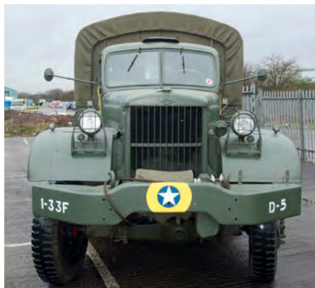
ABOVE & BELOW: With a load capacity of four tons, the 968/968A saw service in all theatres during World War Two. A soft-top version was used in warmer regions LEFT: The small cab is lifted straight from a pre-war Diamond T light commercial. The long mirror arms make for excellent all round visibility
