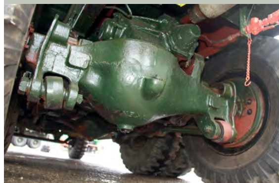
The rear axles are Timken double reduction units giving low speed but enormous power
