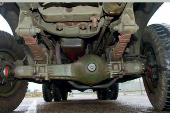
Timken F-2090-W-73 double reduction front axle. In normal use the vehicle operates as a 6x4, but 6x6 is selectable when needed
