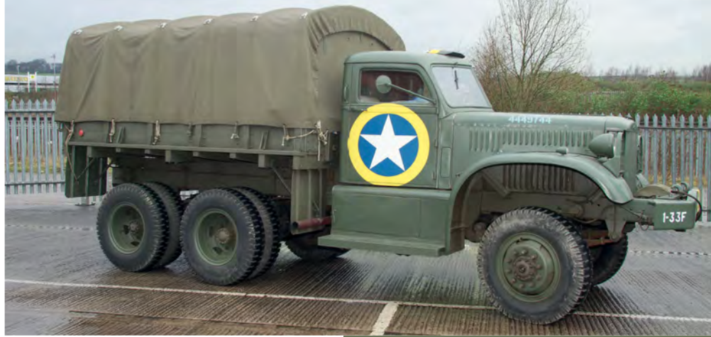
ABOVE & BELOW: With a load capacity of four tons, the 968/968A saw service in all theatres during World War Two. A soft-top version was used in warmer regions LEFT: The small cab is lifted straight from a pre-war Diamond T light commercial. The long mirror arms make for excellent all round visibility
