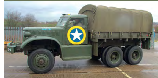
ABOVE & BELOW: With a load capacity of four tons, the 968/968A saw service in all theatres during World War Two. A soft-top version was used in warmer regions LEFT: The small cab is lifted straight from a pre-war Diamond T light commercial. The long mirror arms make for excellent all round visibility
