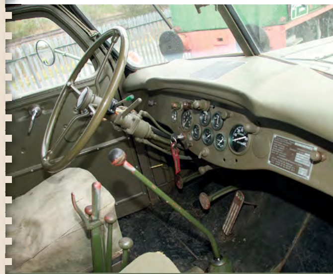
ABOVE: The inside of the cab is well laid out, and all controls fall readily to hand. The massive wheel compensates for the lack of power steering ABOVE MIDDLE: The twin Timken SFD-154-W rear axles are suspended on leaf springs with supporting struts, and offer impressive articulation
