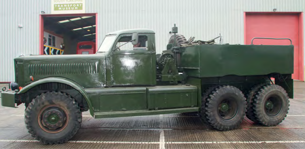
ABOVE: Nigel's Diamond T 980 with eight-ton ballast body RIGHT: 980s served into the early 1970s in British use BELOW: The ballast body was found in a field in Norfolk. It could be loaded with sand or gravel or cast concrete blocks for maximum weight
