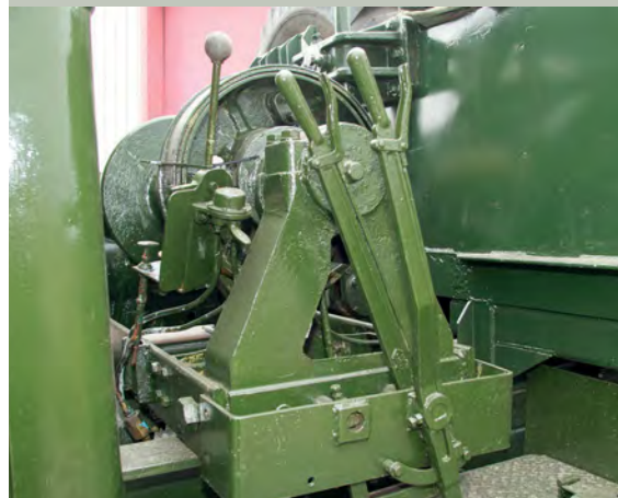
The Garwood winch is operated from the power take off, and has a 40000 lb capacity
