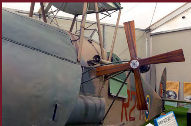
Above The fuselage of LF789 at the de Havilland Aircraft Museum showing the substantial windmill that powered the air compressor.
