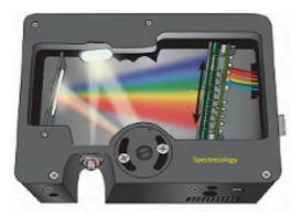
1c Full-width at half-maximum (FWHM) values are motivated at many typical wavelengths and are listed in the shape, suggesting a wavelength quality of about 5 nm. The spectrometer can be used within a wavelength range covering the visible and the near infrared area (~400 nm-1000 nm, limited by the level of sensitivity of the CMOS detector).
