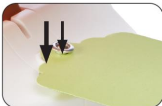
1. Assemble eyelet by placing tag hole on post with eyelet on top.
