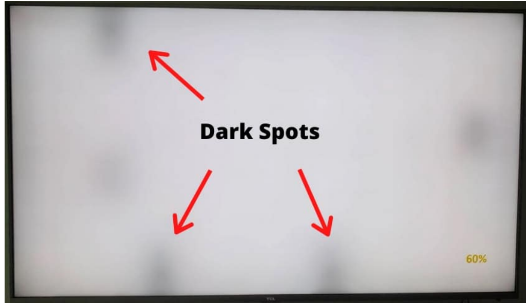
Fig 74. Heat Damage on LCD Displays
