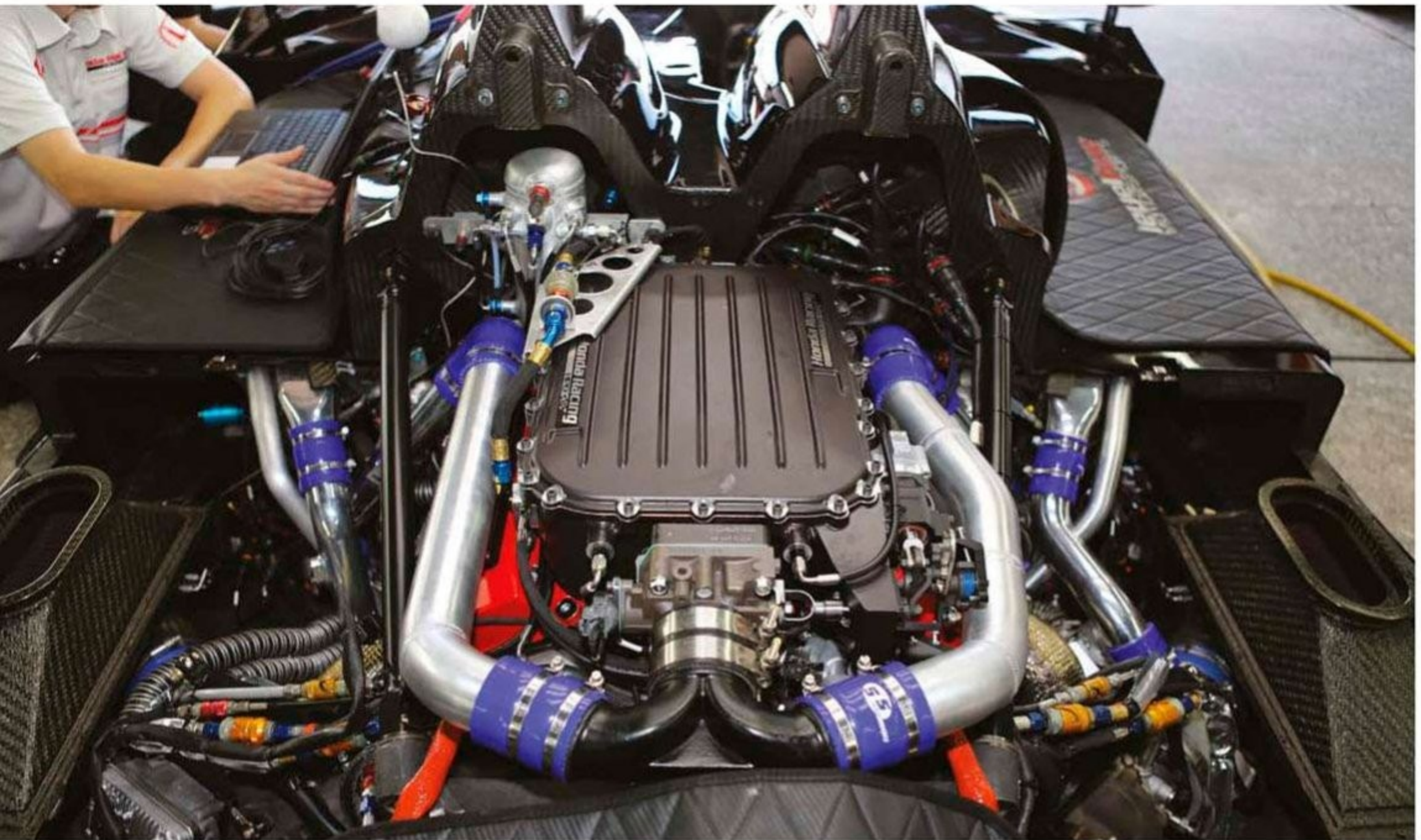
Dimensionally, the direct injection version of the P2 engine has been tailored to bolt into the HPD ARX-03b chassis with minimal modifications required
