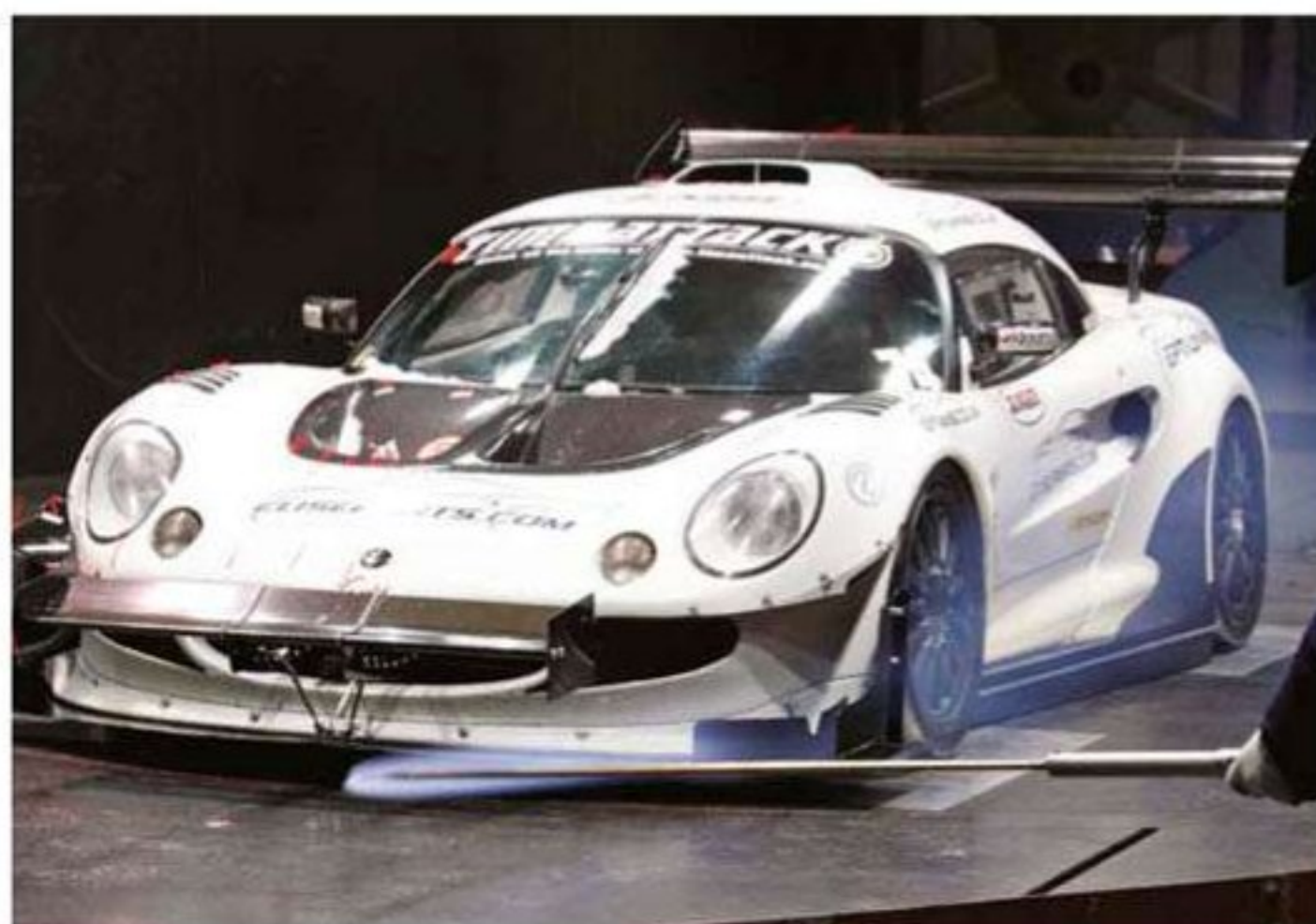
The Jamie Willson Lotus Exige Time Attack car featured splitter end fences that partially constrained the airflow
