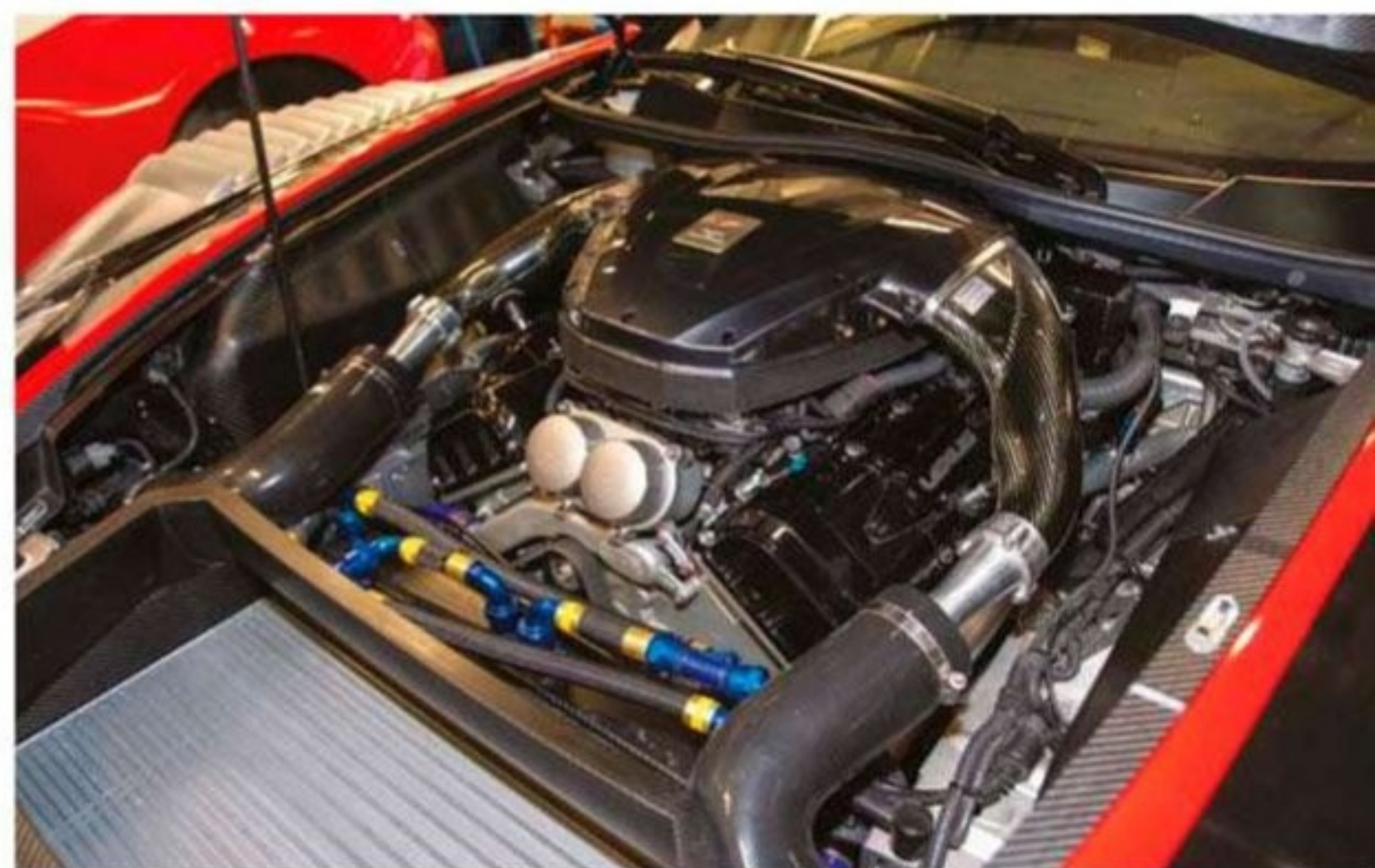
The engine in the new LFA is based on the production supercar, retaining the 4.8-litre V10 layout. Maximum power is 367kW, produced at 8000rpm
