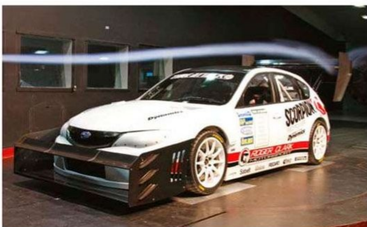
... but the wing's own induced downwash also turned the upstream flow downwards, as shown by the smoke plume outboard of the car's body
