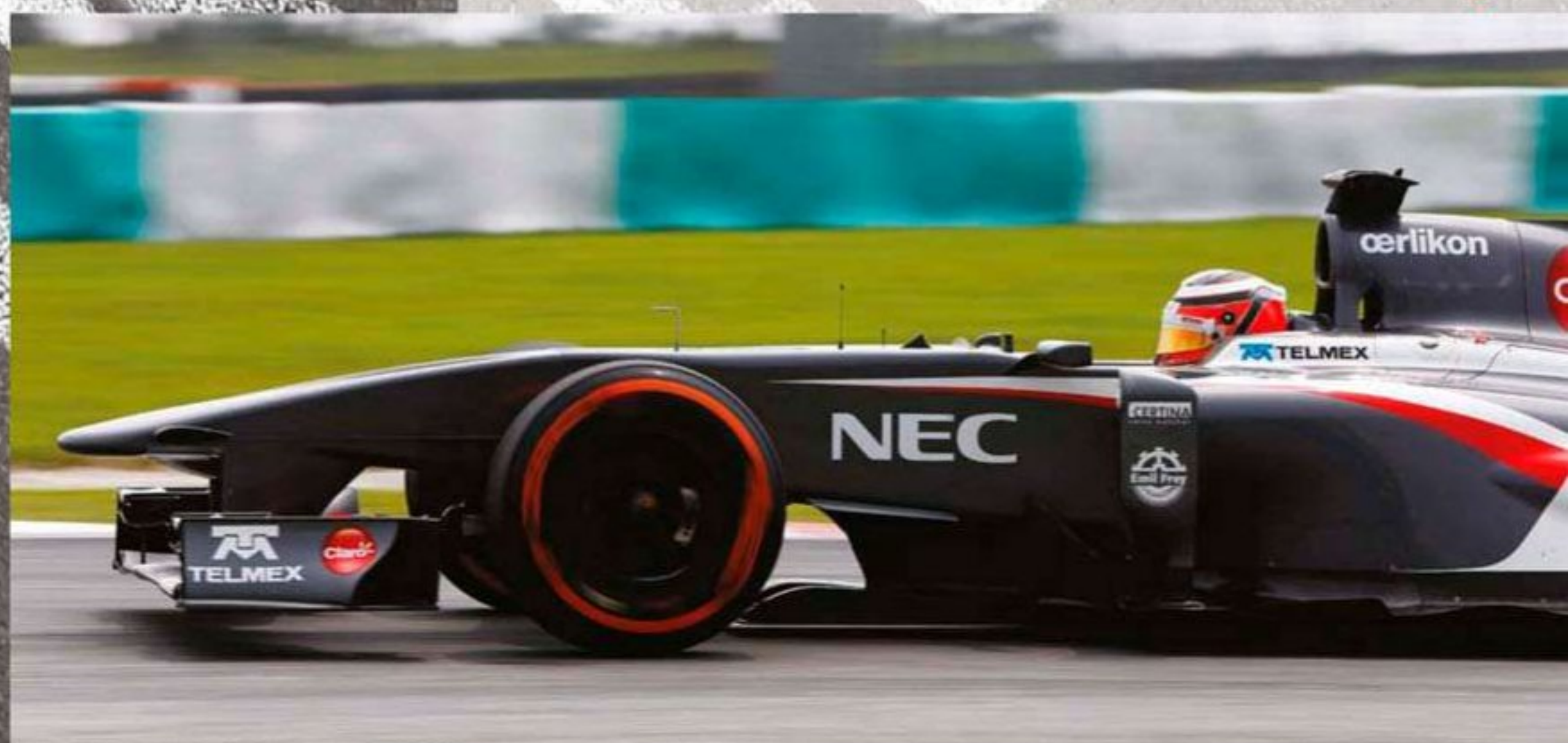
Sauber has smoothed out the nose of the C32 with a vanity panel but it is the view from above that shows the distinctive H-shape
