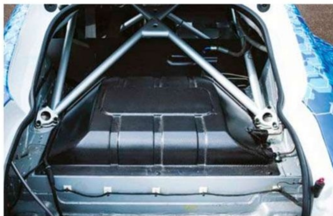
The hydrogen system adds around 100kg to the weight of the Rapide S, around 70 per cent of which is added by the fuel tanks and plumbing
