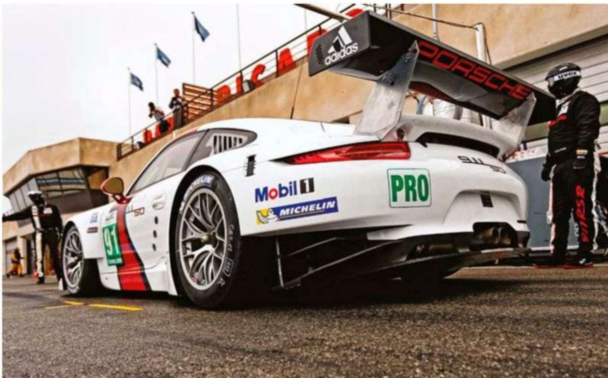
Strakes behind the rear wheel are not significant, says Porsche's motorsport director Hartmut Kristen. They just look good. The roofline and rear deck are slightly higher than on the 997
