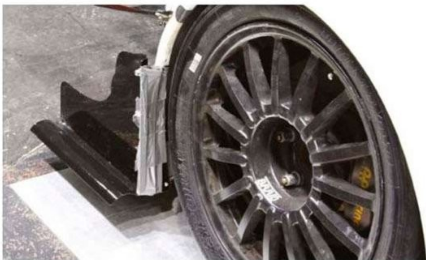
Race tape helped the splitter end plates to deliver more front downforce
