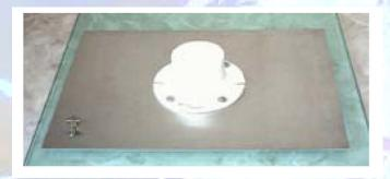
Now back to the PVC flange, using (4) 8-32 bolts, <sup>3</sup>/<sub>4</sub>" long, (4) large flat washers, (4) flat washers and (4) nuts. We will mount the PVC flange. Place a large flat washer over bolt, and then push thru PVC flange.
