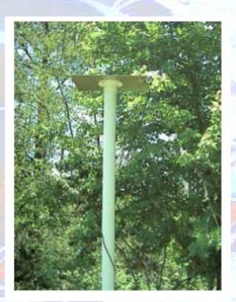
Force down all the way. Using 3 Sheet metal screws, to secure your PVC pipe to the Base, thus a movable antenna or you may glue in for a more permanent antenna. You can use tie wraps to hold coaxial cable to the pole.
