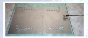
OK! Grab your drill and make those 6 holes, you may file away any burrs. Get that Coaxial Ground Block and mount it just as on the Antenna. Using 8-32 X ½" bolts thru Coaxial Ground Block, push into SS Top Plate and on back side, place your flat washer and tighten nut securely.
