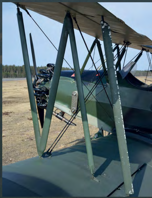
Top right Powered by a seven-cylinder Siemens Halske Sh13A4 radial engine, the Viima has a top speed of around 100kts (186km/h).
