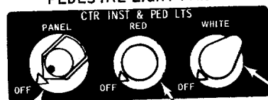
CENTER INSTRUMENT AND PEDESTAL LIGHT PANEL
