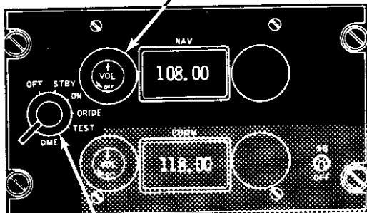
VHF NAV/COMM CONTROL PANEL
