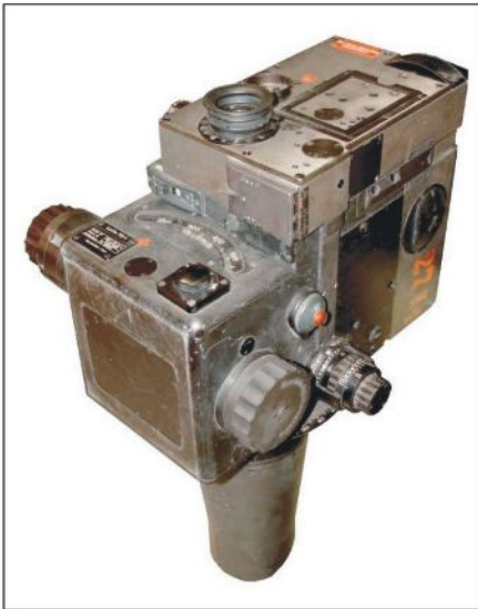
Above: Germany's Lotfe 7 was simpler than the Norden sight. Right: Nazi agent Herman Lang copied the Norden's plans.
