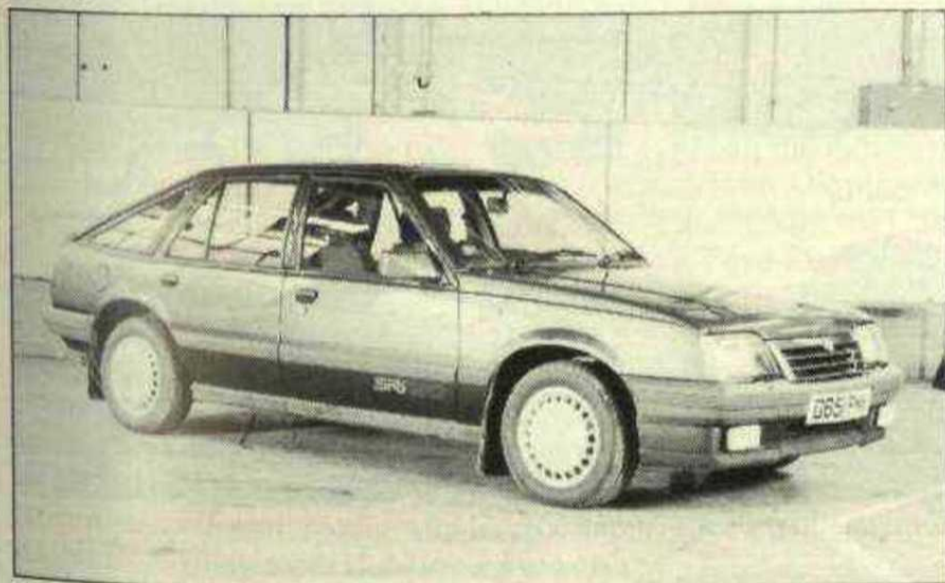
Second facelift for the Cavalier includes unappealing slotted grille. SRi 130 has deeper spoiler.
