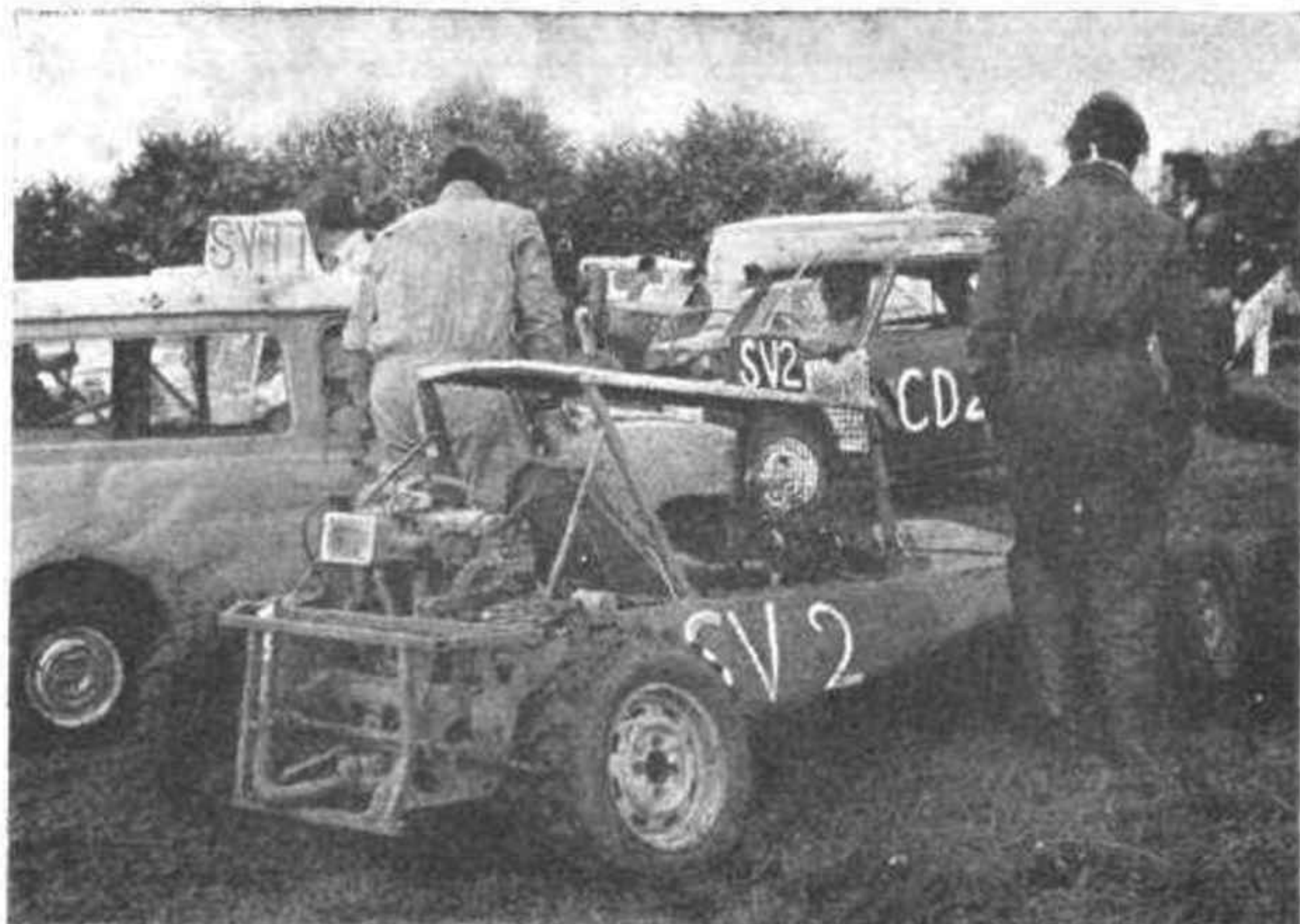
A TYPICAL jalopy at a meeting near Leominster. This one has a mini front end mounted at the rear and adapted for rear-wheel drive.
