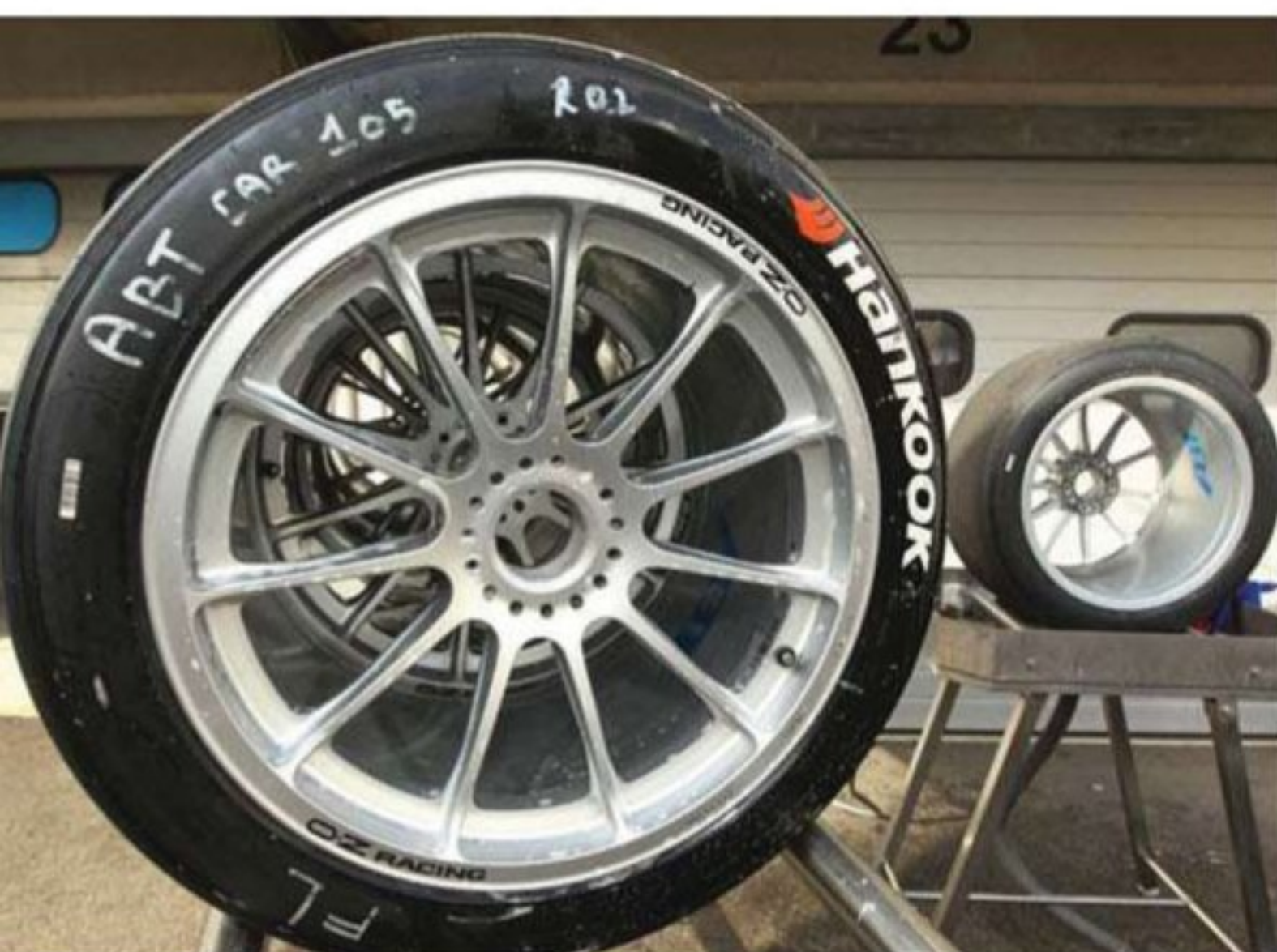
With more emphasis on mechanical grip and suspension tuning, as opposed to aerodynamics, tyre supplier, Hankook, has produced a wider rear tyre
