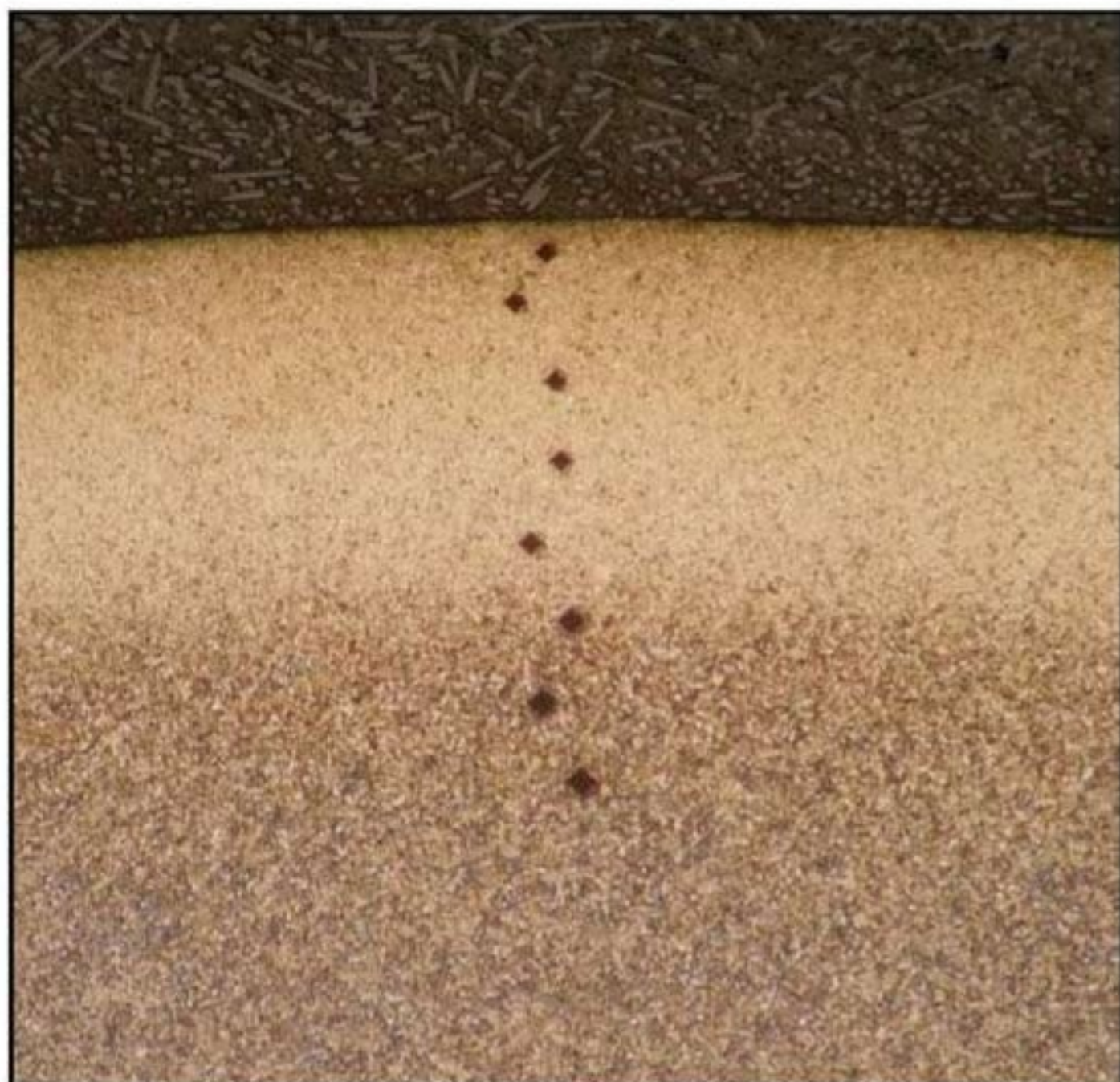
Figure 4: a 'micro-etched' section of the 9310 camshaft and associated micro-hardness profile diamond indentations
