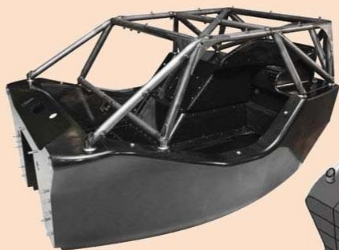
Development of the carbon tub and roll-over structure was led by Mercedes-Benz, then agreed by all three manufacturers before being built by an outside source
