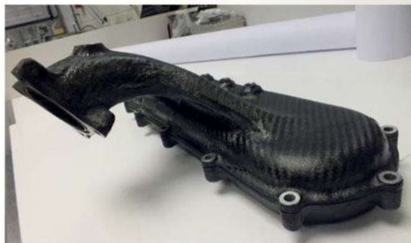
Low height carbon plenum is one of the few parts from the interim engine
