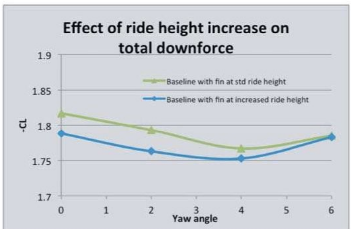
Figure 6: the effect on the 'baseline plus engine cover fin' specification of increasing the ride height
