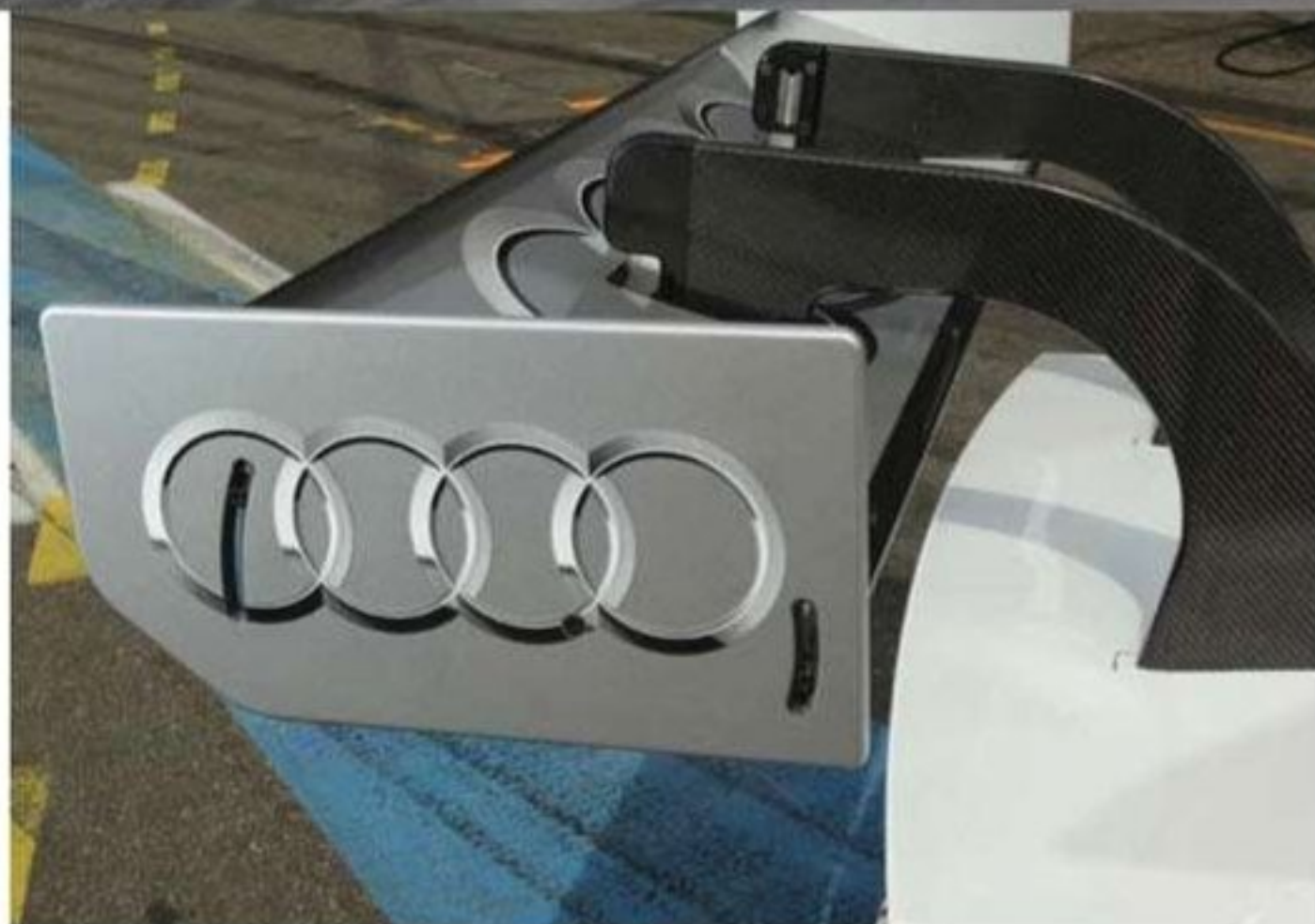
The rear wing, with its swan neck supports, will work in conjunction with the giant rear diffuser to produce vast amounts of downforce
