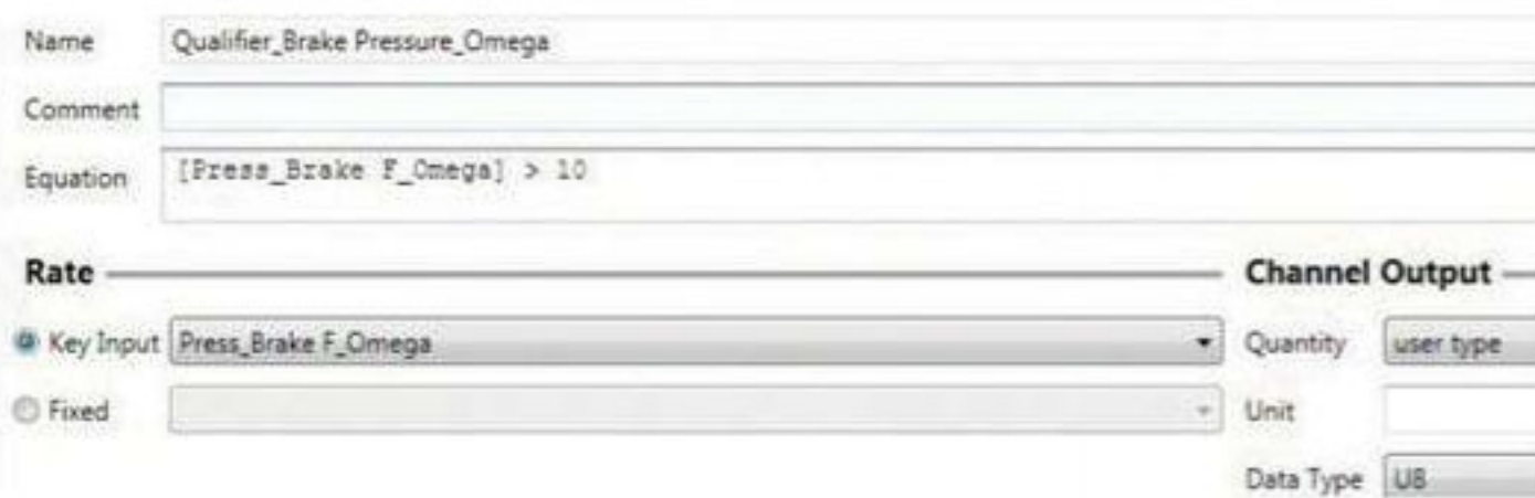
Figure 4: system state for brake balance activation. This maths channel goes to 1 as soon as the brake pressure reaches more than 10bar
