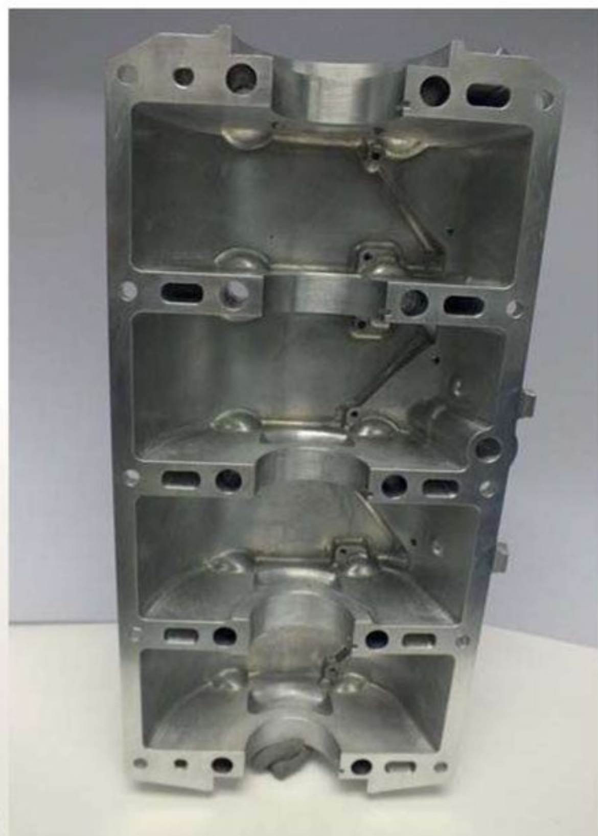
Main picture: drilled crank with tungsten weights is an extraordinary piece of engineering, and weighs just 7.8kg. Sump (above) is milled from a solid lump of 7075 aluminium and weighs just 4kg
