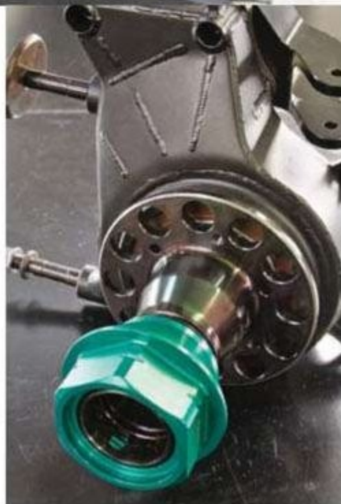
Right: new front uprights feature larger bearings and hubs but retain the lower pushrod mounting concept of the F308
