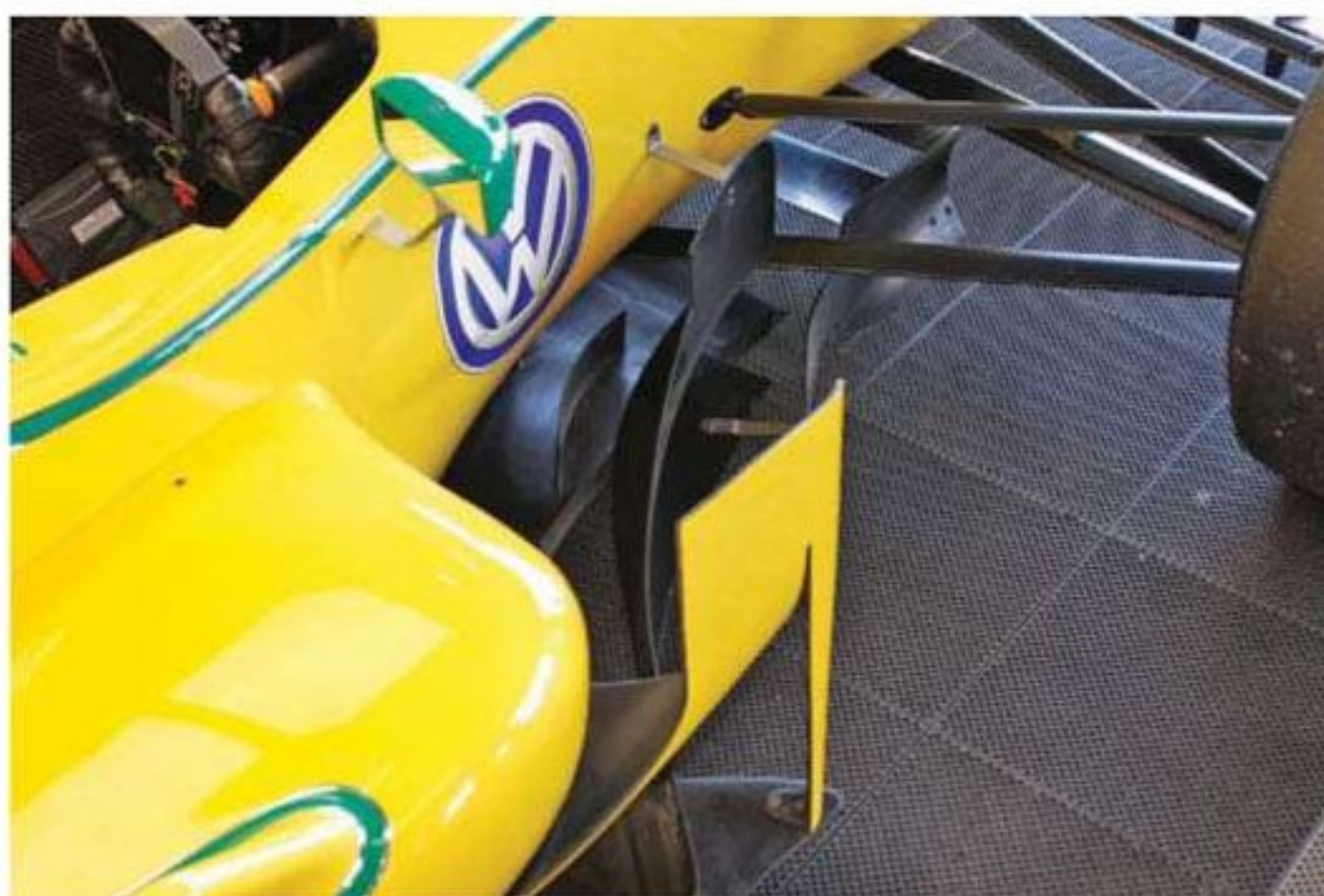
In 2011 spec, the F308 sported a number of aerodynamic devices ahead of the underbody that have now been outlawed by the new regulations
