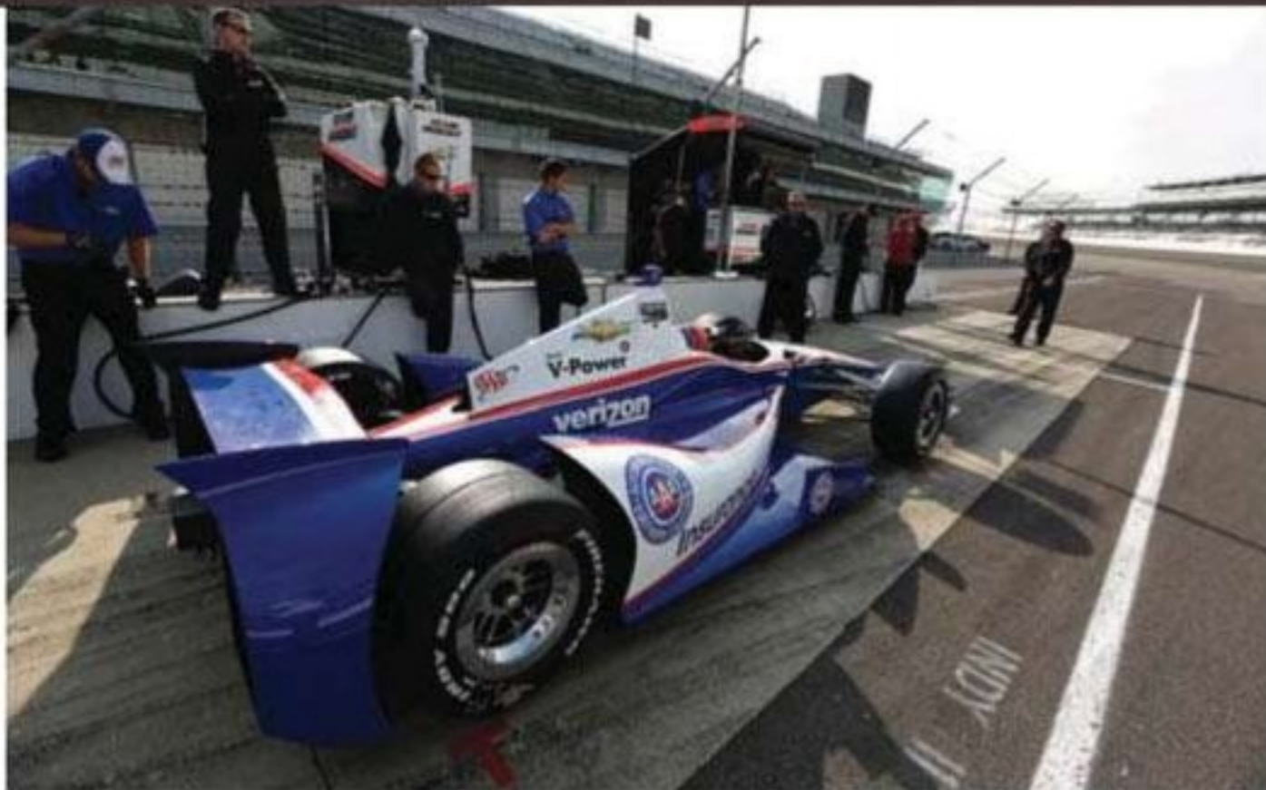
In order to improve the car's balance, new inboard mounting blocks were made for the rear suspension, and the front and rear suspension pick-ups modified so the wheelbase is now one inch back at the rear and two inches back at the front. Only the front wishbones had to be re-manufactured
