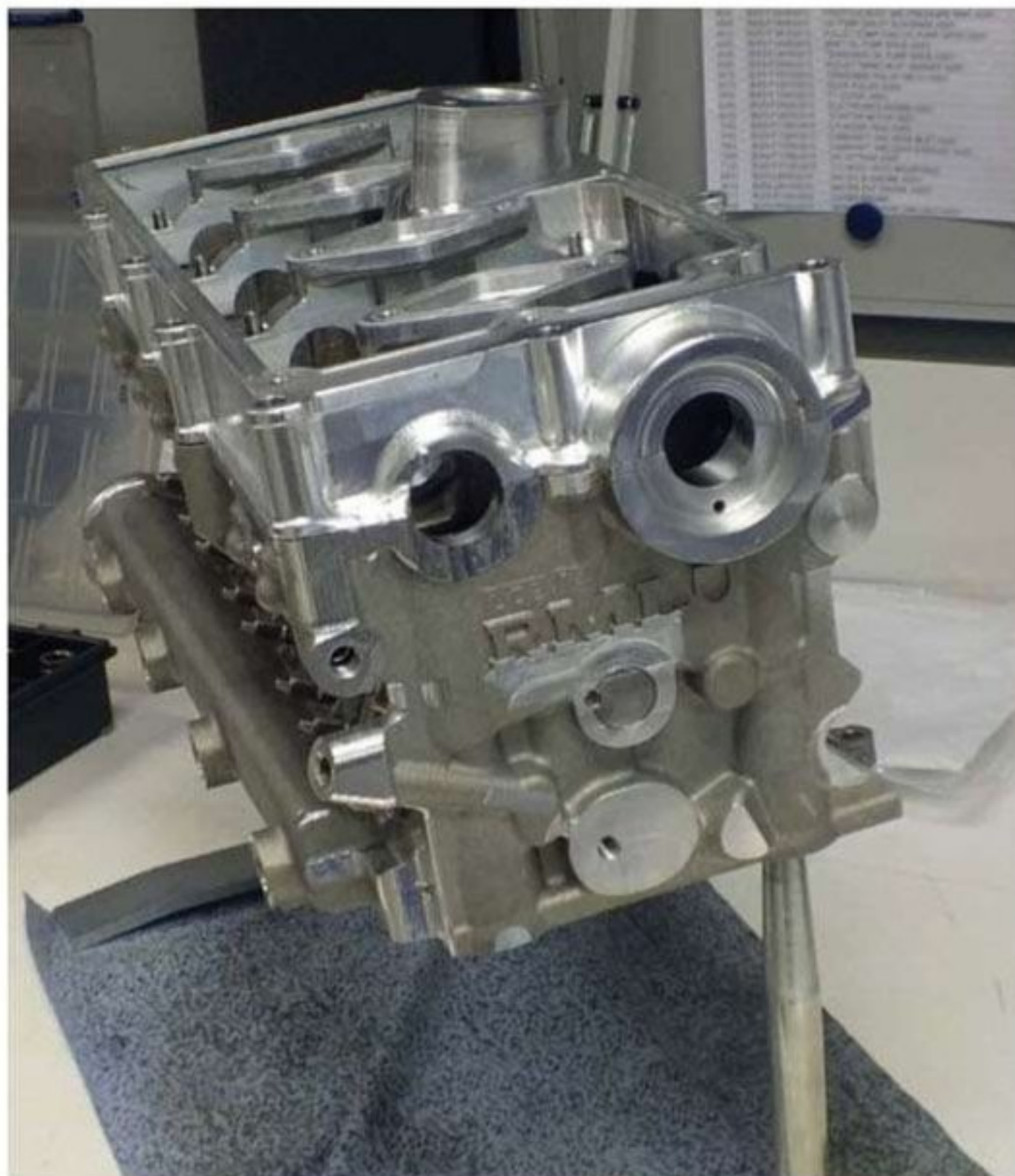
Above: every part of the engine was designed by RML, including the non-structural aluminium block, that weighs just 15kg
