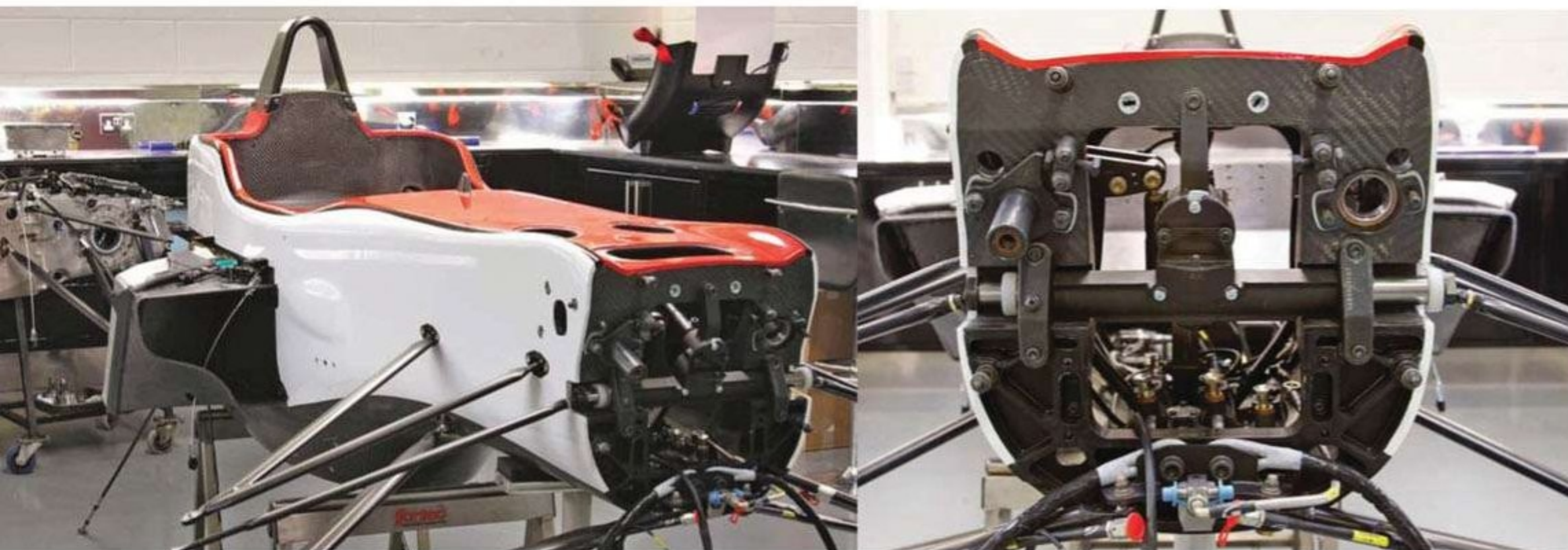
All new carbon composite monocoque approaches Formula 1 safety standards, and features new side intrusion panels
