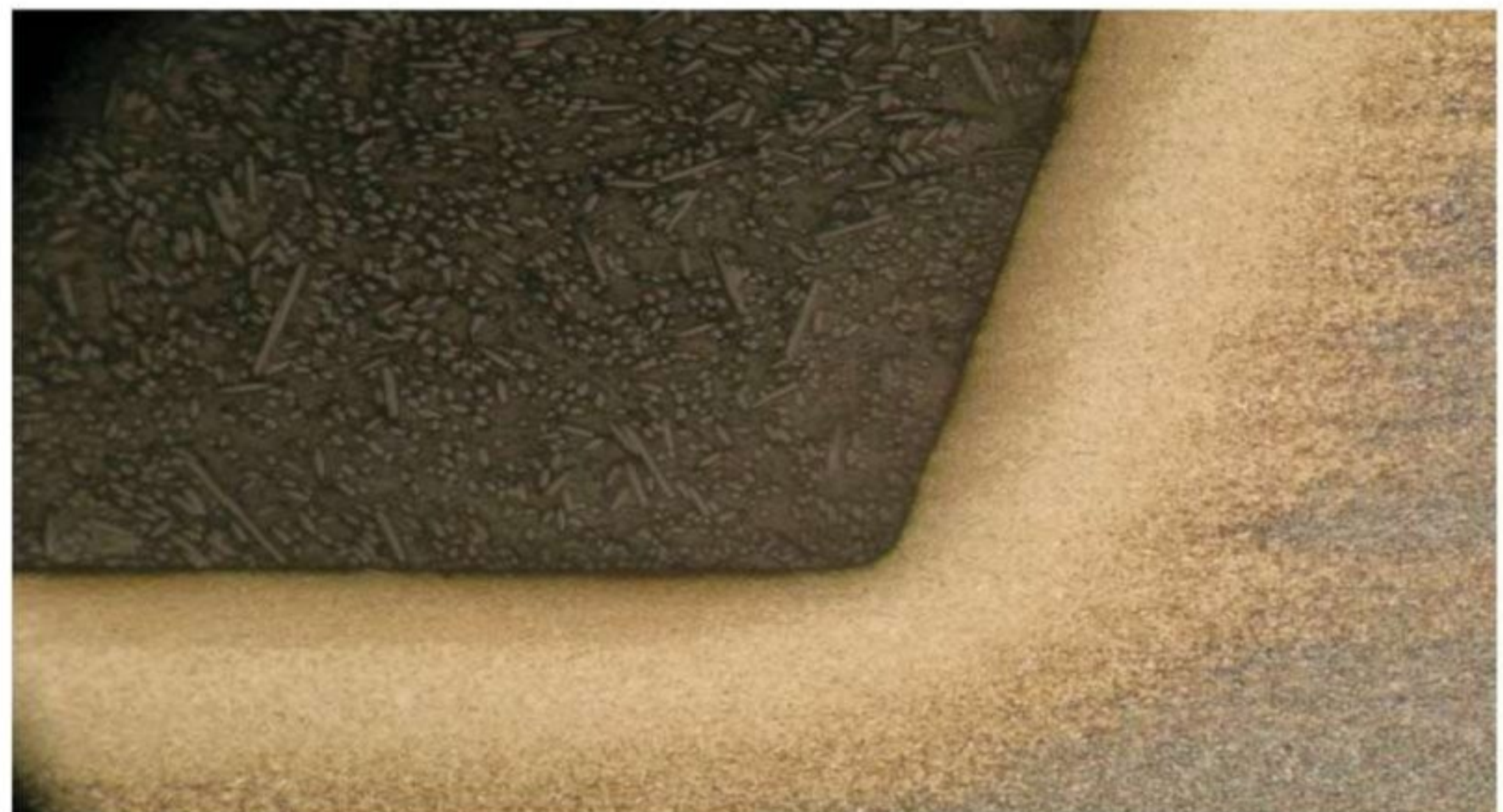
Figure 2: this shows the uniform, fine grain structure free of coarse precipitated carbides that is imperative for optimum bending fatigue resistance
