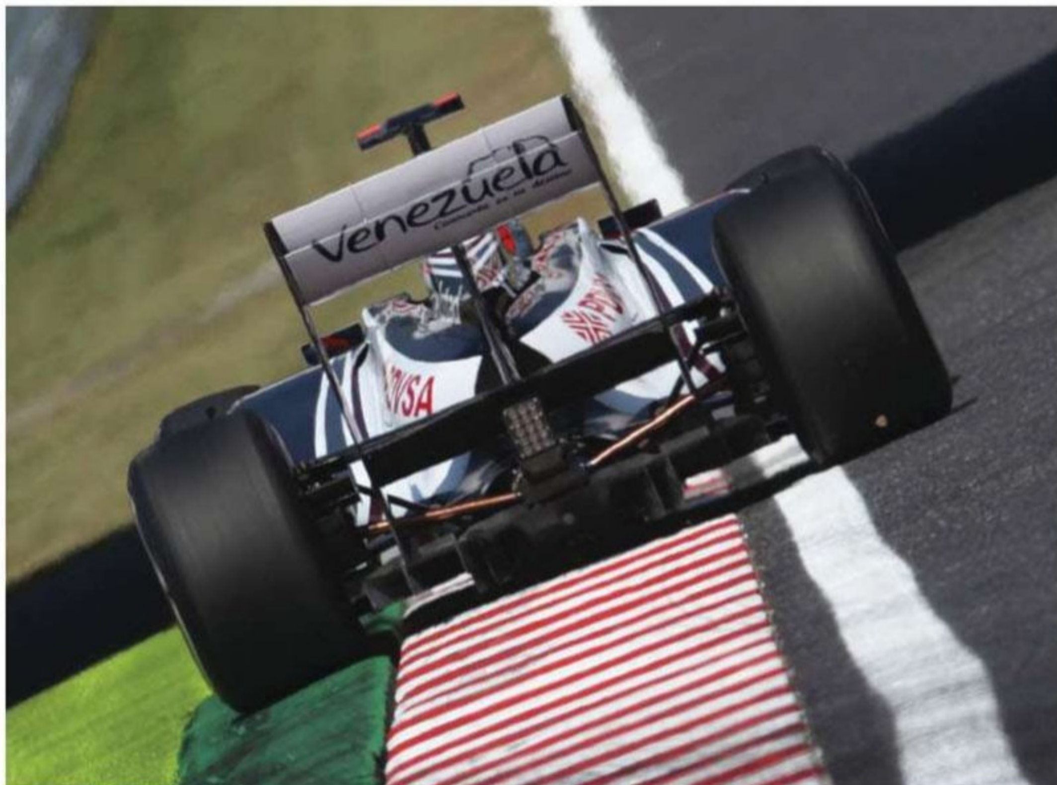
The Williams FW33 of 2011 had a very low gearbox, meaning extreme driveshaft angles were required
