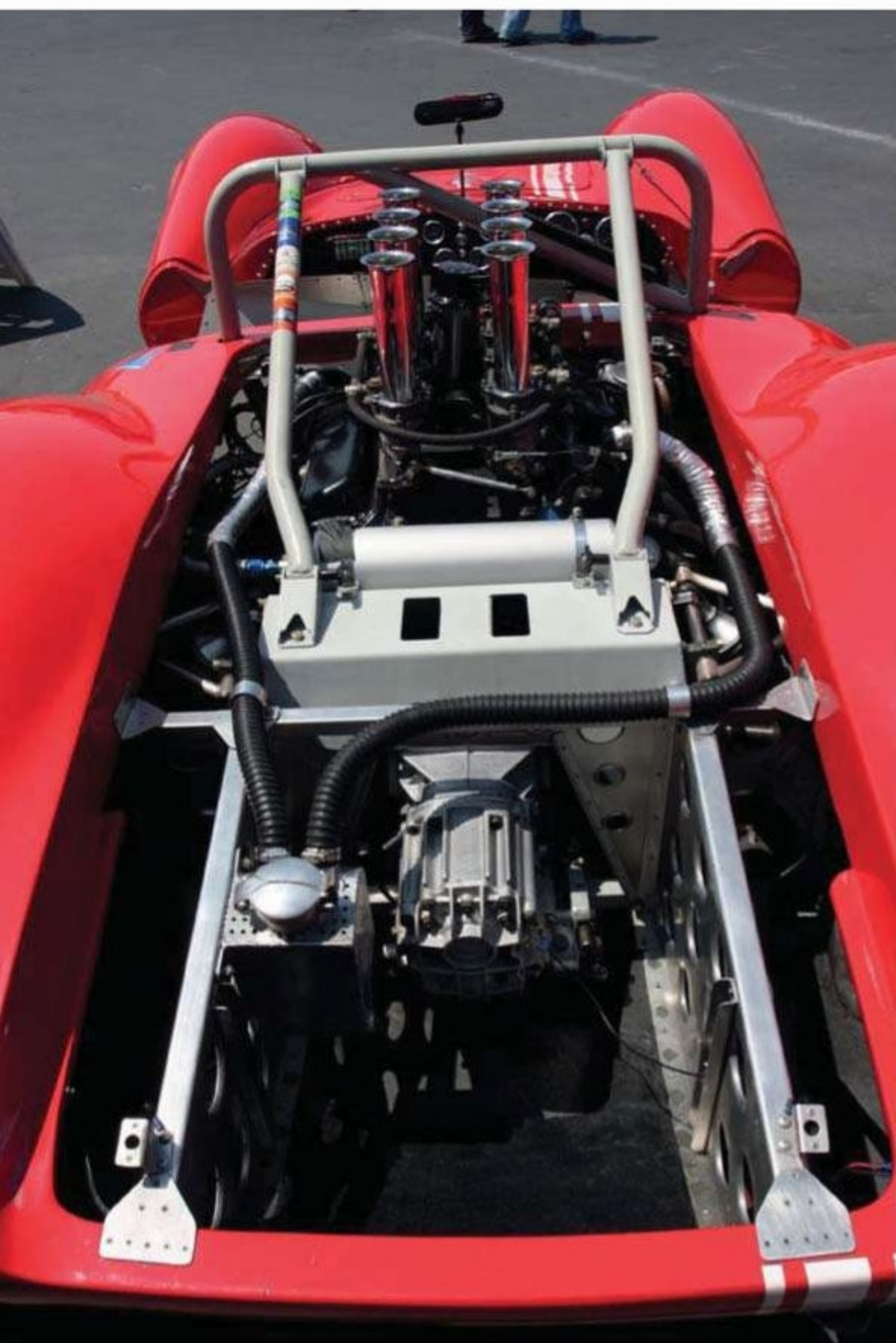
The folded steel backbone chassis is clear in this view
