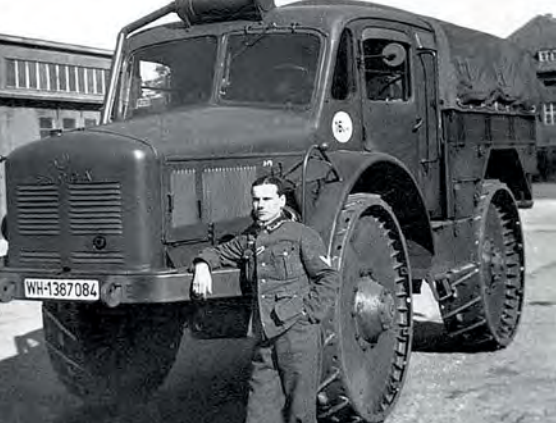
Looking factory-fresh with its shallow cleats, this was the Radschlepper Ost reporting for duty. It proudly carried the name of its maker
