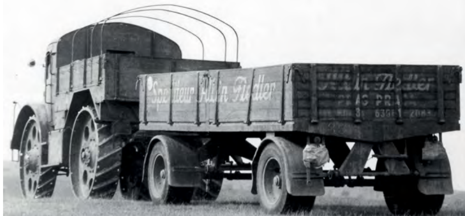
In towing trials the Skoda RSO was rated at five tons capacity. On hard surfaces it was notable for the noise generated by its steel wheels
