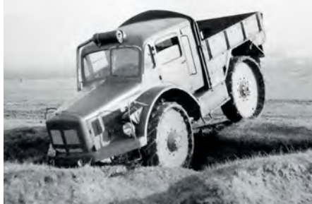
Shallow cleats figured in the Type 175's tests in final form, this one wearing its bonnet sides. The driver's windscreen could now be opened
