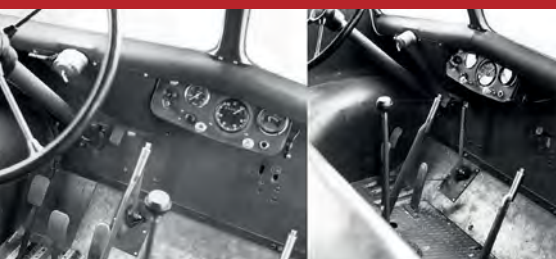
Instrumentation of the prototype Skoda RSO showed oil pressure, fuel level and engine revolutions plus a totaliser
