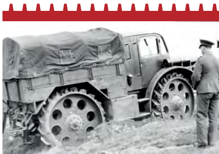
The trials near Mladá Boleslav were not without their setbacks. Certain surfaces were troublesome to the Type 175, leading to changes in its gear ratios
