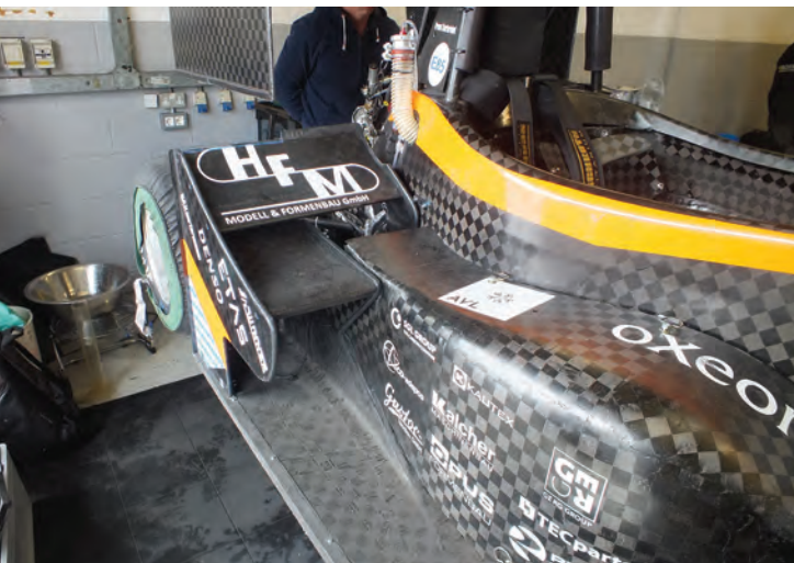
TU Munich was one of a number of teams who attempted to recapture lost downforce via the use of sidewings – overall winner TU Delft also used these
