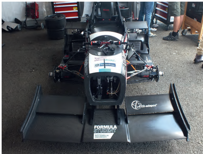
The ETH Zurich car is driven by four student-designed hub motors and boasts a neat composite monocoque
