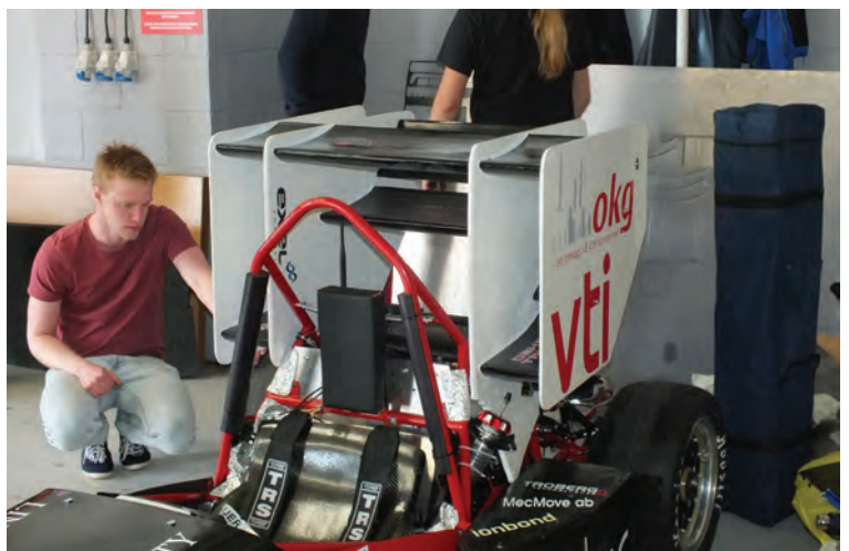
Linkoping arrived with perhaps the most wing elements ever seen on a FSAE car. We lost count at 11 in the rear wing alone. Team claims to have optimised wings
