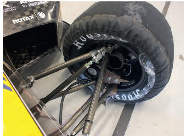
The Karlsruhe car also needed to use cooling fans on the front brakes as a consequence of the front wing reducing the air flow over the disc and caliper
