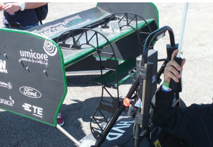
Swan neck rear wing supports were used by some teams but derided by others, a number of teams also opted to use these very delicate lattice-like swan necks
