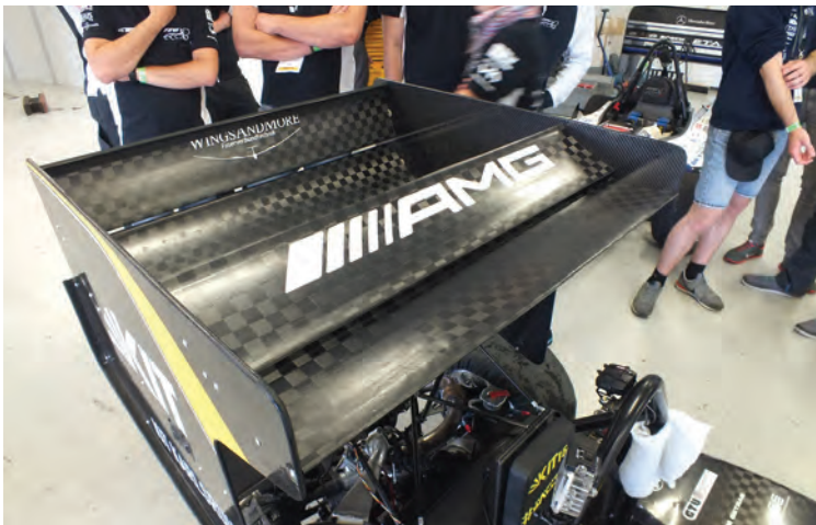
The Karlsruhe car sported an apparently Benetton B193 inspired rear wing with a forward element – the German team was one of a number of competitors to opt for this style of wing
