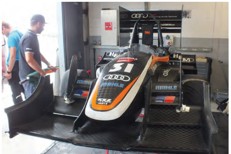
The level of complexity of the aerodynamic packages on the 2015 cars went beyond anything seen before as teams tried to claw back aero lost to new rules
