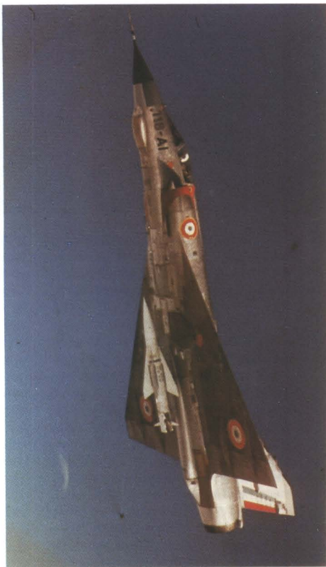
Above: A Mirage IIIE of the Armée de l'Air displays the tailless delta configuration adopted for high-speed, high-altitude interception.
