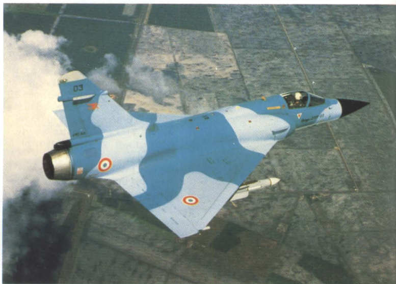
Above: The automatic leading edge manoeuvre slats and the two-section elevons are used to produce variable camber.
