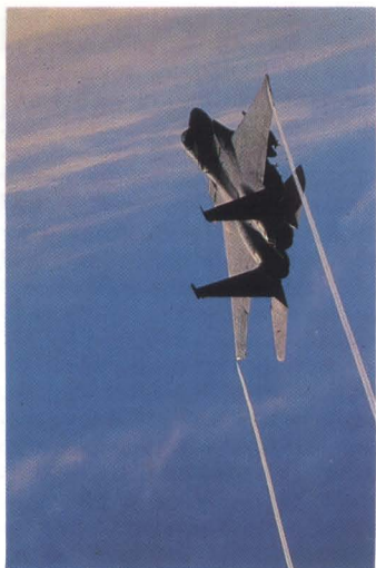
Above: streaming contrails from its wingtips, an F-15C Eagle reefs into a hard turn using military power only.
