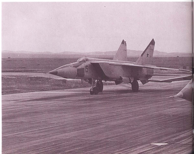
Above: The Foxbat-E seen here carrying four AA-6 missiles is an upgraded Foxbat-A, with High
