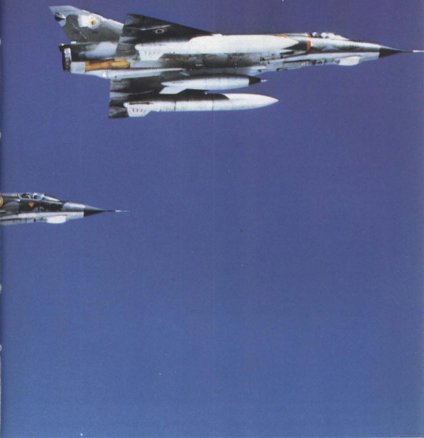
Above: Three Mirage IIIEs of the Armée de l'Air carry (right to left) air-to-ground, air-to-air and anti-shiping weapons, plus drop tanks.
