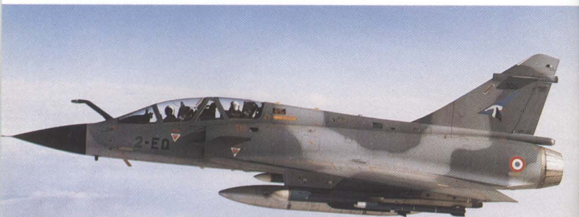
Above: The automatic leading edge manoeuvre slats and the two-section elevons are used to produce variable camber.
