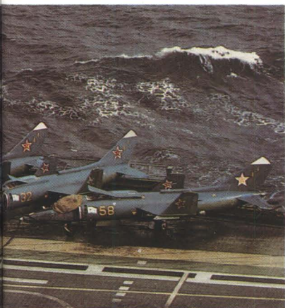
carrier Kiev. Forger combines two lift engines with a vectored-thrust main engine for V/STOL capability.
