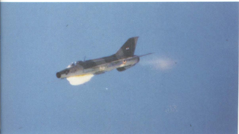
Above: MiG-21bis Fishbed-L of the Soviet Air Force. Lack of range and poor visibility from the cockpit are two drawbacks.
