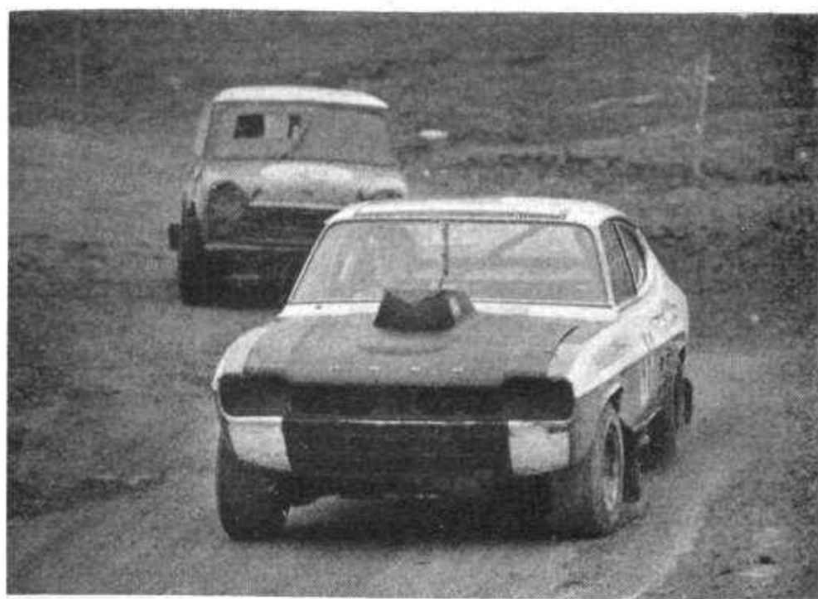
FORD's four-wheel-drive Capris have been extremely successful as they have become developed. This car driven by Roger Clark features a 250-b.h.p. engine with aluminium heads and fuel injection.
