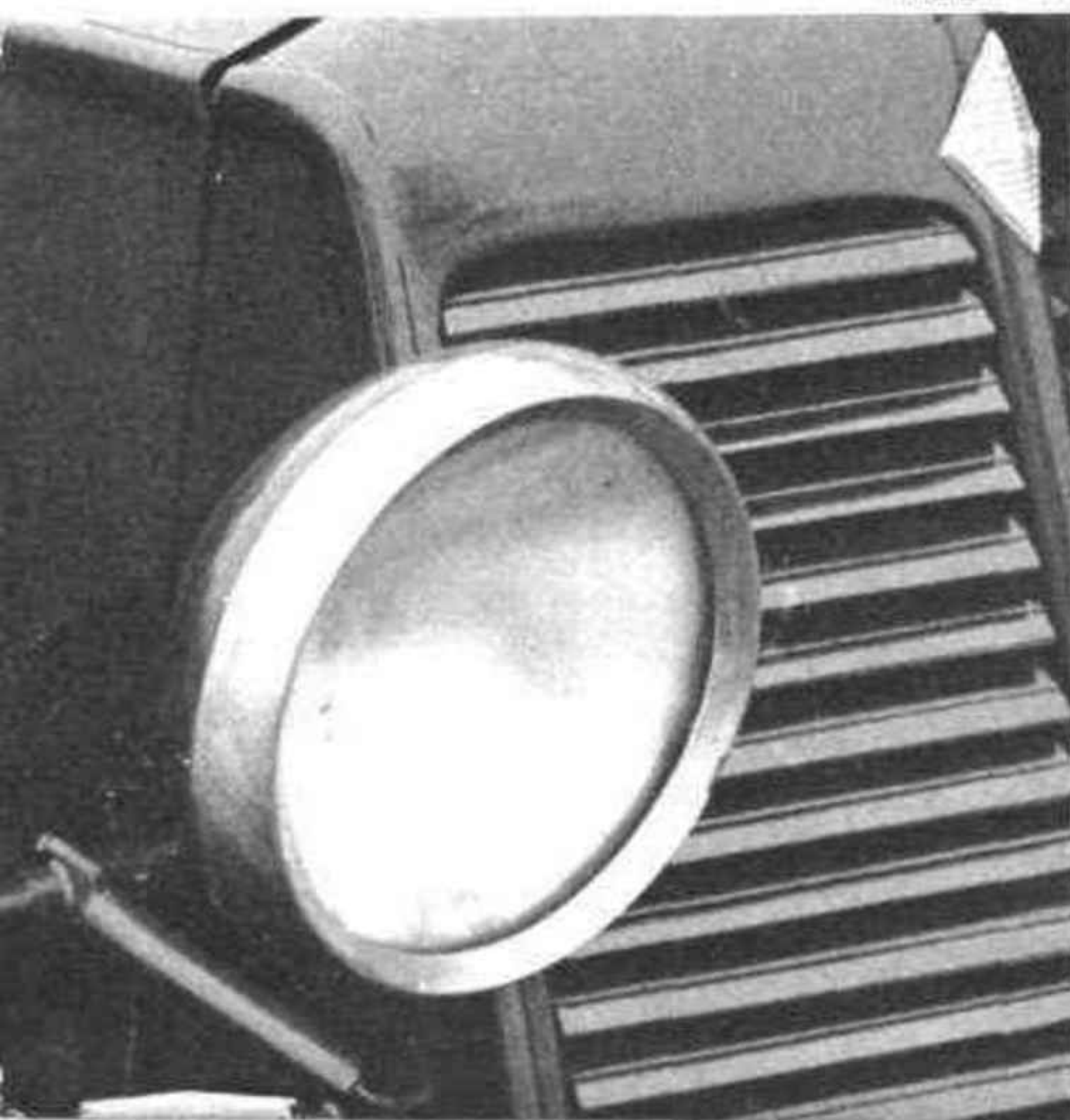
SOME RENAULT NERVASTELLA DETAILS.—From l. to r., the frontal aspect, showing the thermostatically-controlled radiator shutters, the rugged spare wheel mounting, and the equally rugged headlamp anchorage.
