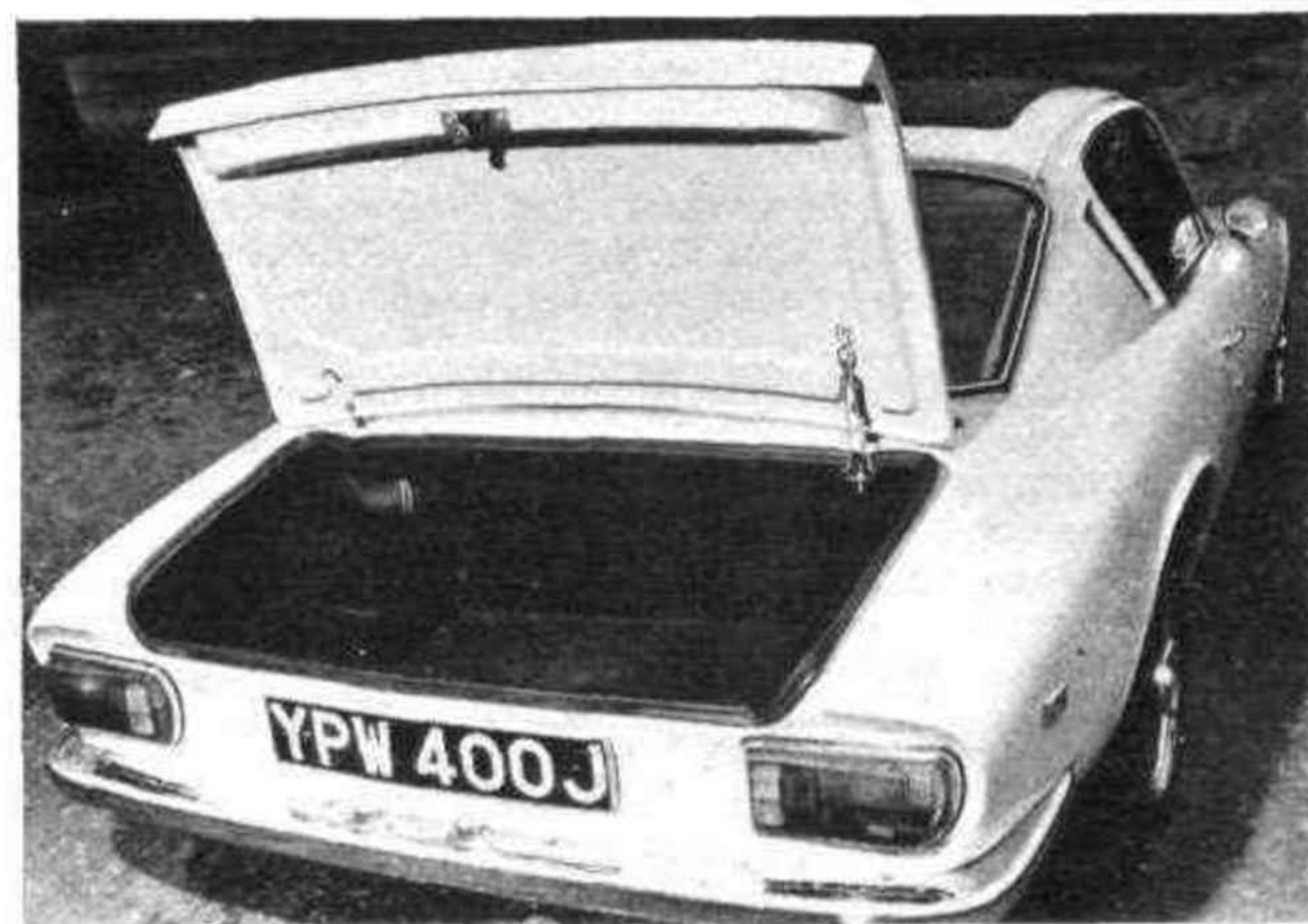
SPACIOUS BOOT for the +2S which is opened from a pull knob in the well of the driver's door.
