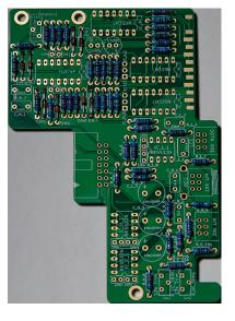
After Placing and Soldering all Resistors, we solder the next bigger parts like IC-Sockets and small capacitors, like Yellow 100nF and capacitors next to IC Sockets. On the LED Meter Board we also add the electrolytics and Wima Capacitors and Board connections, and cut leads after soldering as short as possible. We will do this process later with Potentiometers also, since we need to make sure that this Preamp doesn't touch any neighbour modules of any kind.
