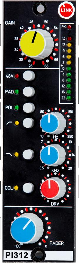
The Peak LED is pre set to +18dBu directly after Preamp
