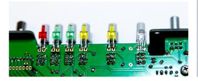
After soldering all LEDs tot the Mainboard unscrew the Frontpanel again. Put the 25mm Spacers on the Mainboard and add the LED-Meter Board. Use the screws to secure the LED-Meter Board. Put the Frontpanel back on again and tighten the Nuts to the bracket. Now we will finally solder the remaining legs of the Pots as they should be perfectly centered now.
