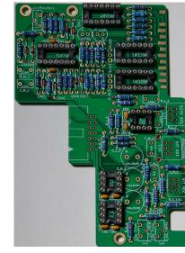
After that Step solder all Wima Capacitors, Electrolytics and Board Connectors as on the pictures.
