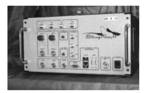
One of the so-called stingray cell phone tracking devices, which impersonates a cell tower.
