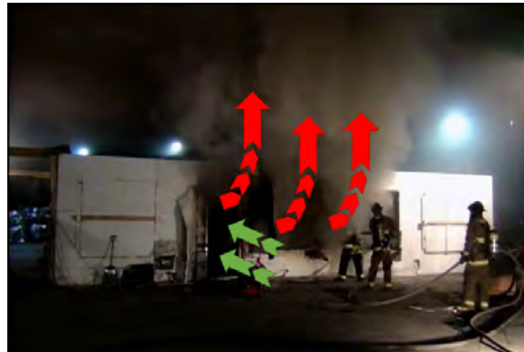
(c) Flow with Positive Pressure Ventilation
