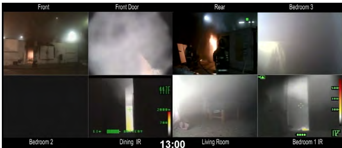
(f) Suppression - Straight Stream Bedroom 2 Window
