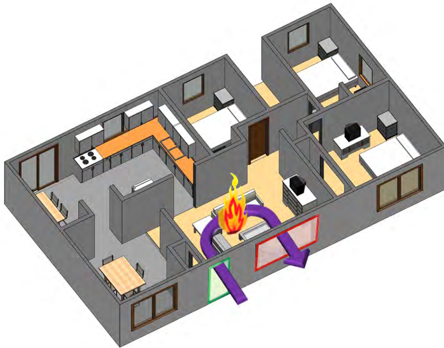
Figure 9.1: Experiment 1 Ventilation Configuration
