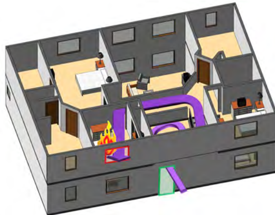
(f) Second Floor Ventilaion Profile
