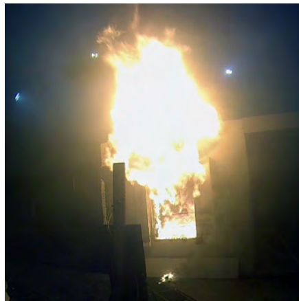
(c) Exhaust Without Fan Flow - Post Flashover
