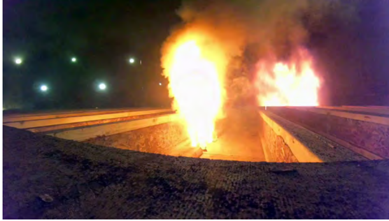
Figure 10.41: Fire From Simulated Balloon Frame Stud Cavity Prior to PPA
