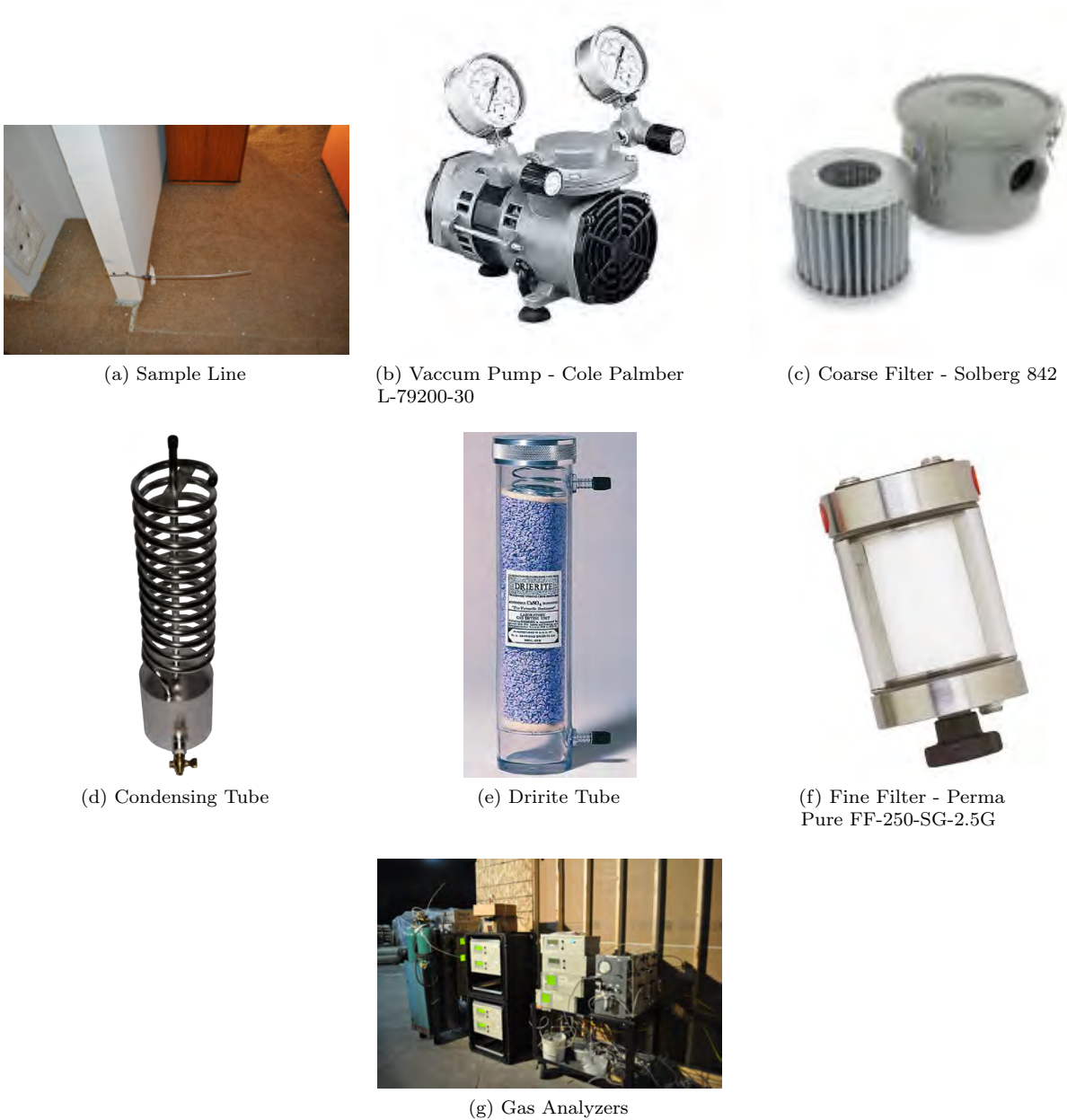
Figure 5.8: Gas Analyzer Configuration
