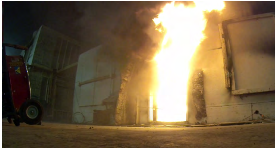
Figure 10.14: Vent Point Ignition of Fan Inlet During Laboratory Experiments
