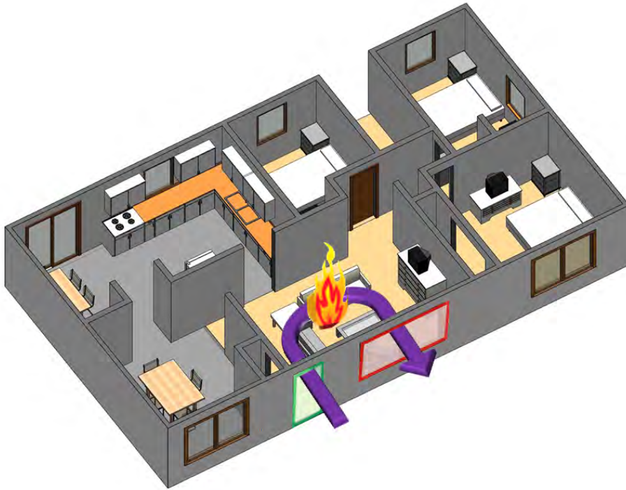
Figure 9.3: Experiment 2 Ventilation Configuration
