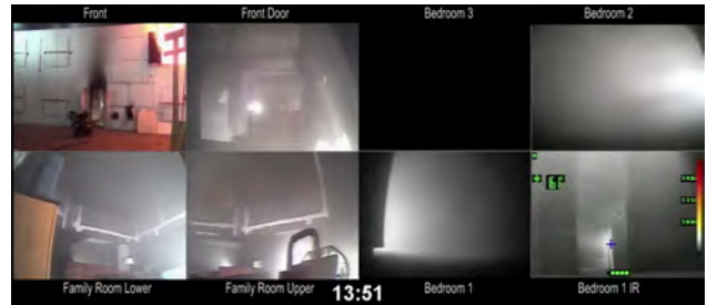
(f) Compartmented Fire (Bed 3) 1min After Fan On
