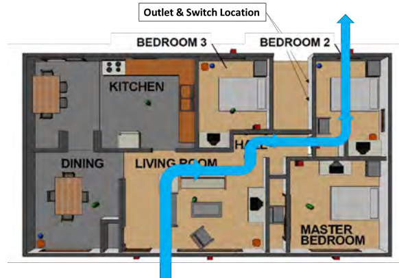
(b) Outlet and Switch Locations
