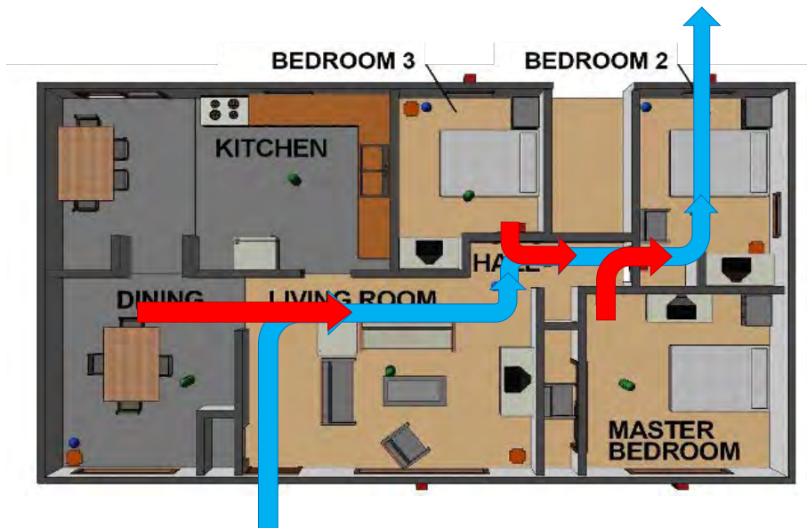
Figure 10.50: Air Entrainment From Connected Spaces
