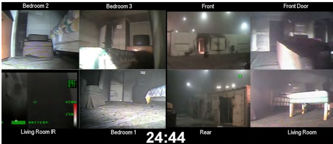
(i) Kitchen Door Open & Bedroom 3 Window Closed
