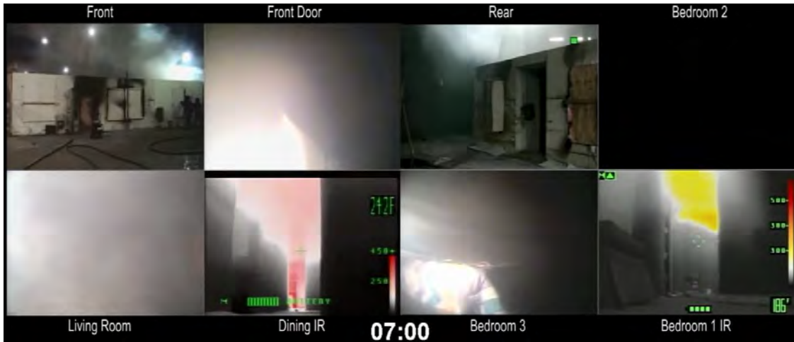
(b) Vent Master Bedroom Window
