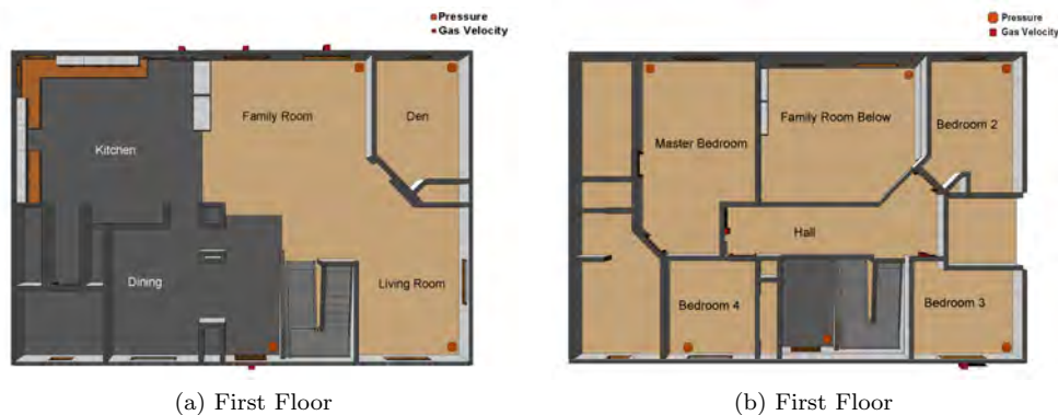
Figure 8.3: Single Story Cold Flow Sensor Locations
