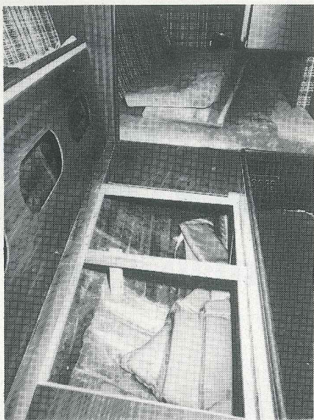
There are storage lockers beneath all the berths. This one, under the starboard saloon berth, extends aft beneath the quarterberth almost to the transom
