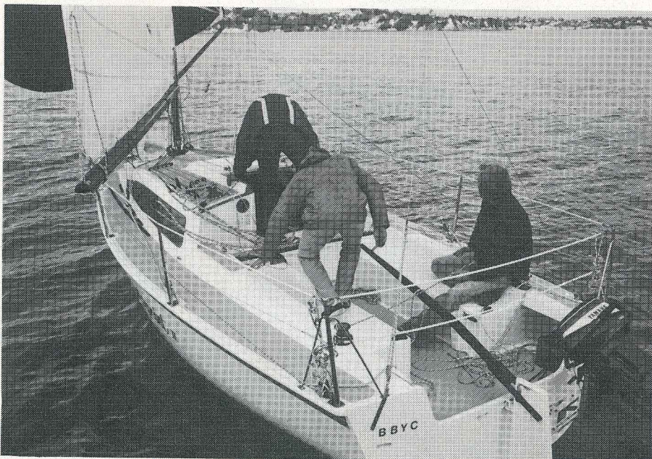
Below: Cockpit is large, with T-shape giving storage room against the cutaway transom for fuel can and gas bottle
