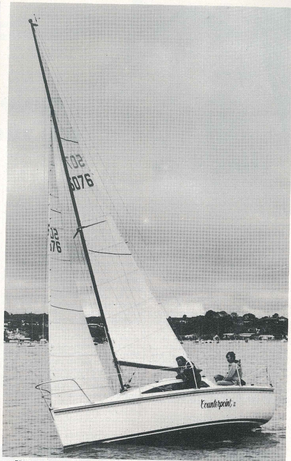
Plumb stem and transom and low coachroof give the SR26 rakish good looks
