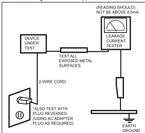
Figure 1-1. Leakage Current Test Circuit
