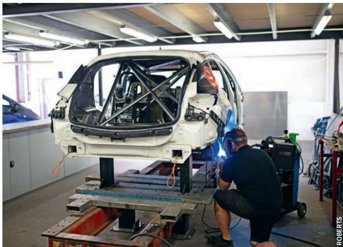
Clockwise from top: PMR has its own sub-assembly area to test the life of parts; adjustments are made on the jig after a bruising race weekend; Cook leads the pack en route to victory at Thruxton
