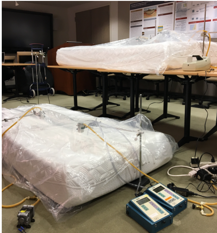
Figure 6: Still air monitoring set up with two mattresses assessed simultaneously.
