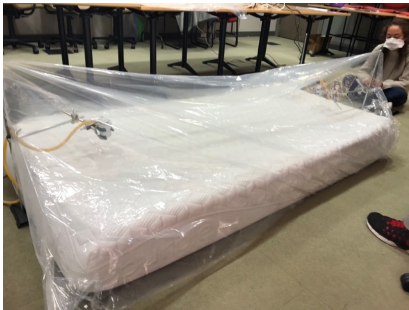
Figure 4 Opened mattress within the plastic bag showing the sampling locations at either end of the mattress. On the left is one filter set up and one DustTrak sampler probe. On the right end, are two filter set ups and the CP probe and another
