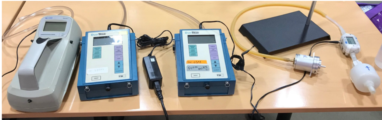
Figure 3: Equipment used: Left to Right, Continuous sampler CPC – TSI 3007, DustTrak set for PM 2.5 , DustTrak set for PM 10 , Filter Holder, and TSI Flow meter (4000 series 0-20 LPM).
