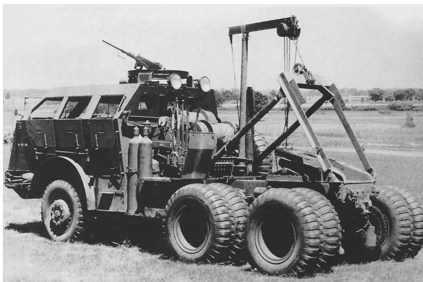
A—BLACKOUT DRIVING LIGHT B—PIONEER TOOLS C—BLACKOUT CLEARANCE LIGHT D—SERVICE CLEARANCE LIGHT E—CAB WINDOW ARMOR SHIELDS F—DOOR WINDOW ARMOR SHIELD G—DOOR H—STEPS J—ACETYLENE AND OXYGEN TANKS K—TOOL COMPARTMENT L—BRACKETS FOR VISE M—REAR WINCH PLATFORM N—FLOODLIGHT
