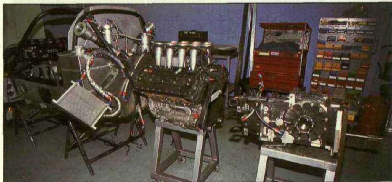
Main structure stops behind driver, allowing various load-bearing engine/gearbox combinations.
