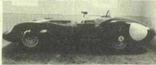
1959 LISTER JAGUAR-CHEVROLET. CHASSIS NO. BHL 130. Regarded as the most original Costin 'slippery' bodied car. Complete with original type 5.3 litre Chevrolet V8 (405 bhp) and Jaguar 3.4 (320 bhp) engines. Racing history in the hands of Mike Antony, Mike Pendleton and Jerry Marshall.
