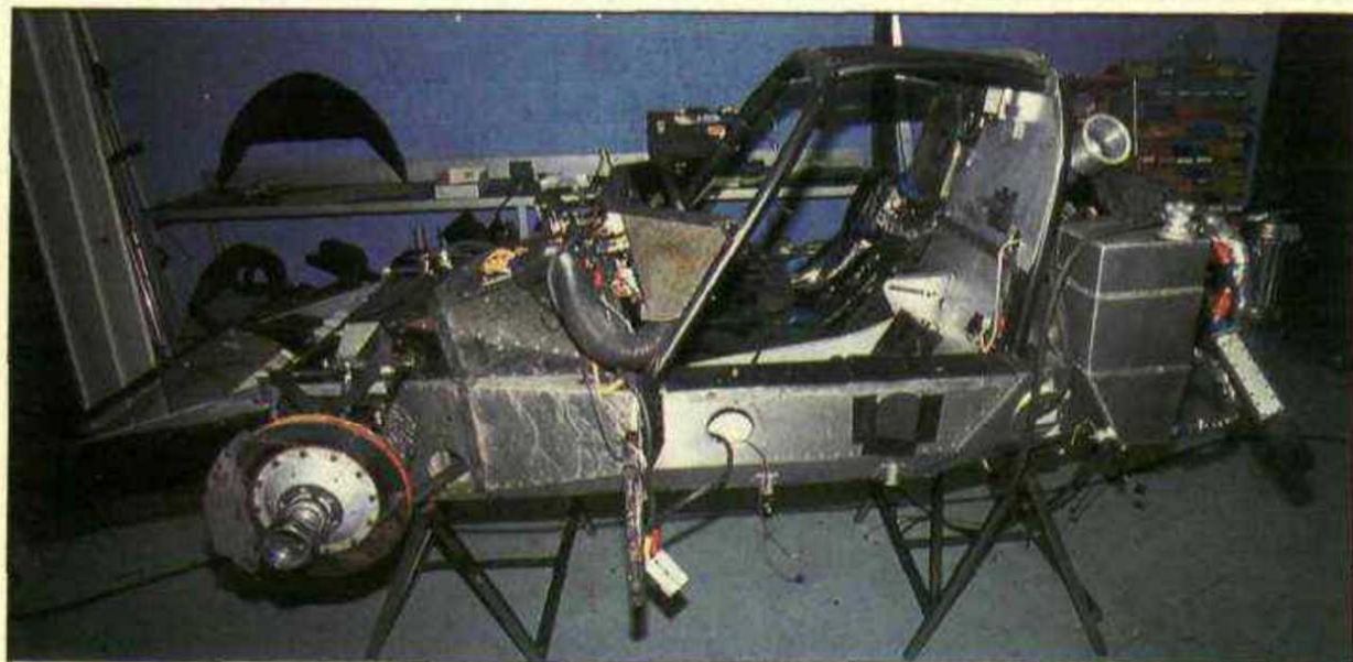
Stripped of bodywork, the aluminium monocoque with its rollage and push-rod front suspension.
