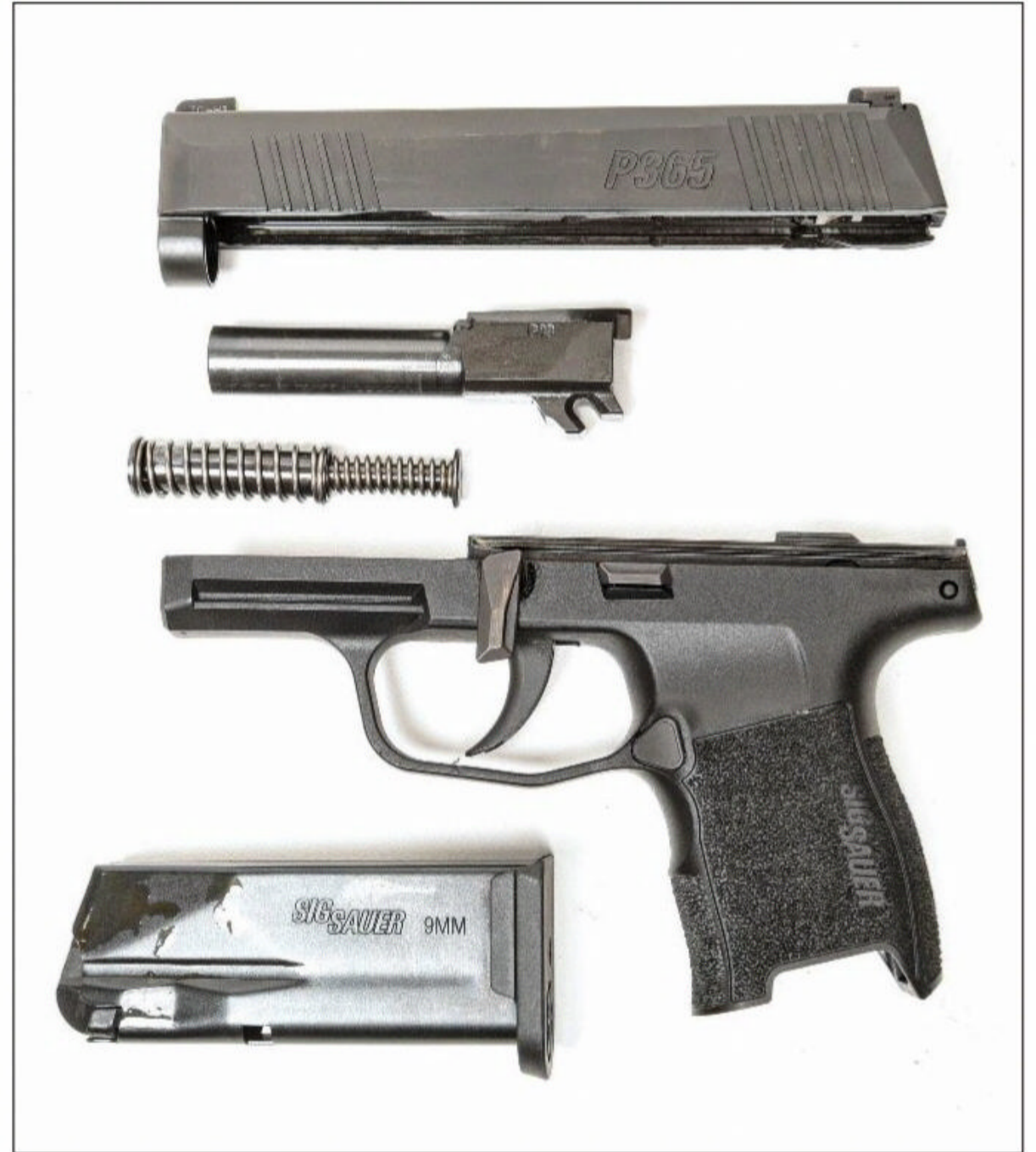
A look at the P365 stripped down, which is easily accomplished. Note the short 3.1-inch barrel and metal guide-rod assembly with captured dual springs.
