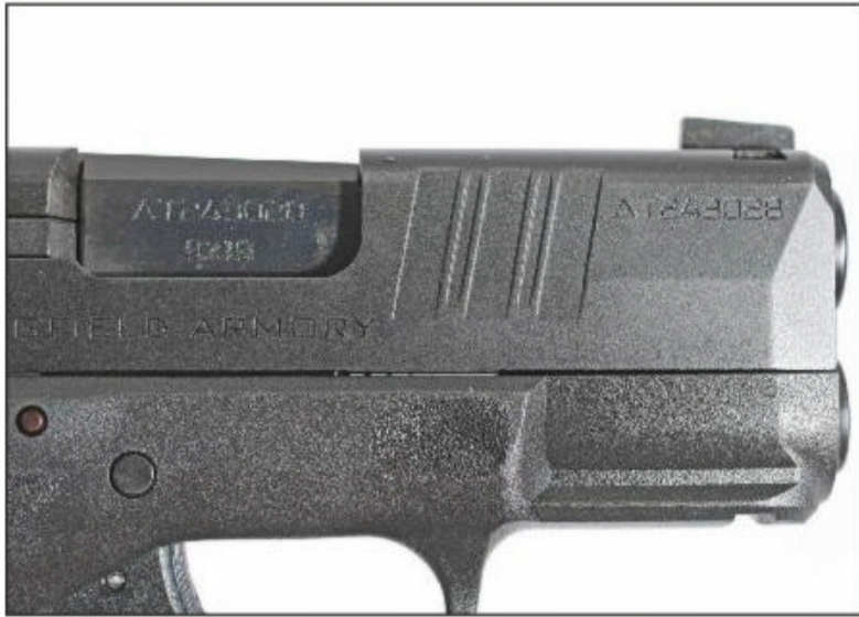
The cocking serrations are grooves in the slide, with the tops of the grasping ridges themselves grooved.
