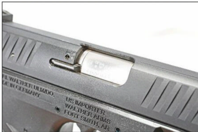
The ejection port is plenty big for the .380, and the extractor is robust for the work asked of it.
