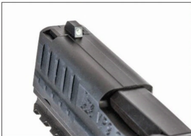
The front sight is steel. There is a tritium insert with a white outline. The forward cocking serrations are nicely aggressive.
