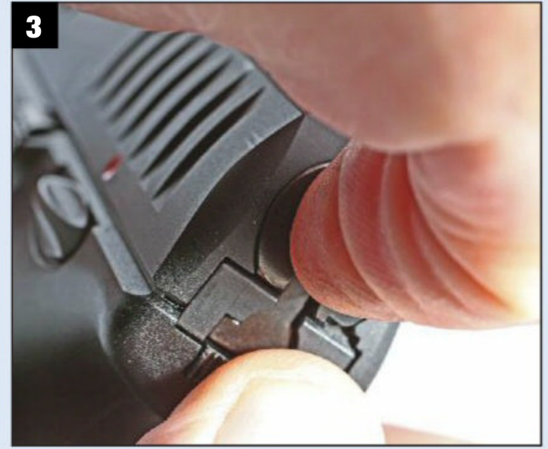
3 Then slide the retaining plate to the right....
