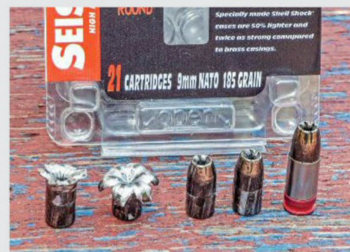
Tarr fired the Seismic 9mm ammo through a pistol (Beretta 92) and a Ruger PCC (from left to right) into both bare gel, and gel covered with heavy clothing. The bullets expanded in bare gel (much more so when fired out of the PCC), but did not expand when fired through gel blocks covered in clothing, although they did penetrate deeply.
