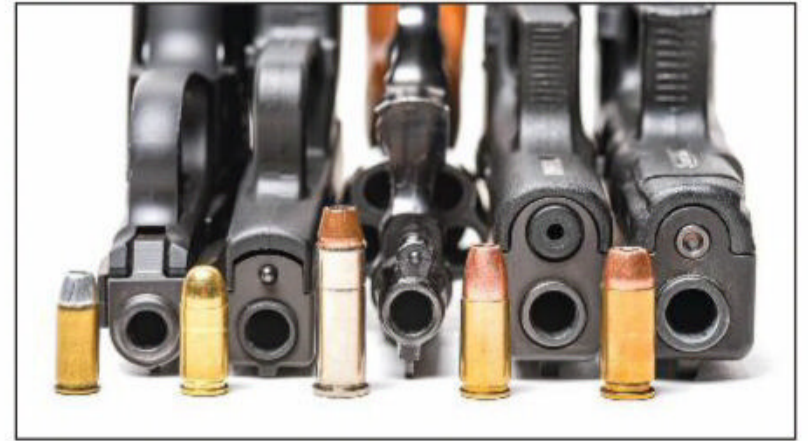
Caliber selection is important when choosing a pistol for personal protection, the 9mm (2nd from left) offers good terminal performance, high magazine capacity and controllable recoil.
