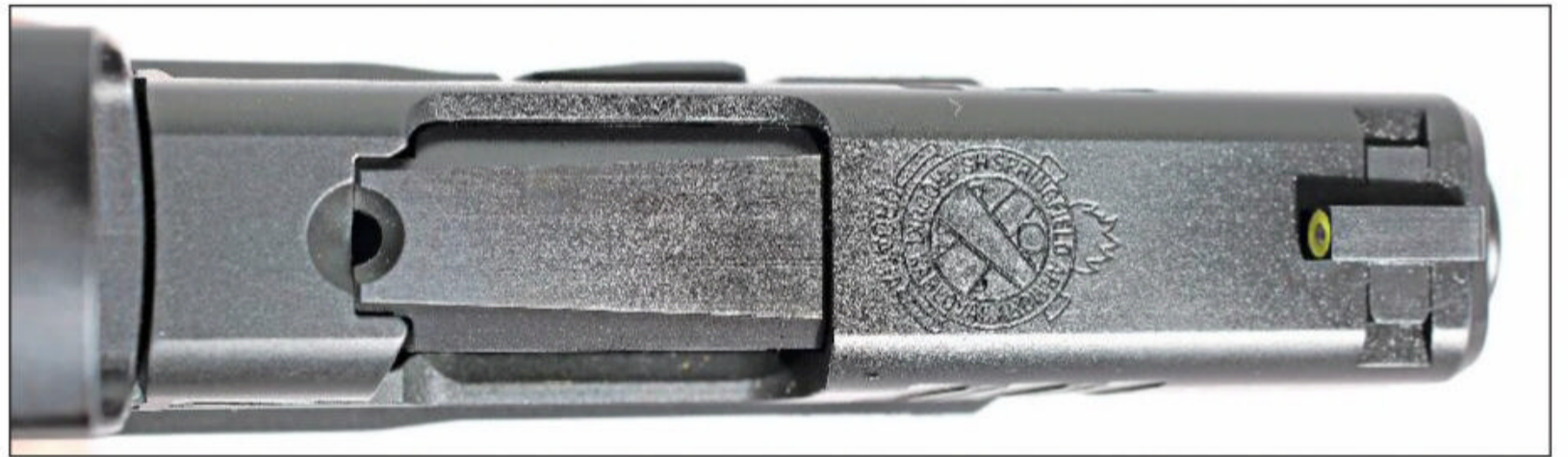
The loaded chamber indicator is simplicity itself: a viewing port on the rear of the barrel hood. Note the Springfield logo ahead of the chamber.
