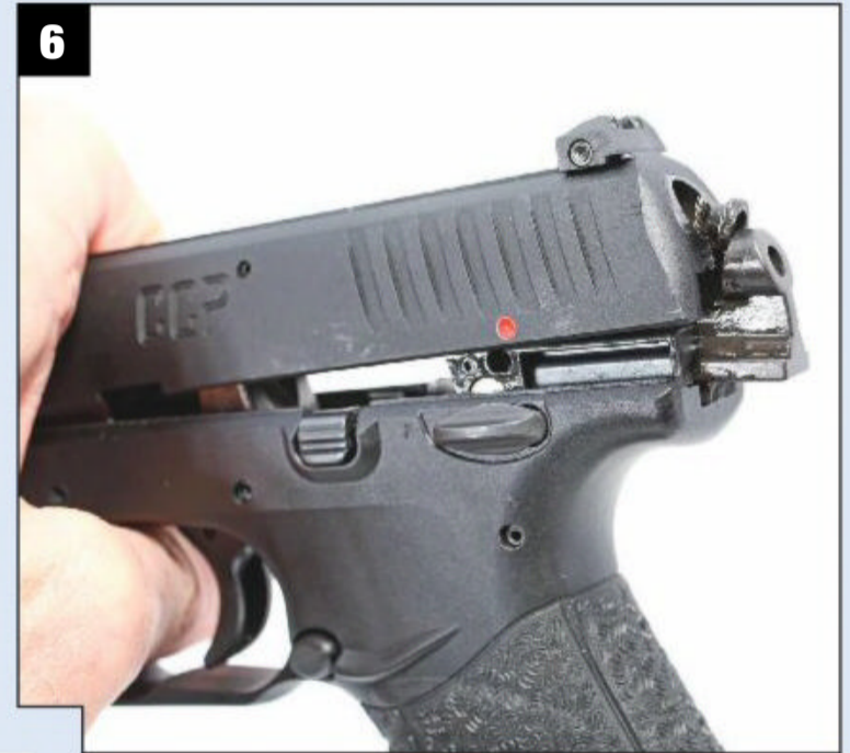
6 The slide can be lifted up off of the frame.
