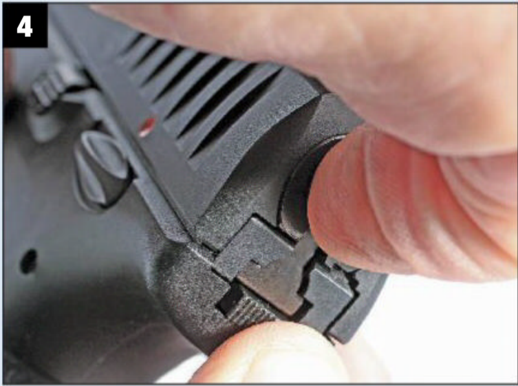
4 And once it moves to the right the striker guide is free to push out of the slide.
