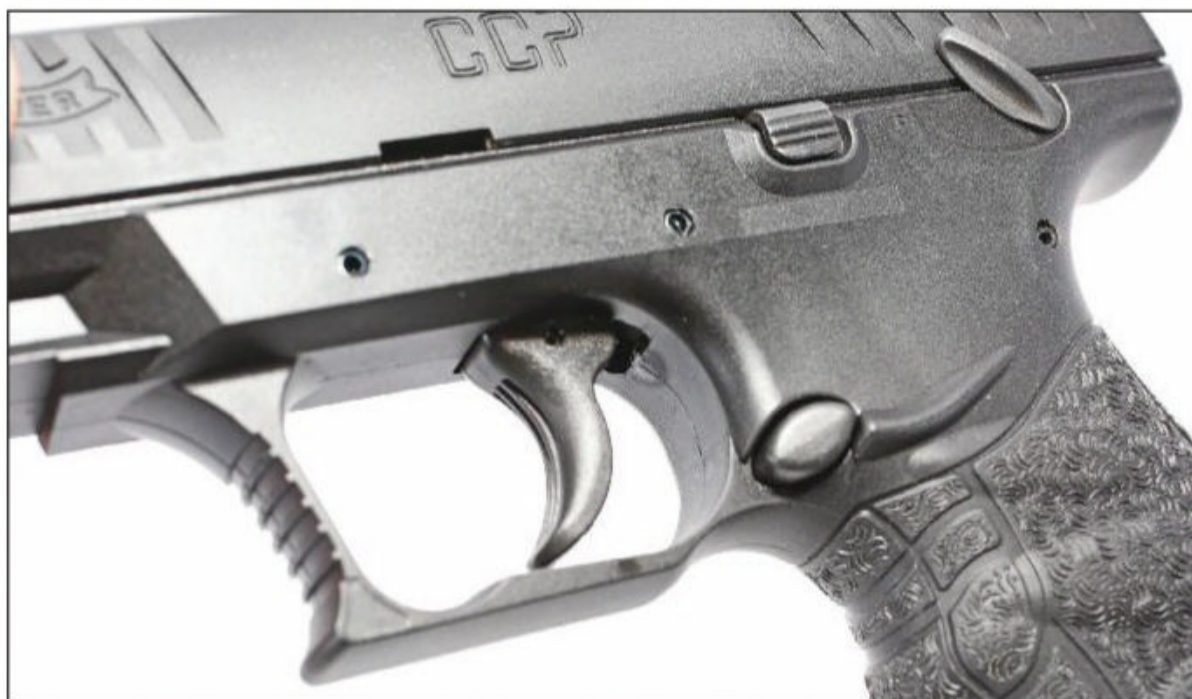
On the side of the polymer shell, you can see the three pins that hold the chassis inside the shell. They are not to be removed. The magazine button, behind the trigger guard, is the American location, and thus this is the M2 pistol. Above and behind those are the slide stop and safety.
