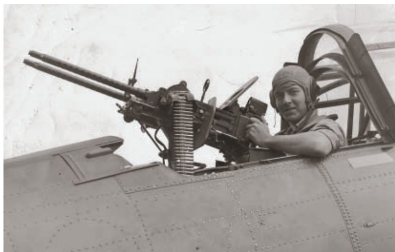
AAM 1/c A. B. Baxter mans the twin Browning AN/M2 machine guns on his SBD-5 in 1944. A lightweight, rapid-fire version of the standard M2 .30-caliber gun, it had a blistering rate of fire of 1350rpm, giving the Dauntless excellent rearward protection. Baxter flew as gunner for VB-16's well-known "wild man," Lt. j.g. Cook Cleland. (Photo courtesy of Jack Cook)
