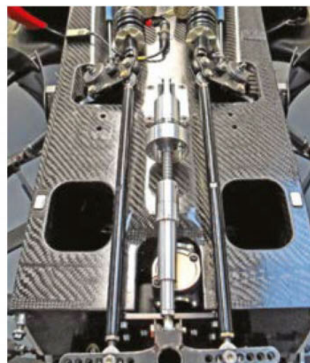
Figure 6: ... which concealed the team's own design inerter at the front...
