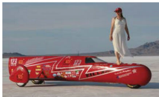
Salt pans are hard, flat and have a friction coefficient of between 0.5-0.6 – the surface works with rubber tyres, albeit special ones
