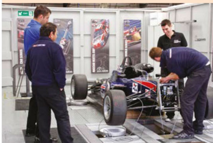
Figure 14: Team West Tec setting up their Dallara F312 for the session on the servo-hydraulic test rig
