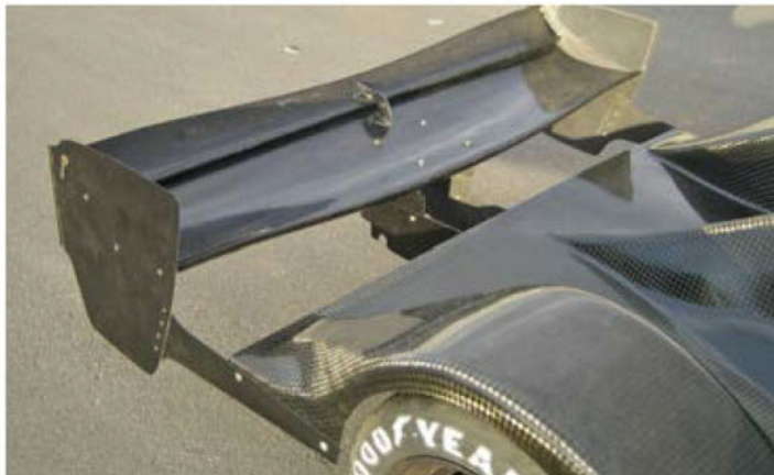
The Dauntless rear wing has been shaped to work with the flows coming off the car (Courtesy: Dauntless Racing)
