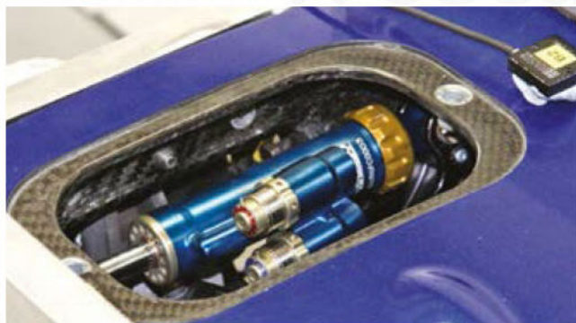
Figure 12: Inerters and four-way adjustables have been banned but teams continue to push suppliers to find performance gains and Team West Tec's Dallaras feature Multimatic third elements front (above) and rear
