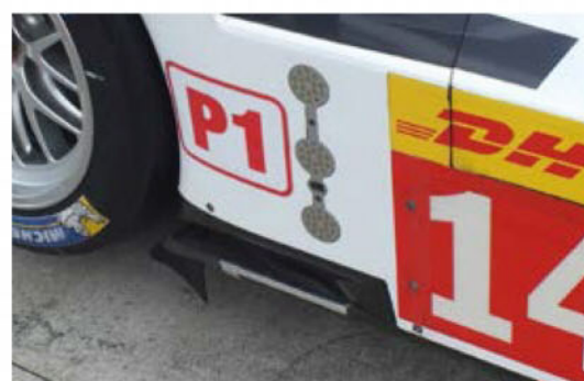
A small turning vane has been added to the leading edge of the floor behind the front wheel
