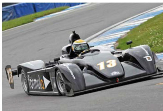
This UK-based Speads runs a Dauntless wing and a splitter devised with Dauntless assistance (Courtesy: BookaTrack.com Ltd)
