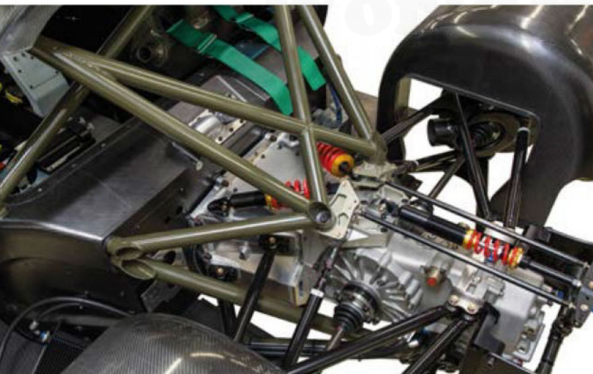
The mother chassis can be configured to be front- or rear-engined. In the front-engined setup here the transmission is off-the-shelf GTA component
