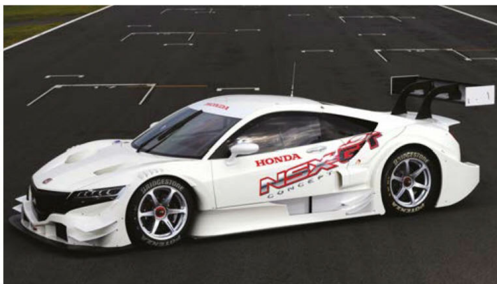
The Honda NSX GT500 features a mid-engined layout but in its original trim (below) it suffered from serious overheating issues, so extra cooling had to be added in the season (above) further increasing drag
