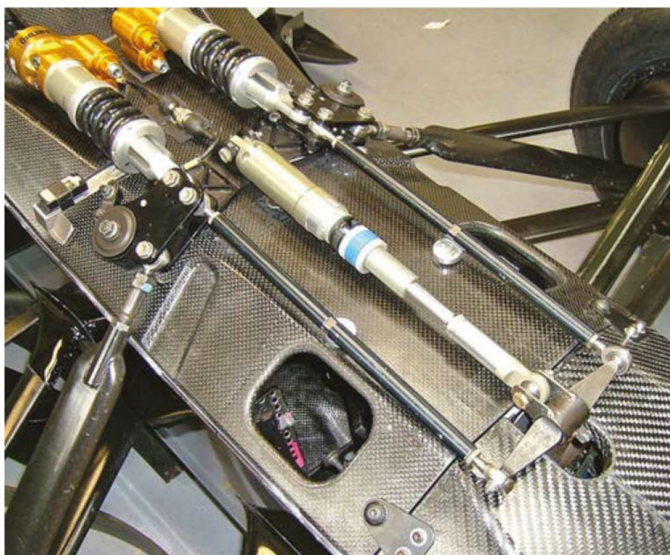
Figure 2: Third element on Fortec Motorsport's 2007 Dallara F307 – 'about as light as you could make it'
