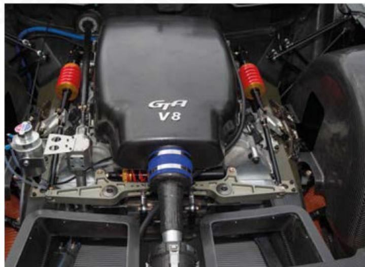
The prototype car which is fitted with the off-the-shelf spec GTA V8 engine – which in reality is a Nissan V8. Other engines can be fitted
