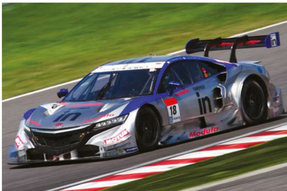
The Honda NSX GT500 features a mid-engined layout but in its original trim (below) it suffered from serious overheating issues, so extra cooling had to be added in the season (above) further increasing drag
