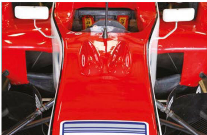
Figures 4 and 5: 'Two humps or three, sir?' One of Fortec Motorsport's Dallara F308s had grown a third damper blister in 2008...
