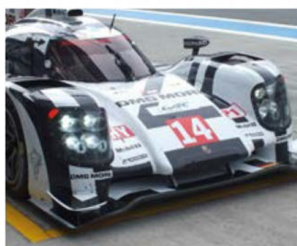
A new front splitter was used in Japan, with a subtle change in shape to that used at Le Mans
