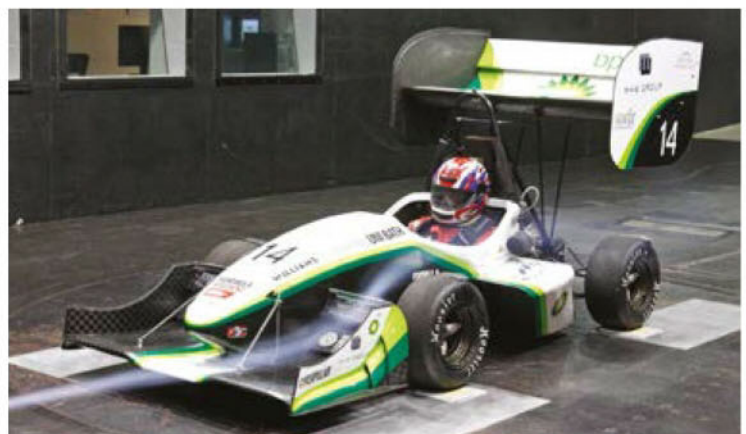
Figure 2: TBR 14's aerodynamics were dominated by its large, aggressive wings; the front wing incorporated some intricate detailing
