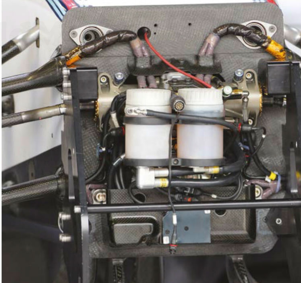
Front bulkhead showing torsion bars and master cylinders
