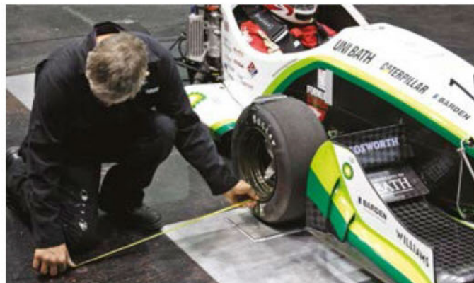
Figure 6: Re-checking the car's alignment after installing tyre shim plates
