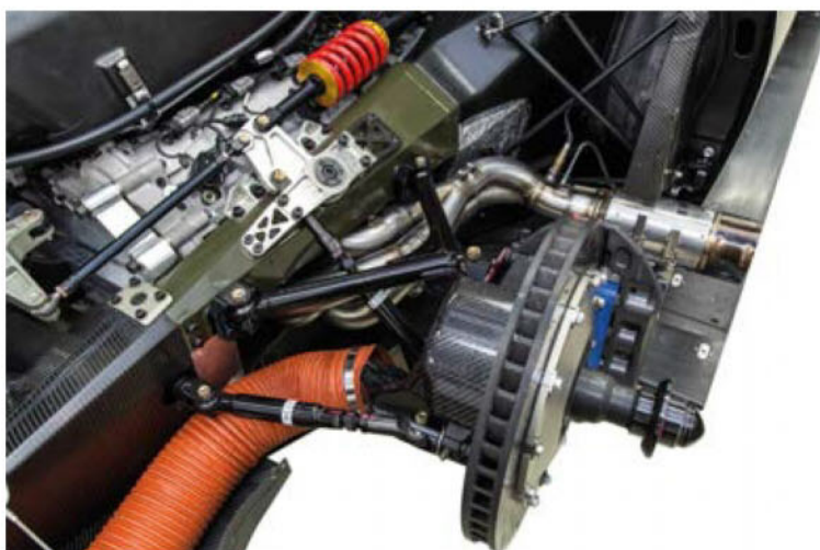
At the front of the mother chassis prototype, a steel structure mounts to the front of the monocoque which carries the engine and suspension
