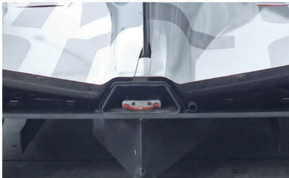
Porsche ran with a revised tail in Japan. The trailing edge of the bodywork still has scop to flex at high speed
