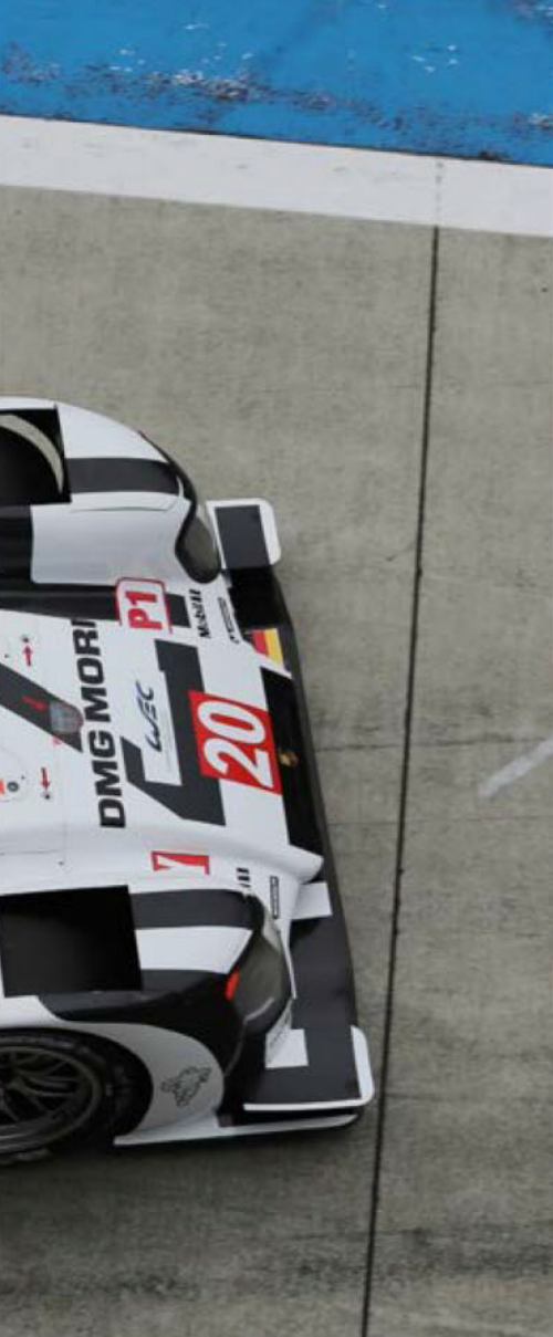
Porsche ran with a revised tail in Japan. The trailing edge of the bodywork still has scop to flex at high speed
