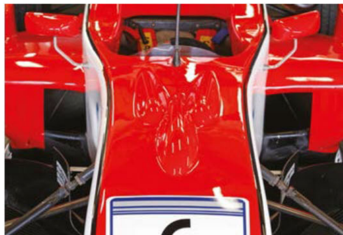
Figures 4 and 5: 'Two humps or three, sir?' One of Fortec Motorsport's Dallara F308s had grown a third damper blister in 2008...
