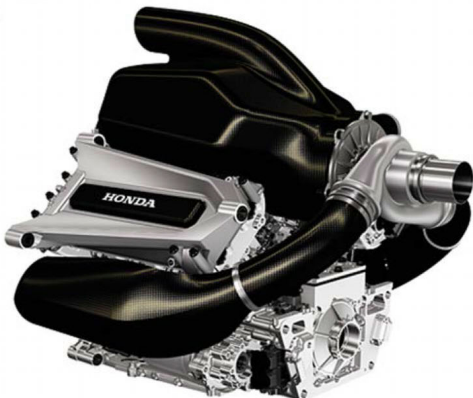
Honda's new power unit. Like all of the current F1 generation it is a turbocharged 1.6-litre V6 engine with direct injection, with a pair of motor generator units and an electrical energy store
