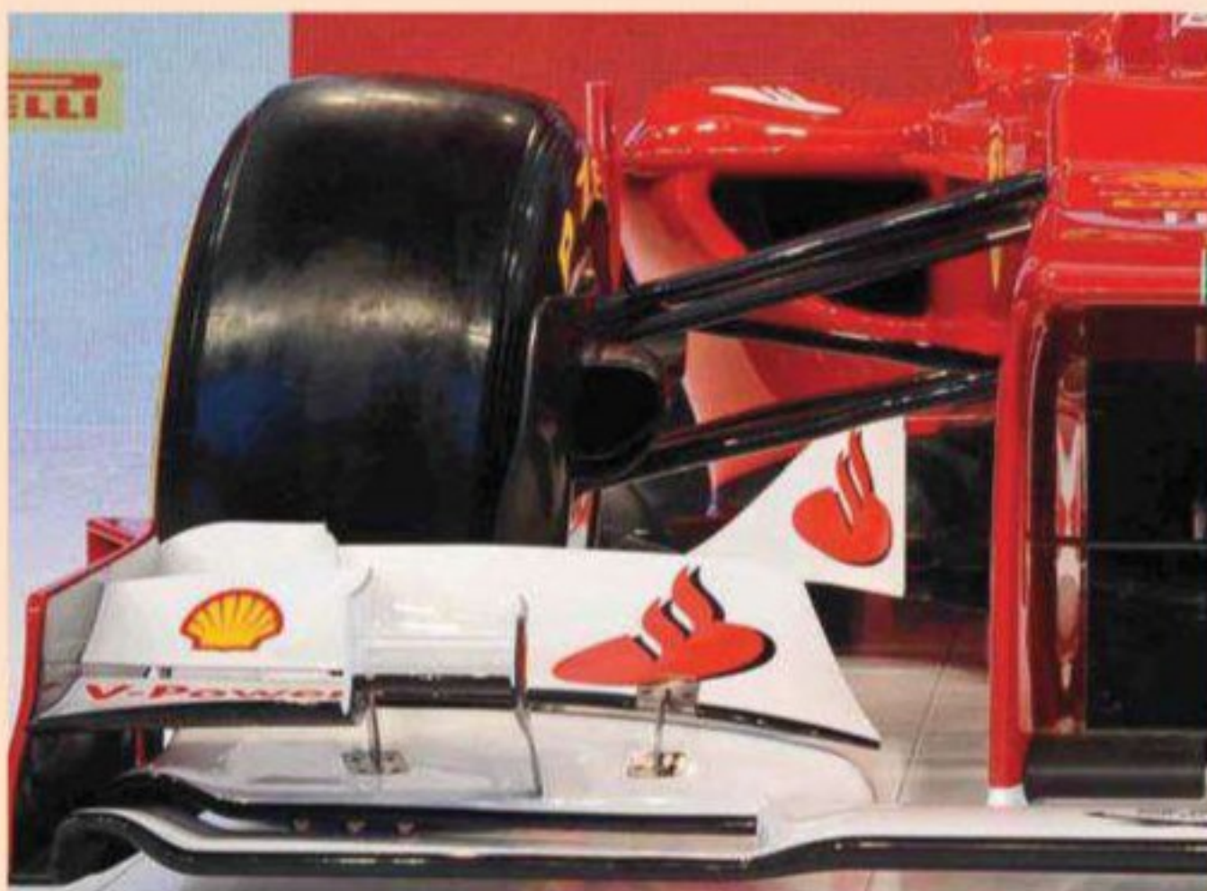
Ferrari has taken a very different approach to its front suspension on the F2012, uniquely for the 2012 season going for a pull-rod layout
