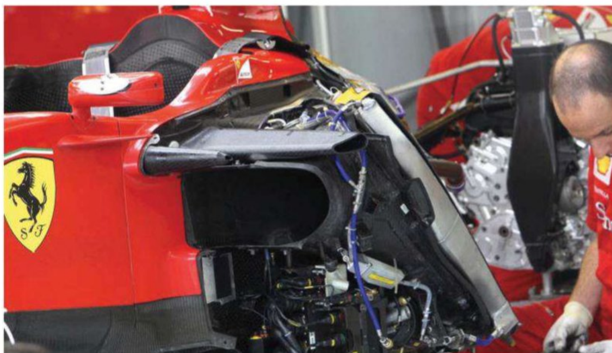
The location of the sidepod inlet duct is essentially fixed, with aerodynamic demands and the mandatory side impact structures defining its shape to some extent and its size. KERS components can also create issues
