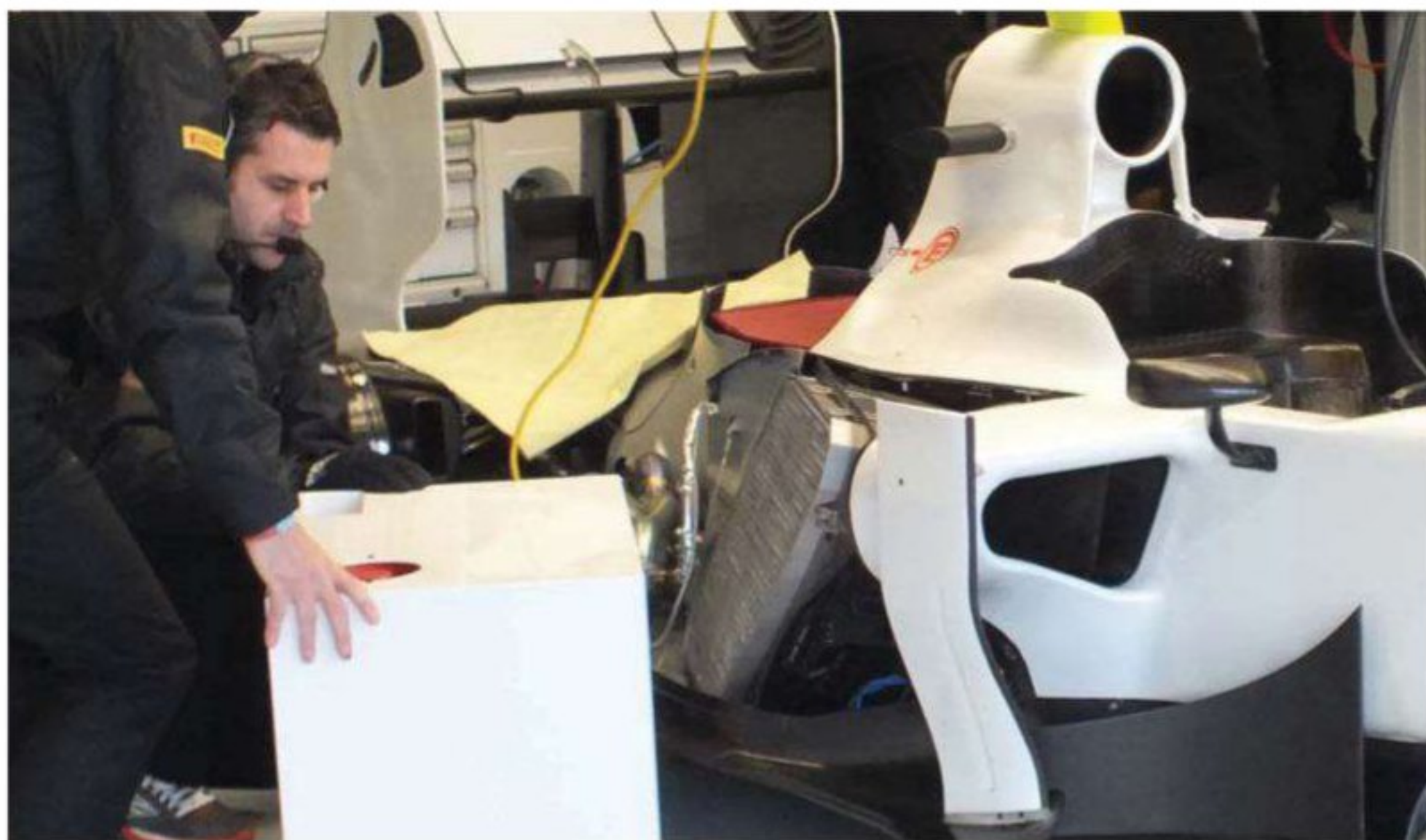
The 2011 HRT F111 has a fairly conventional cooling layout, with the heatexchangers sat in the sidepod at a slight angle. Positioning and shape of the radiators has a major influence on the cars aerodynamics
