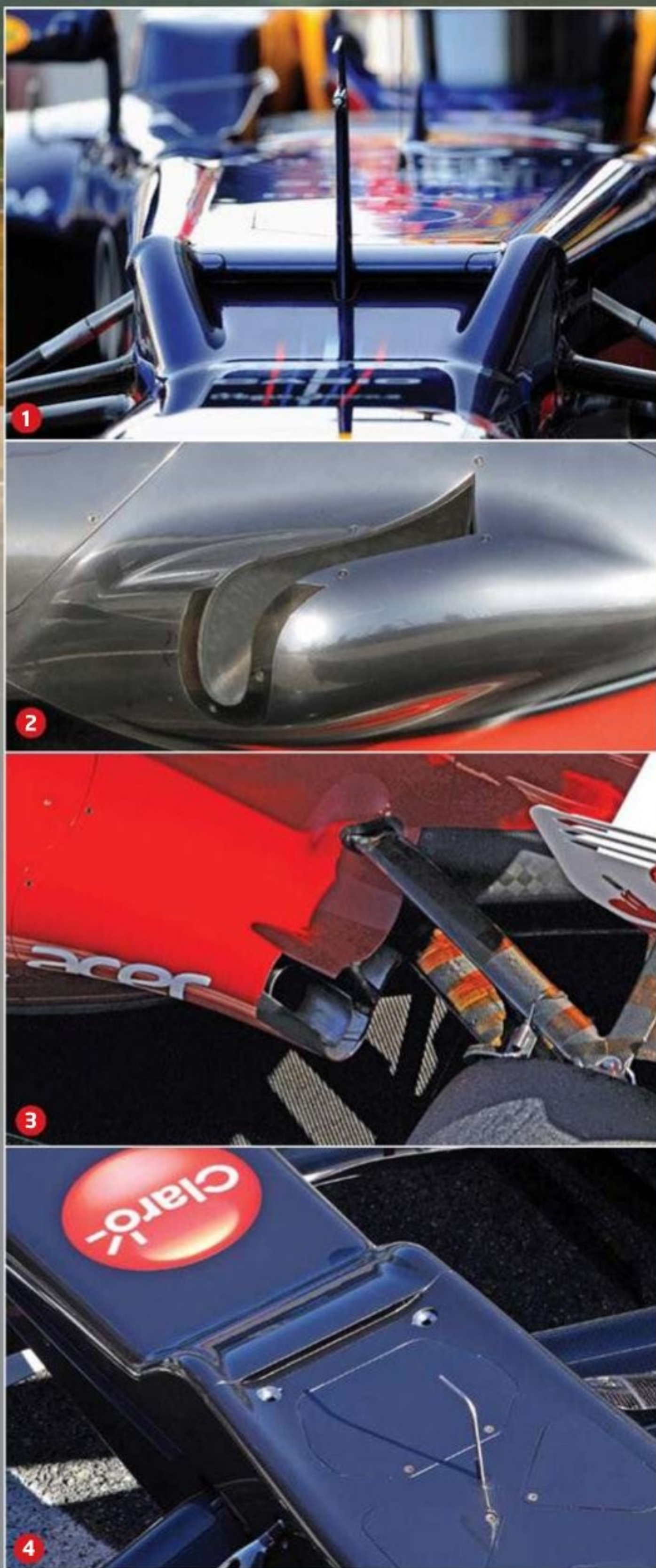
1. Red Bull's 'driver cooling duct' has attracted much discussion 2. McLaren's exhaust exits sit a long way outboard of the chassis and on the limit of the regulatory box. Some have already questioned the legality of the design 3. Ferrari has experimented with many variations of its exhaust in an attempt to re-capture some of the lost downforce 4. Sauber's nose duct faces the opposite direction to the one on the Red Bull
