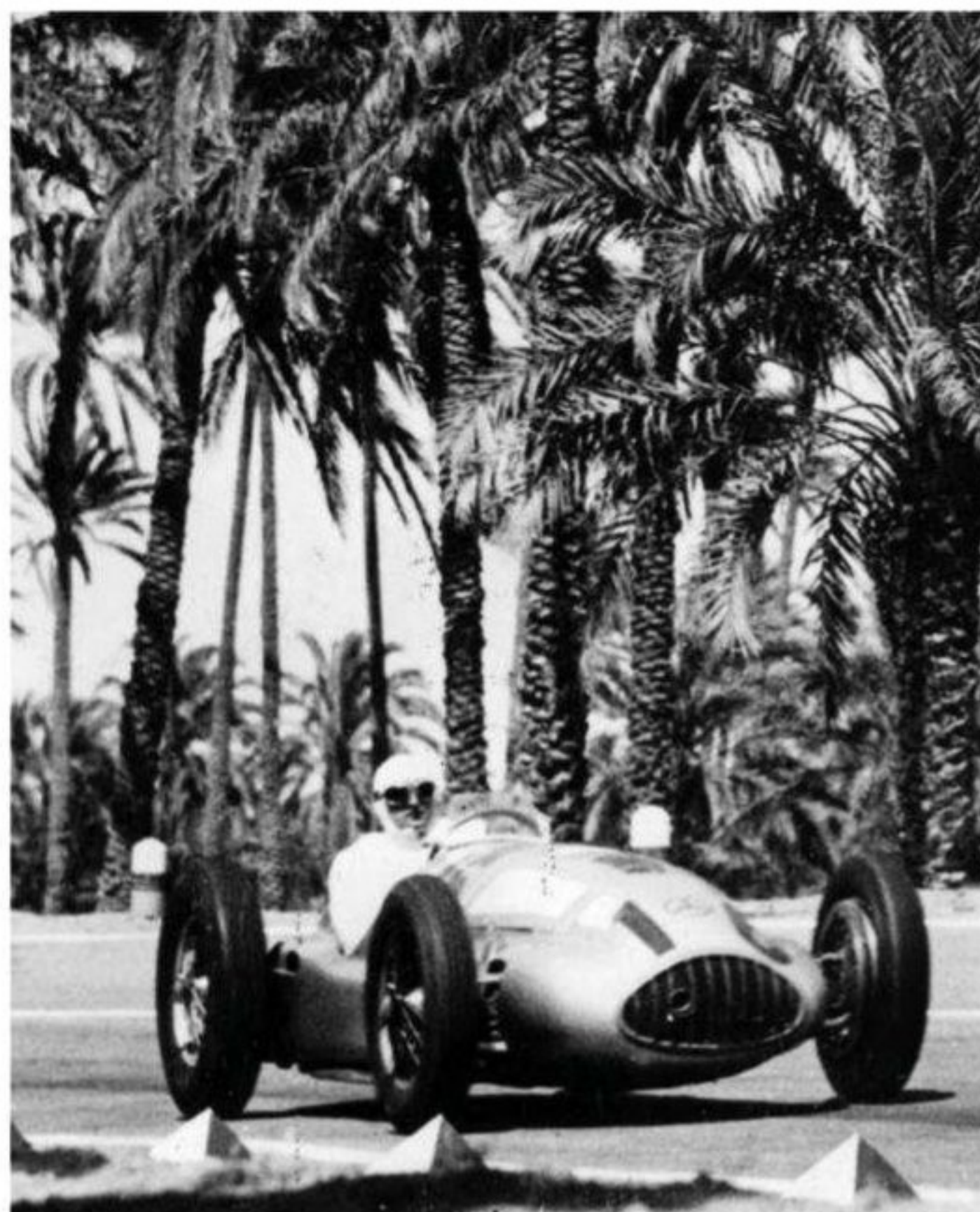
Like its predecessors, the W165's suspension design promoted understeer, which, with the skinny tyres, required a very committed driving style
