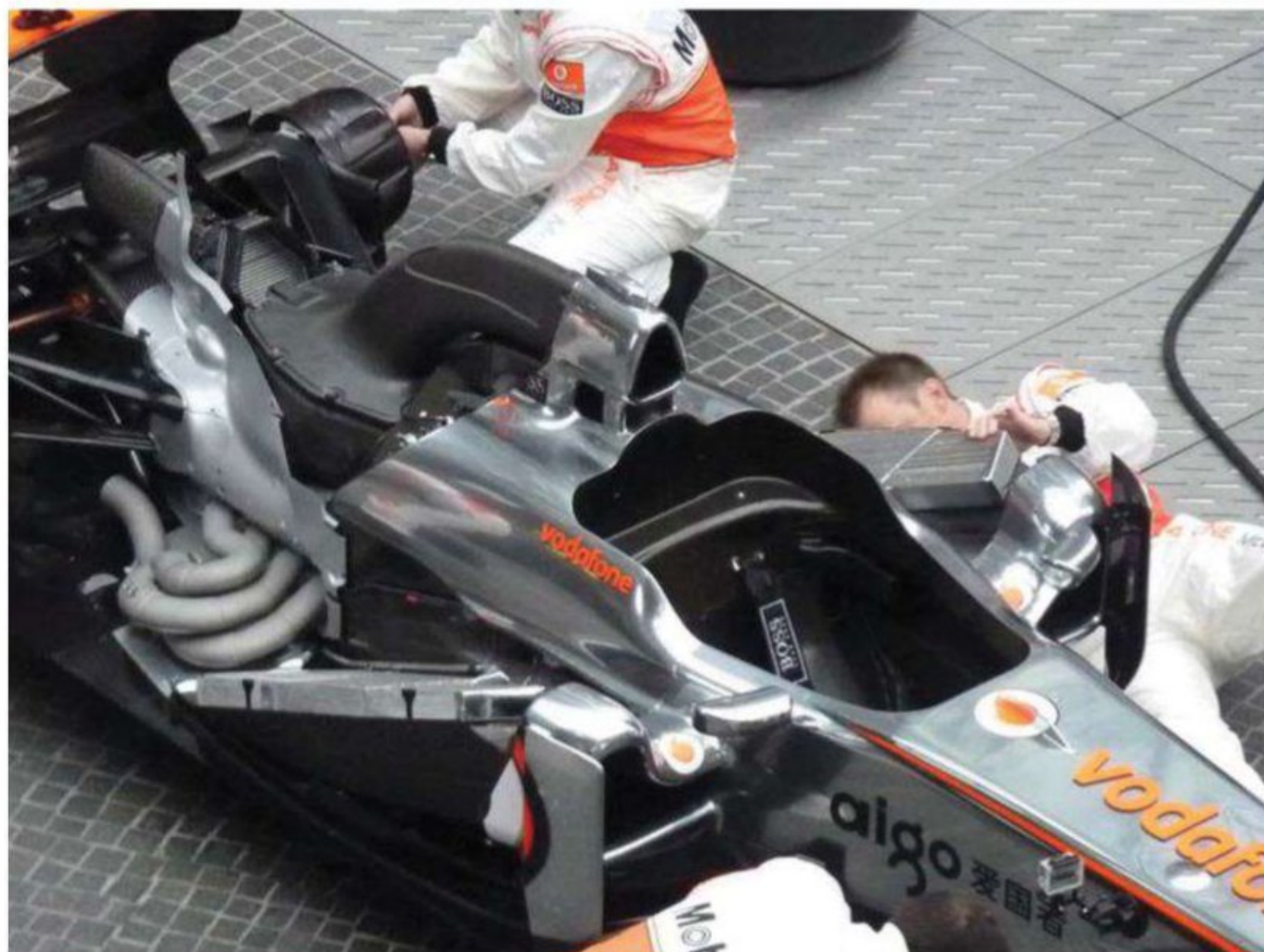
McLaren's 2011 car was launched without its bodywork allowing a view of a slightly more unconventional sidepod layout, the radiators sit at a very different angle to that of the HRT. Note the gearbox heat exchanger at the rear
