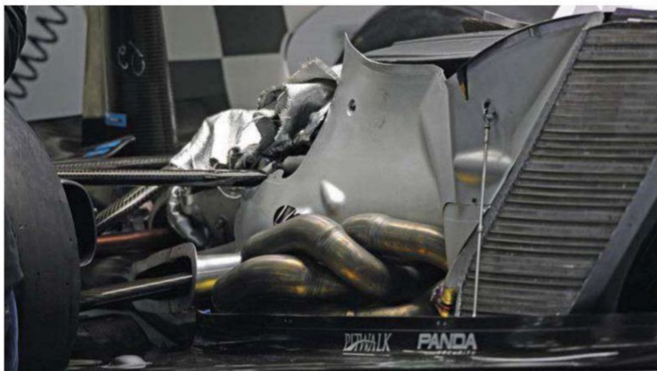
The shape of an F1 radiator core can be angle and twisted to achieve the optimum surface area in the limited space available, here the heat shielding around the rear of the car is clear to see
