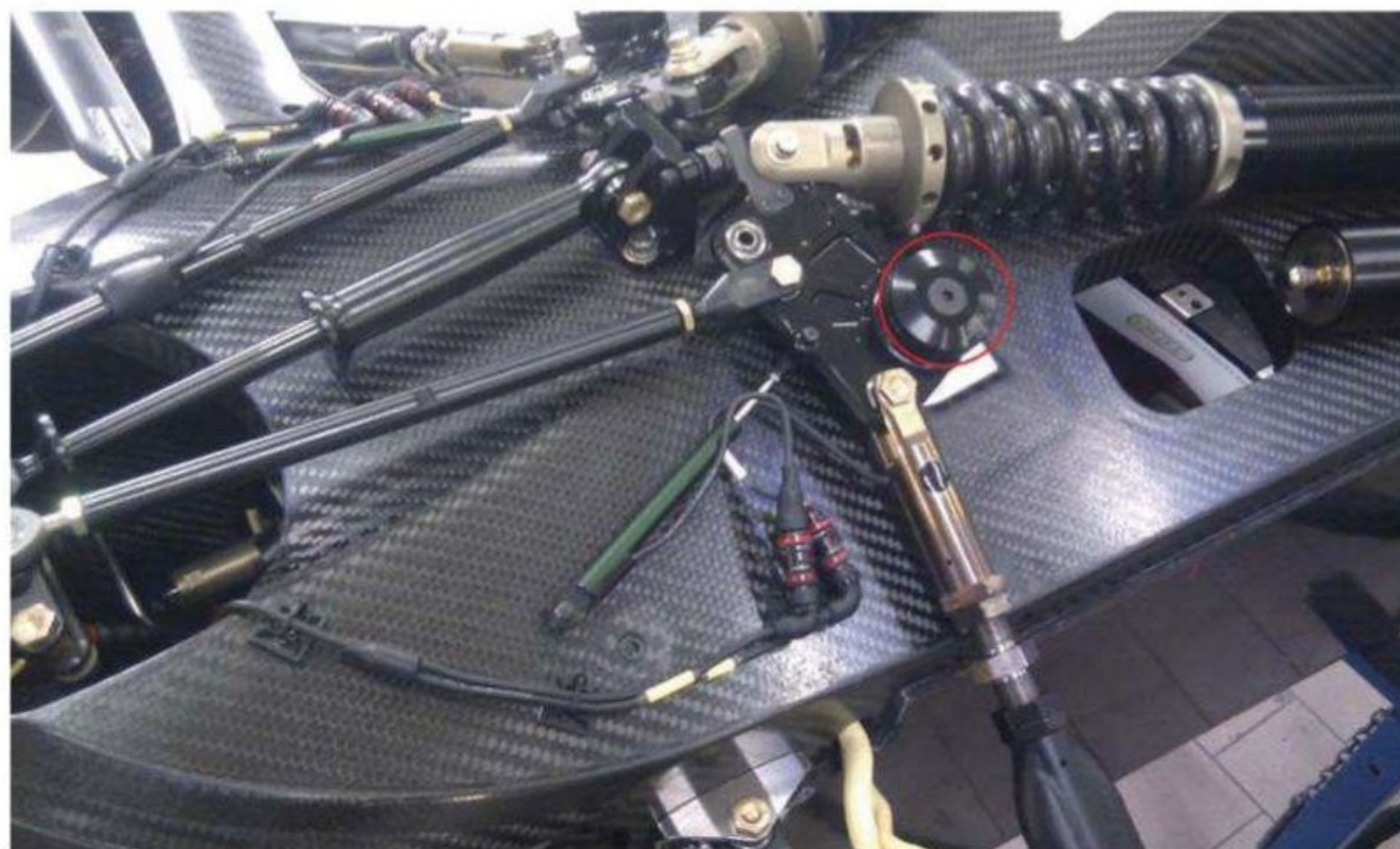
Figure 1: either a linear or rotary potentiometer can be used for rocker arm-type suspension. The linear sensors fitted in the picture below are green, while a rotary sensor would be fitted where the rocker arm is fixed to the chassis (marked by the red circle)
