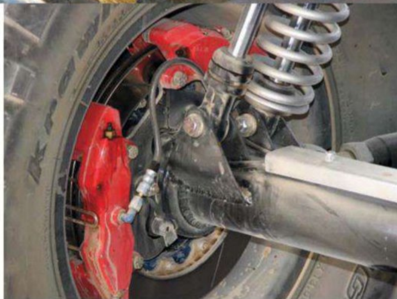
Dual brake calipers used on the rear axle – one for the main system and another for the cutting brakes, with protective covers for the brake lines
