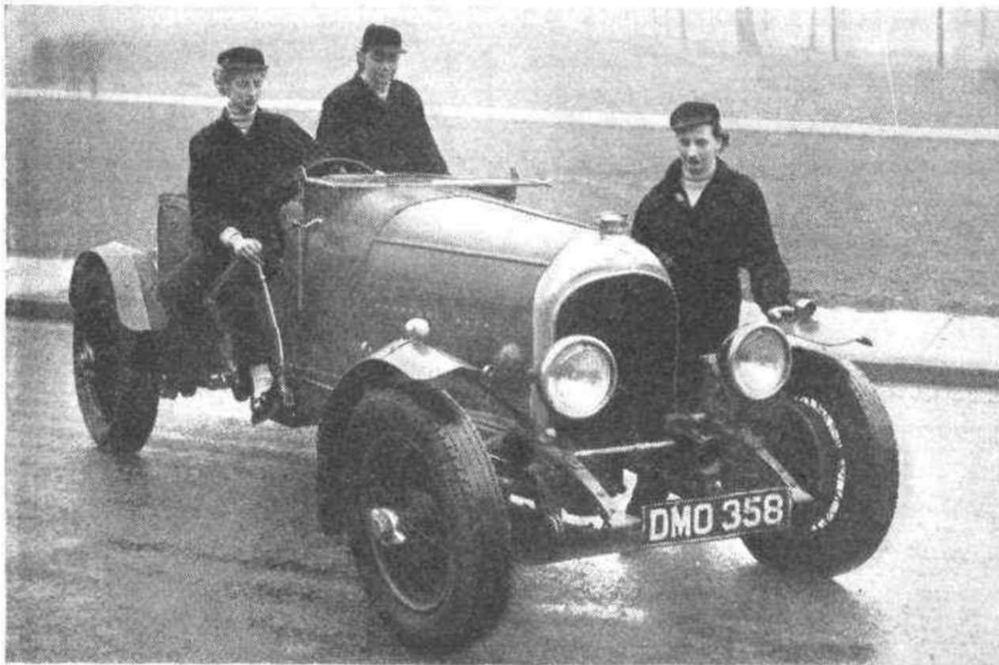
BENTLEY 3-litre Red Label. This car was completely rebuilt in 1947 with a new 2/4-seater body. It has many mods., including six half-brake drums, twin Zenith carburettors, electric pumps, etc. Excellent hood, etc. (our glamour gallon girls EXTRA) ... £250
