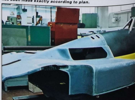
18. The bonnet can be any of a number of different shapes; here, a very long one has been fitted towards the back of the body. Other, shorter ones, will also be tried.
