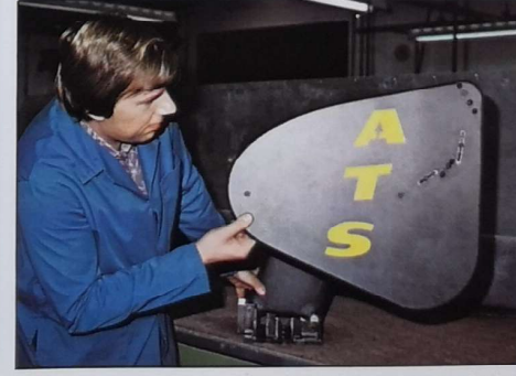
8. The first carbon fibre part to be fitted is the rear wing. Carbon fibre is expensive, but can reduce the car's weight substantially. Even the side wing panels are made using this technique; several panels are made.
