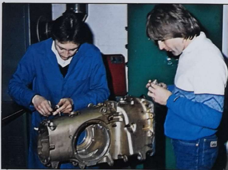
13. According to Gustav Brunner, the shape of the gearbox is important; the aerodynamic efficiency of the rear part of the car depends to a great extent on how narrow the gearbox casing is. Manfred Winkelhock looks on.
