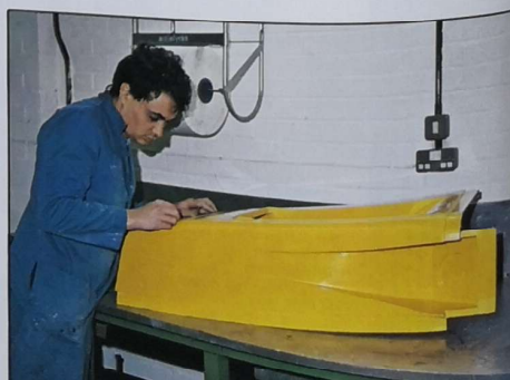
6. After the shape of the sidepods has been decided, they are made up out of fibreglass, ready to be fitted on to the car. The shape of the sidepods is not necessarily final. It may be modified in the course of the season.
