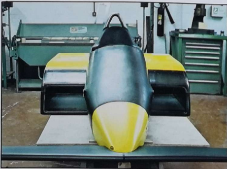
17. Gradually, bits are added to the body; once the oil and water radiators have been installed, the fibreglass sidepods are fitted into place. At this stage, no-one can tell whether they will feed enough cool air to the radiators.
