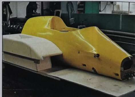
5. Once aerodynamic tests have been carried out on the bodywork, the side pods, with the oil and water radiators, are fitted to the model. They are made of wood, which means their shape can be easily altered.
