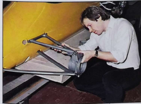
7. The parts that make up the suspension are ready to be fitted to the buck. Here, some of them are placed on the model to allow the design team to see where the mounting points on the final body should be.
