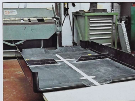
15. Unlike last season's cars, this season's have a flat bottom, which cancels out most of the ground effect. In the case of the ATS, this too is made out of carbon fibre.
