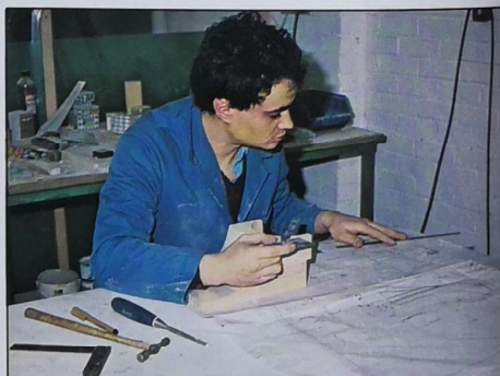
2. Once the basic design is ready, the next step is to bring that design to life; wooden moulds are made. Fibreglass ones will follow.
