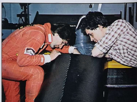
14. The carbon fibre body, built by Seger and Hoffmann, has just arrived; Manfred Winkelhock wastes no time in deciding where the safety harness should be fitted, and checks that the driver's seat has been made exactly according to plan.
