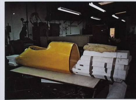
4. An example of how the fibreglass model is used; it allows the team to see very quickly where the fuel tank should be fitted. (The fuel tank itself is a model, also made of fibreglass.)
