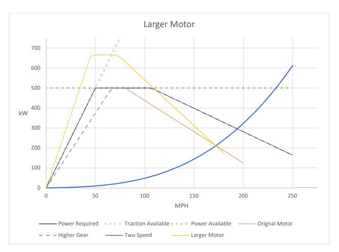
What if we took the space and weight of the two-speed transmission and put that into a bigger motor. Let's just scale up the motor we've got by 10%. That means 10% longer, 10% larger diameter, and 33% more weight.
