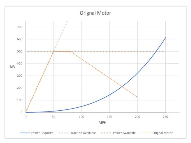
Now we have to choose a motor for our car. Conveniently, motors have constant torque at lower RPM's that, with the correct gearing, will line up with the traction available extremely well. This is mostly why BEV's are so unbeatable off the line. If the BEV has as much traction as another vehicle, there's no amount of power that can be applied to accelerate faster.
