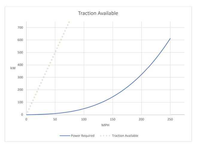
Next, we'll plot out the traction available to the car. Any more power applied to the tires than this diagonal line will only cause the tires to spin and won't accelerate the car more quickly. A heavier car or tires with better grip will make this line more vertical, but that won't change our results. The same can be said for non-linear changes in traction caused by things like downforce.
