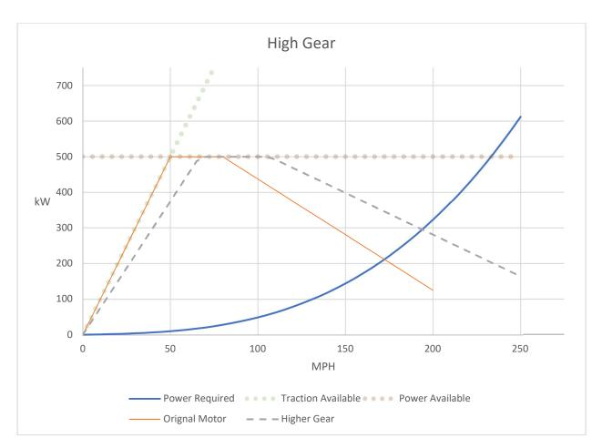
Nobody says that the car has to be geared right to the edge of traction though. What happens if we increase the gear ratio by a third?
