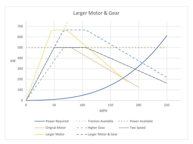
With the bigger motor, a higher gear can be driven. When we increase the gear ratio of the larger motor to line up with the traction available, an amazing thing happens. The battery still caps the power output of the motor to 500kW, but the motor can provide that output all the way up to 160MPH. The higher gear ratio allows a slower decay of power output and the end result is a top speed of 210MPH.
