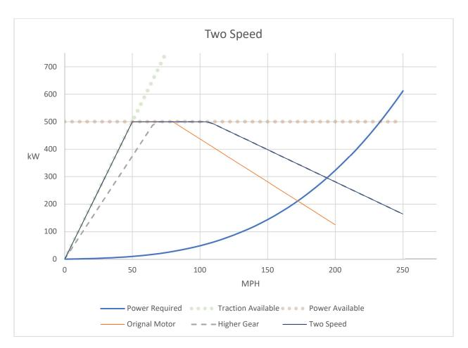
The obvious solution is to put in a two-speed gearbox. As long as the transmission shifts between 70 and 80 MPH, you get the full benefit of both gears. The only downside is the relatively small weight and added complexity of the two-speed transmission. It's looking like a slam-dunk for two speed transmissions and many engineers would stop the analysis here, but were going to go a little further, just to be sure.
