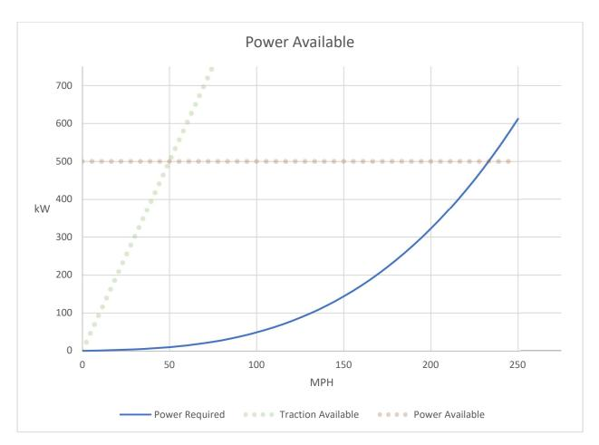
We'll also need to define the amount of power the battery can safely deliver. I choose 500kW for the nice round number. This isn't as high as a Porsche Taycan or a Performance Tesla Model S or X, but It's probably higher than most other BEV's. This value will change with temperature and state of charge but it will stay a horizontal line which is all the matters to this example.
