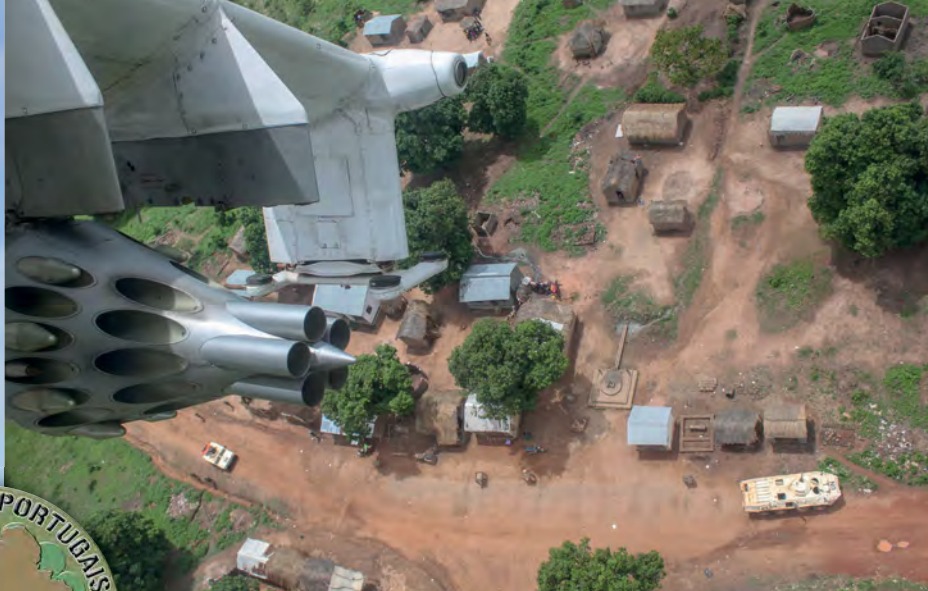
Above: A view from the cabin of one of a pair of Mi-24 helicopter gunships provided by Senegal for jungle operations in the CAR. Note the partially loaded UB-57-32 pod for 57mm rockets under the stub wing. Left: The insignia of Portugal's Airborne Rapid Reaction Force in the CAR. Below: The heavy machine gun position on a Portuguese armoured vehicle as a Senegalese Mi-24 in UN markings prepares to depart a basic airstrip. Temporary bases deep in the interior of the Central African Republic, with fuel supplies, have proven essential in the ongoing war. All photos Al J Venter Collection
