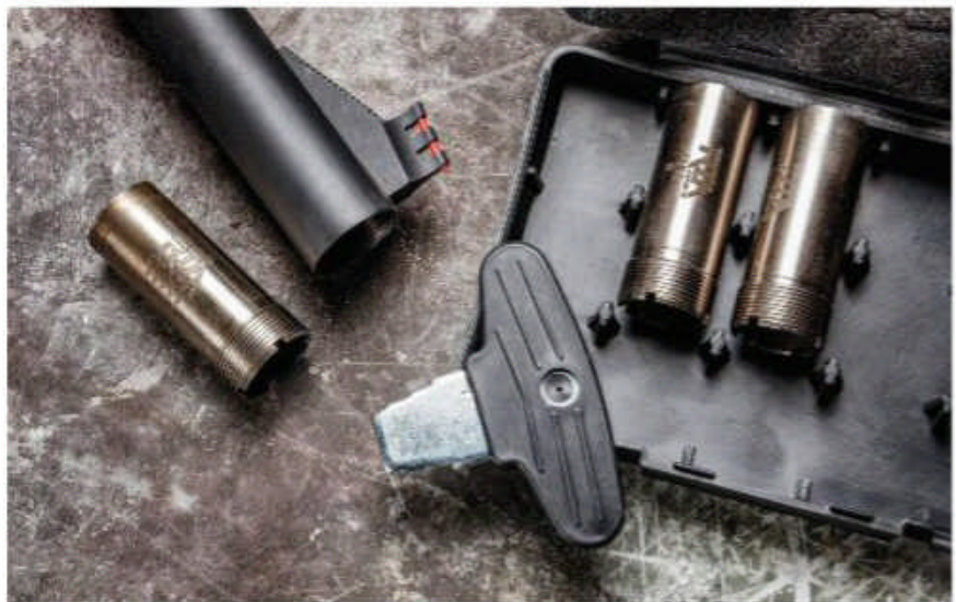
Three choke tubes were included with the VRPA40: Cylinder, Modified and Full. Notches — five, three and one, respectively — on the top lip of the tubes identify the different constrictions.
