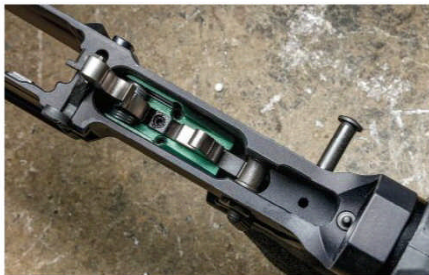
Disassembly follows the familiar two-pin procedure of most AR-style platforms. From the factory, the UP-15 comes with Velocity Precision Engineering's Curved Classic AR Trigger.
