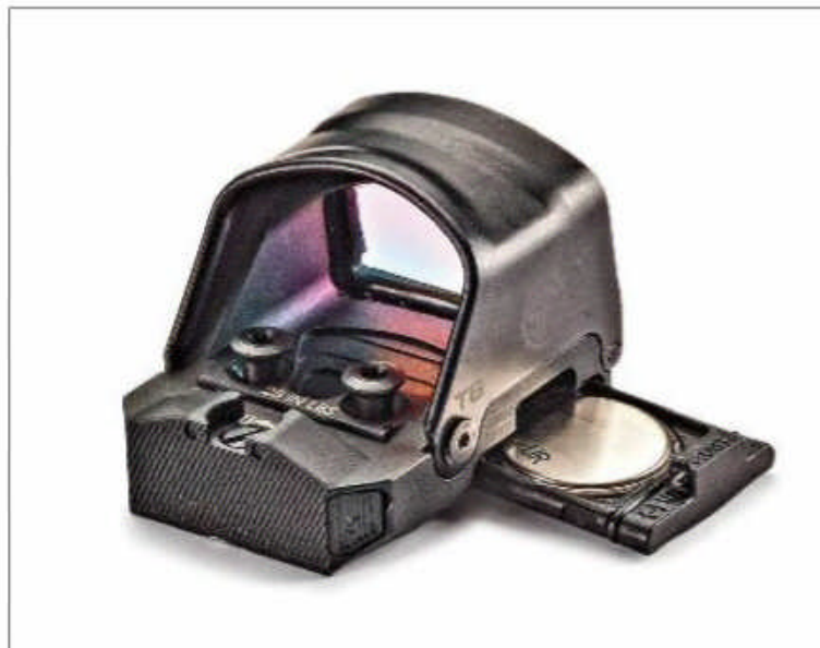
The Romeo2 features a spring-loaded, O-ring sealed battery tray that is release by a button at the right-rear of the sight. The sight is powered by a CR2032 battery.
