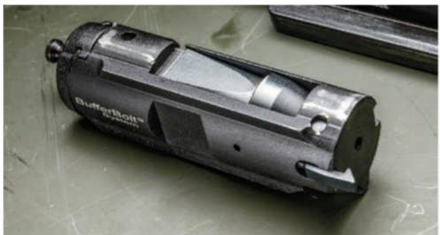
The gun's bolt uses a single extractor that proved capable and reliable even under the stress of fast-paced courses of fire and a long day at the range firing a mixed bag of 12-gauge ammunition.
