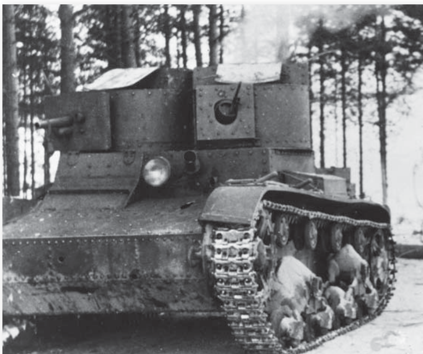
A twin-turret T-26 Model 1931 knocked out during the 1939–40 Winter War with Finland. It has the original riveted hull and has a 37mm PS-1 gun in the right turret.
